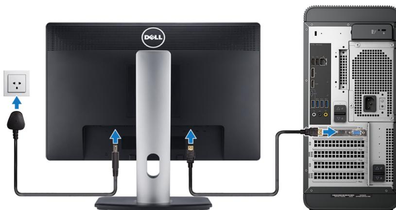
**NOTE:** If you ordered your computer with a discrete graphics card, the HDMI and the display ports on the back panel of your computer are covered. Connect the display to the discrete graphics card.
