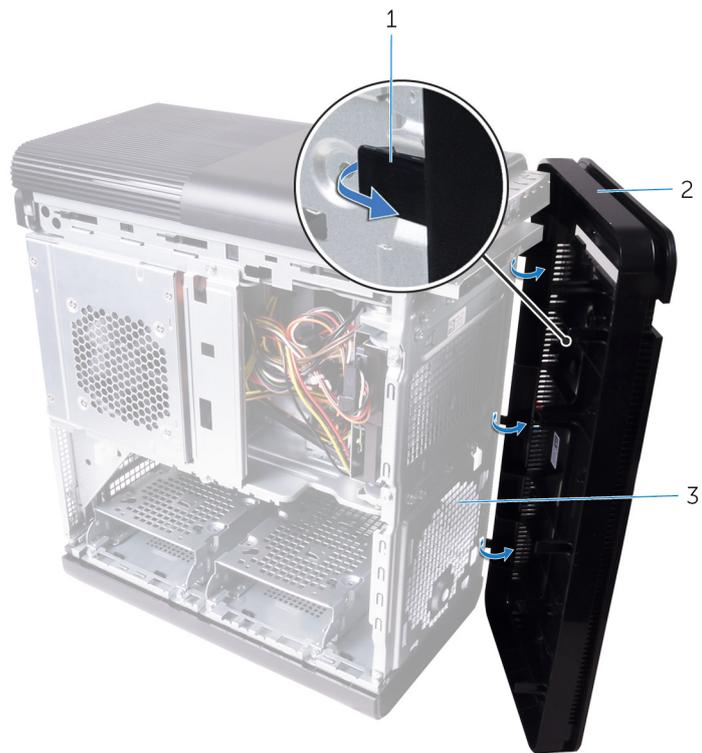
**Figura4. Remover a moldura frontal**
