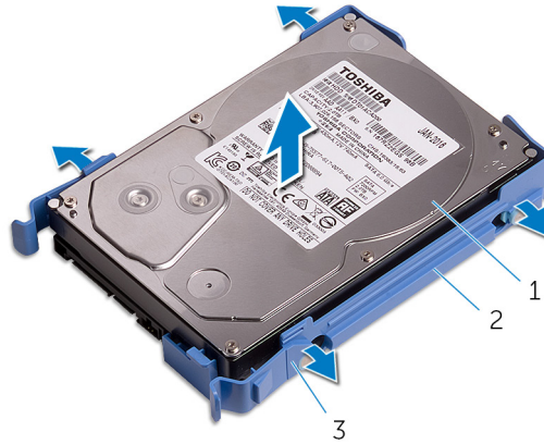
Figure 13. Removing the hard drive from the bracket
