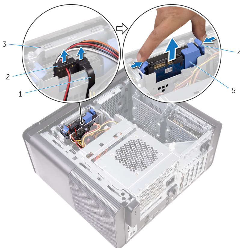
Figure 12. Removing the hard-drive assembly
