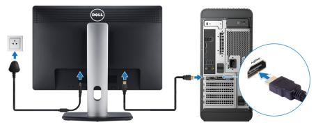
i NOTE: If you ordered your computer with a discrete graphics card, the HDMI and the display ports on the back panel of your computer are covered. Connect the display to the discrete graphics card.
