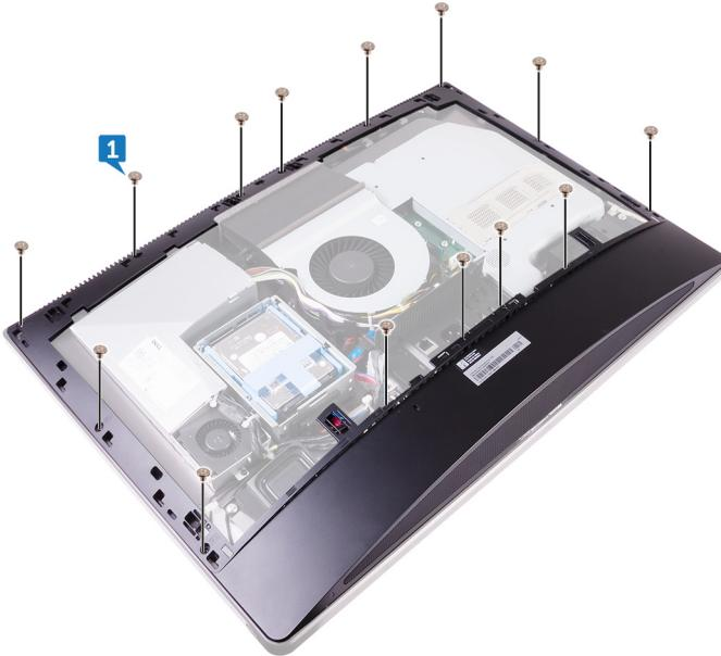
2 Gently pry the inner frame from the sides and lift it off the middle frame.
