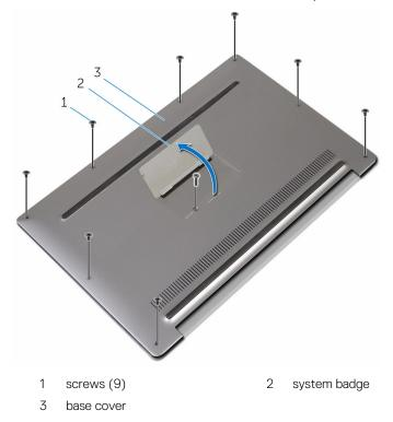
Starting from the back of the computer, pry up the base cover using a plastic scribe.
