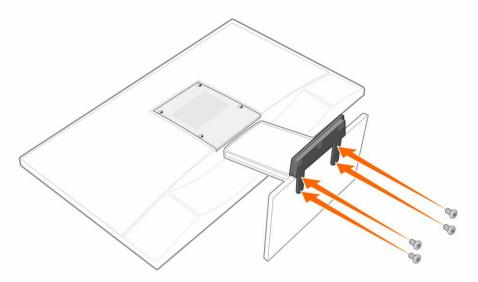
3 Attaching the E mount to the monitor–Remove the four screws from the back of the monitor. Position the E mount on the back of the monitor, and attach it using the same screws.
