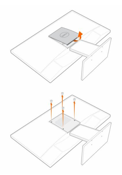
3 Attaching the base extender—Slide the base extender onto the monitor stand and use the screws provided in the tool kit to secure the base extender to the monitor stand.
