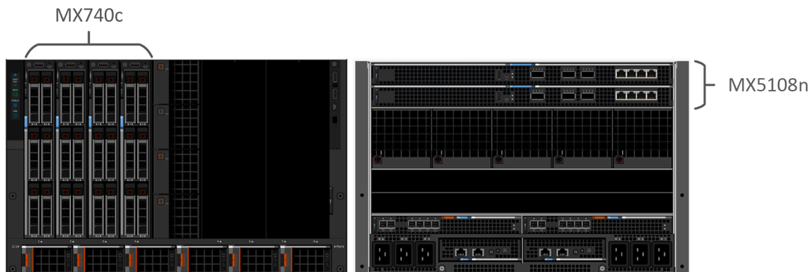
Figure 13. Single PowerEdge MX7000 enclosure
