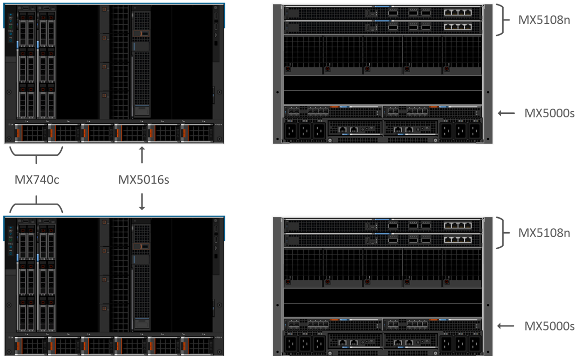
Figure 16. Two PowerEdge MX7000 with MX5016s storage
