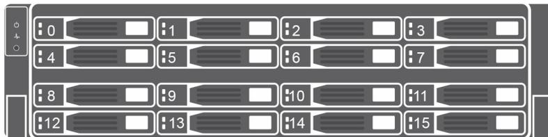
Figure 8. SCv3000 Storage System Drive Numbering
