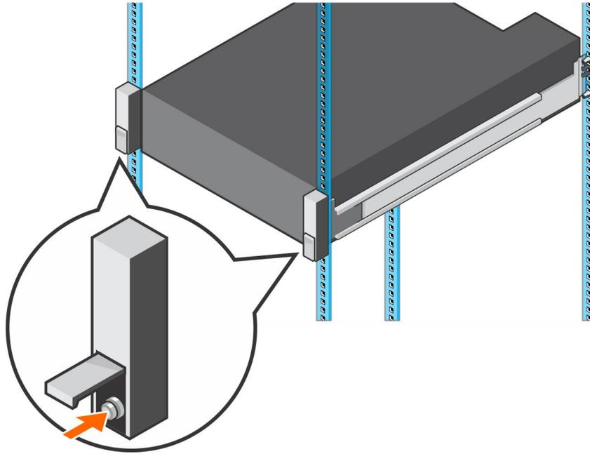
**Figure 11. Tighten the Screws**
