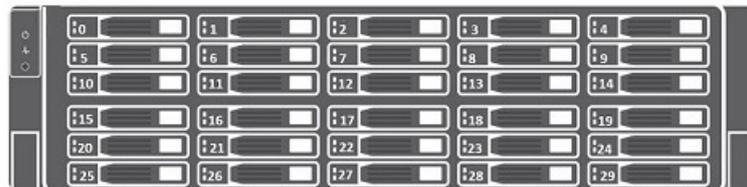
Figure 9. SCv3020 Storage System Drive Numbering
