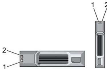
**Figure 3. SCv300 and SCv320 Expansion Enclosure Drive Indicators**
