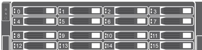
**Figure 4. SCv3000 Storage System Drive Numbering**
