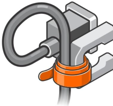
**Figure 12. Removing the Hook and Loop Strap from the Power Cable**
