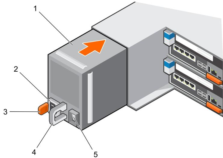
**Figure 13. Removing a Power Supply/Cooling Fan Module**
