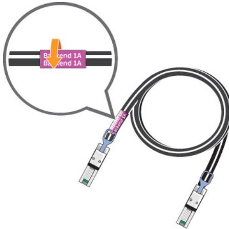
**Figure 50. Wrap Label Around Cable**
