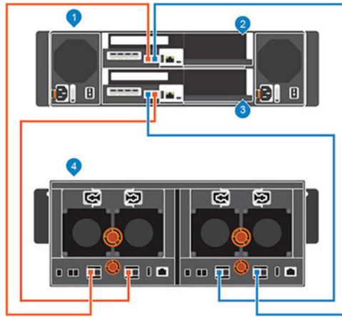
**Figure 47. SCv3000 and SCv3020 and One SCv360 Expansion Enclosure**
