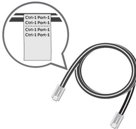
**Figure 37. Attach Label to Cable**
