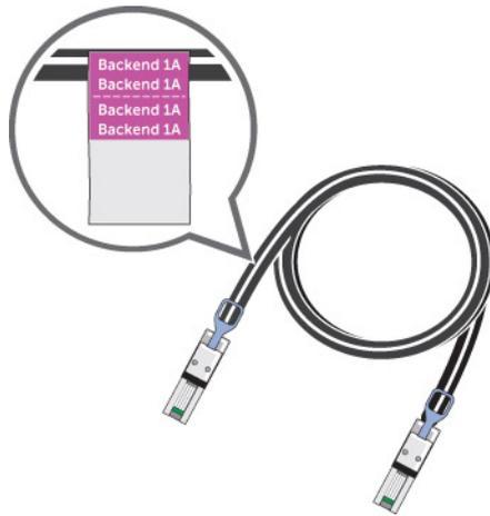
**Figure 49. Attach Label to Cable**
