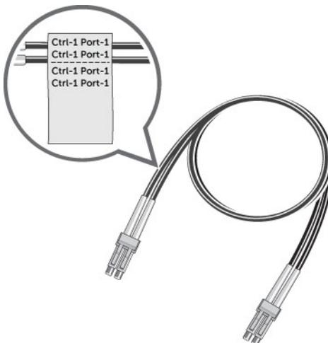
**Figure 32. Attach Label to Cable**
