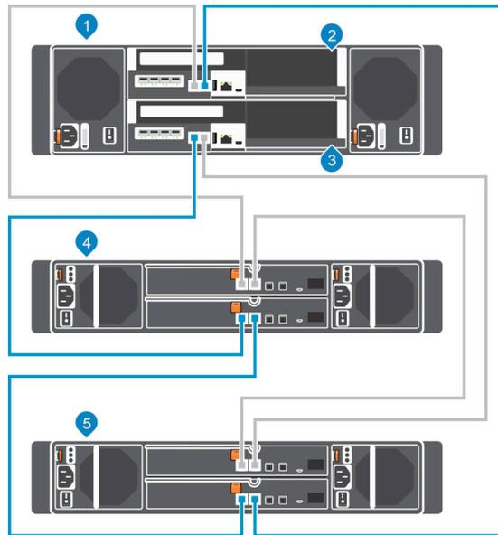
**Figure 55. Connect the B-Side Cables to the Expansion Enclosures**
