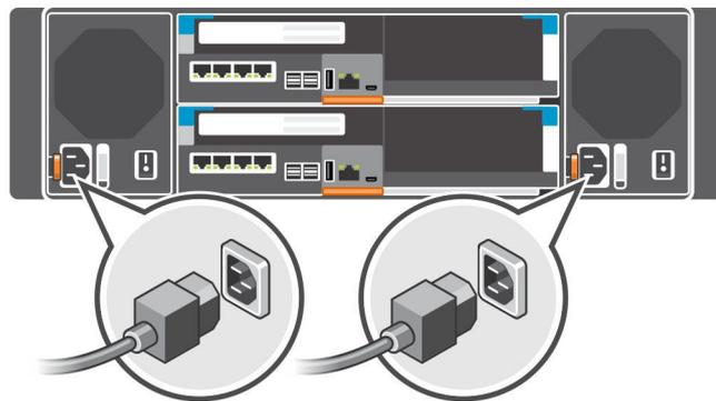
**Figure 51. Connect the Power Cables**
