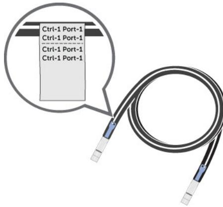
**Figure 40. Attach Label to Cable**
