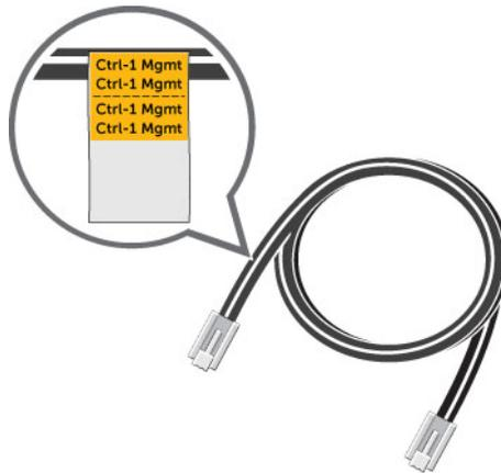
**Figure 43. Attach Label to Cable**
