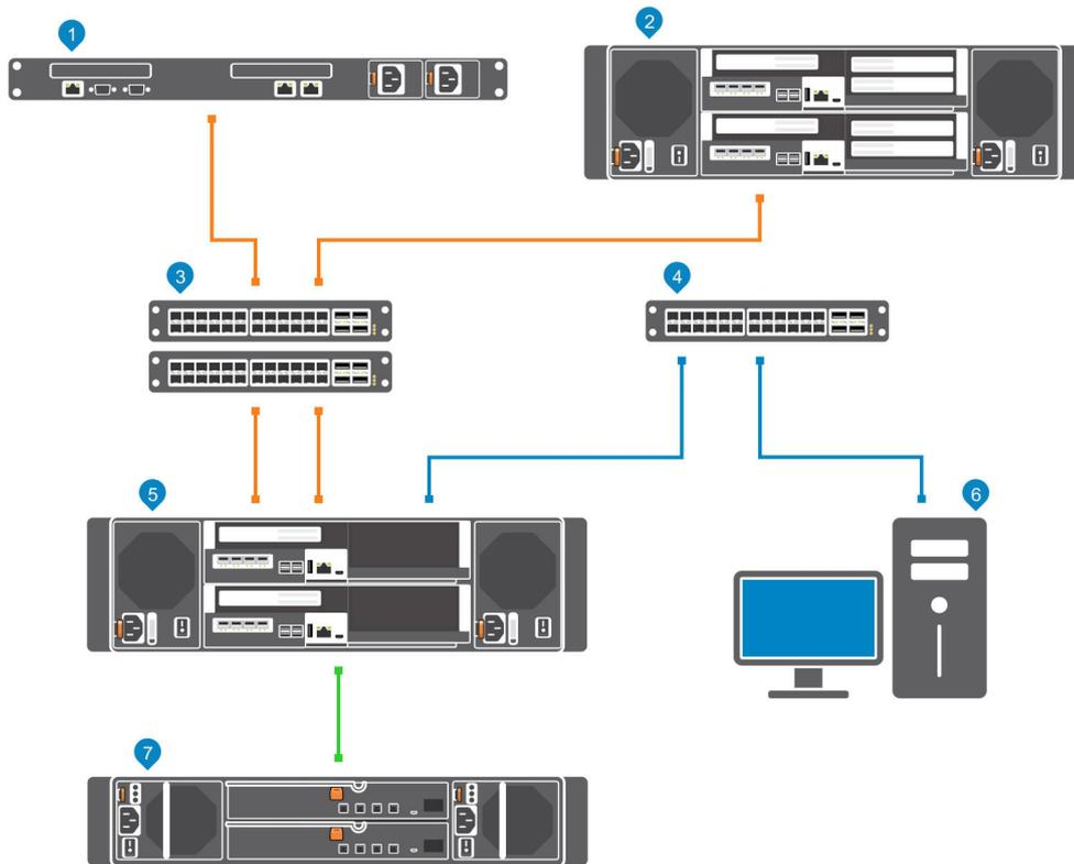
**Figure 2. Storage System With iSCSI Front-End Connectivity**
