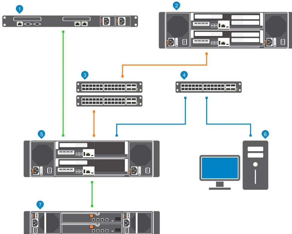
**Figure 3. Storage System With Front-End SAS Connectivity**
