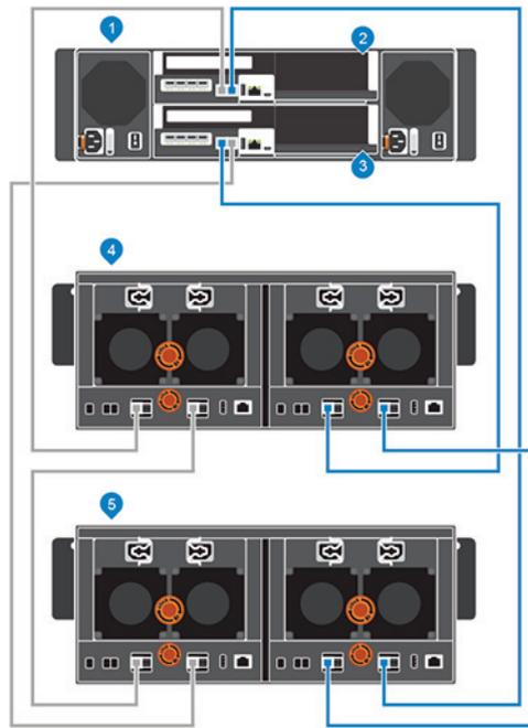
**Figure 67. Connect B-Side Cables to the New Expansion Enclosure**
