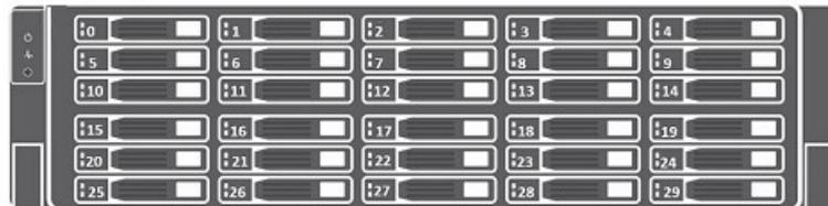
Figure 10. SCv3020 Storage System Drive Numbering
