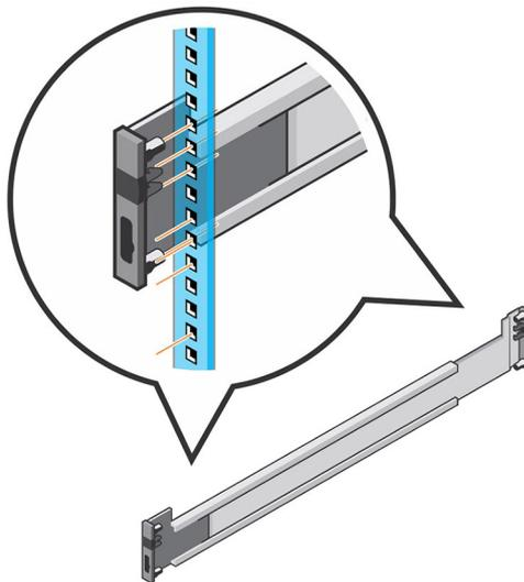
**Figure 27. Attach the Rails to the Rack**
