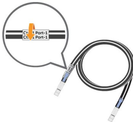
**Figure 41. Wrap Label Around Cable**
