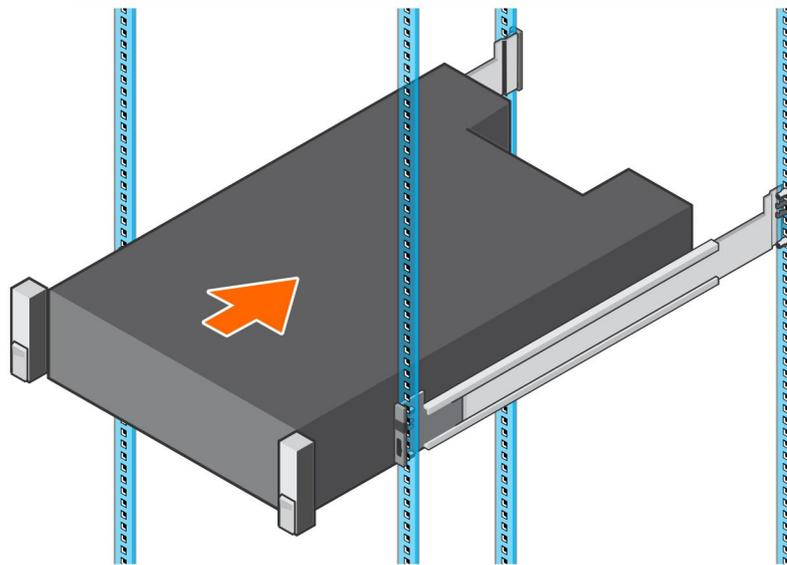
**Figure 28. Slide the Storage System Onto the Rails**
