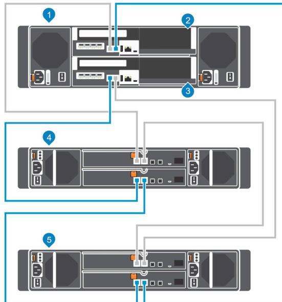
**Figure 63. Connect B-Side Cables to the New Expansion Enclosure**
