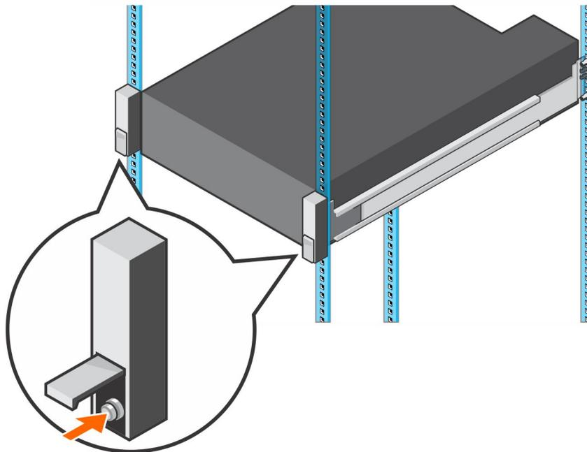
**Figure 29. Tighten the Screws**
