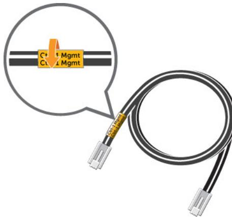
**Figure 44. Wrap Label Around Cable**
