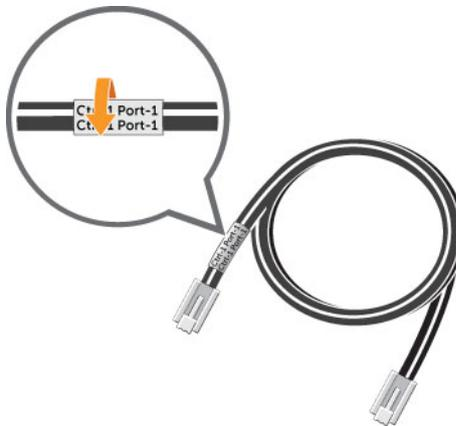
**Figure 38. Wrap Label Around Cable**
