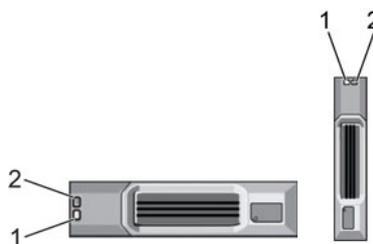
**Figure 8. SCv300 and SCv320 Expansion Enclosure Drive Indicators**
