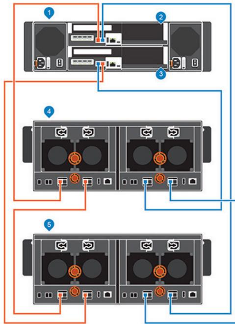
**Figure 48. SCv3000 and SCv3020 and Two SCv360 Expansion Enclosures**
