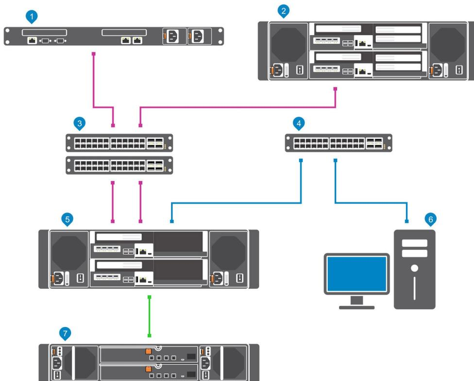
Figure 1. Storage System With Fibre Channel Front-End Connectivity
