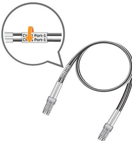
**Figure 33. Wrap Label Around Cable**
