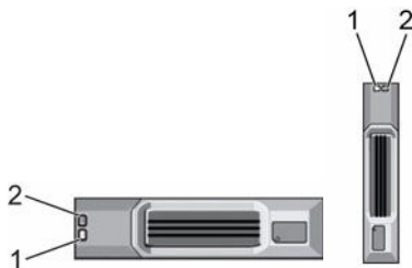
Figure 13. SCv2000/SCv2020 Storage System Drive Indicators
