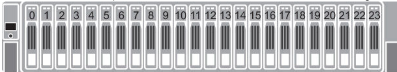
Figure 15. SCv2020 Storage System Drive Numbering
