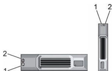
Figure 20. SC100/SC120 Expansion Enclosure Drive Indicators
