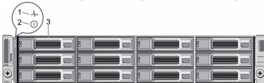
Figure 16. SC100 Front-Panel Features and Indicators
