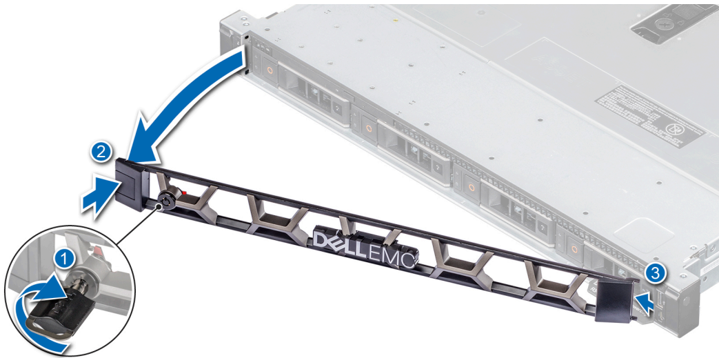
Figure 16. Removing the front bezel
