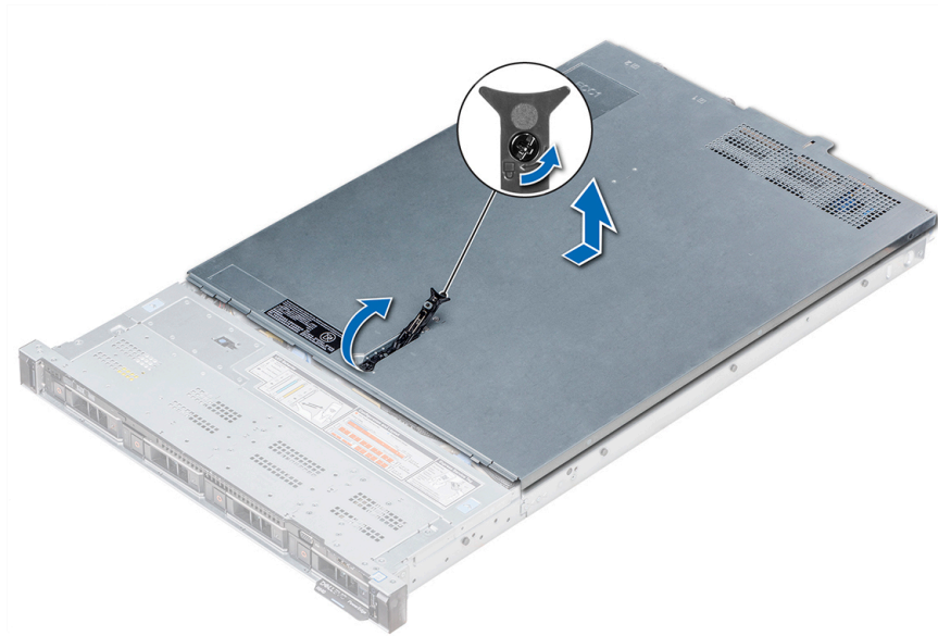
Figure 24. Removing the system cover
