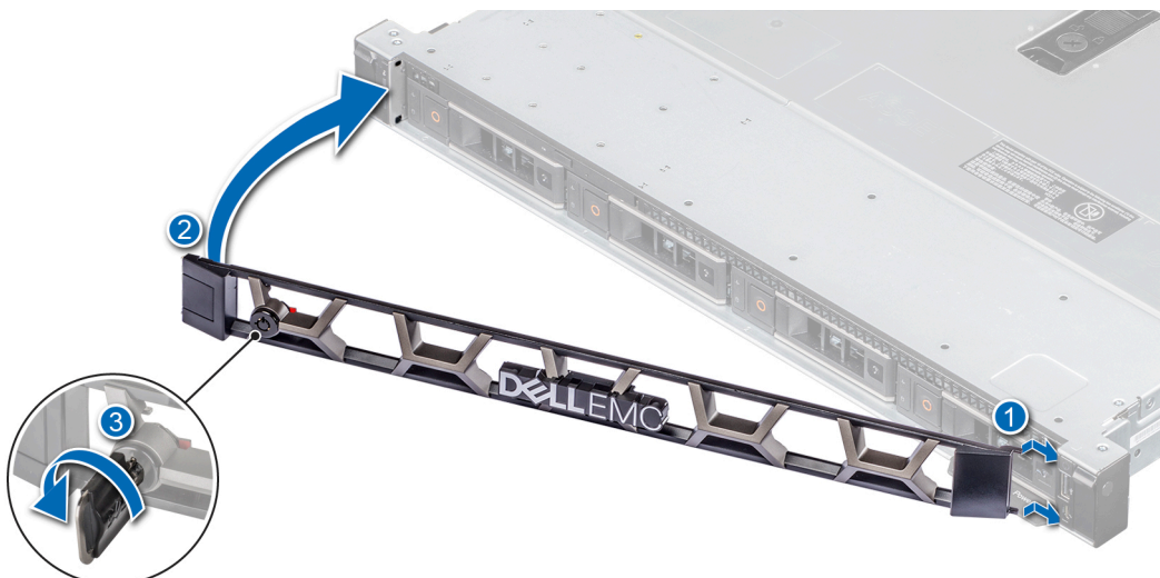
Figure 17. Installing the front bezel
