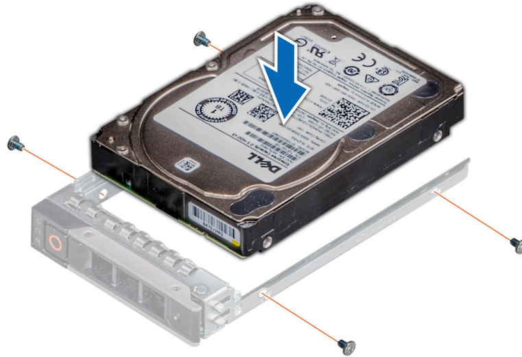
Figure 23. Installing a drive into the drive carrier
