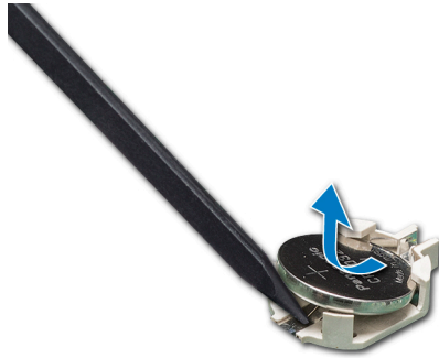
Figure 90. Removing the system battery
