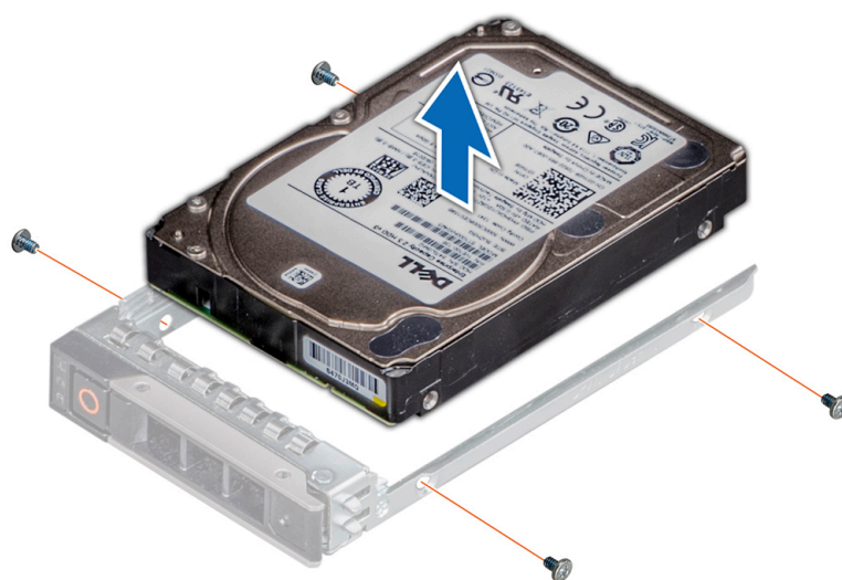
Figure 40. Removing the drive from the drive carrier
