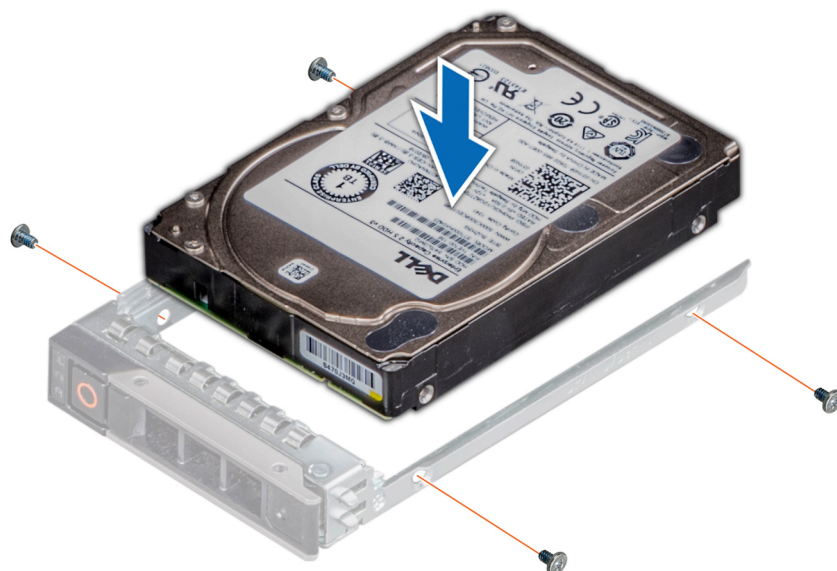
Figure 41. Installing a drive into the drive carrier
