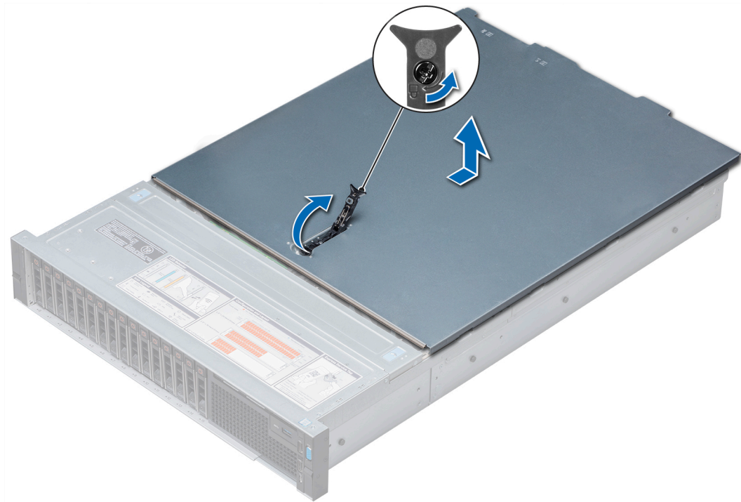
Figure 12. Removing the system cover
