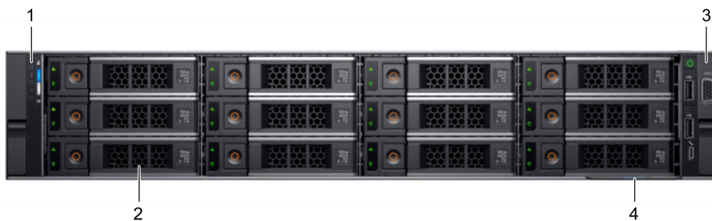
Figure 2. Front view of 12 x 3.5-inch drive system
