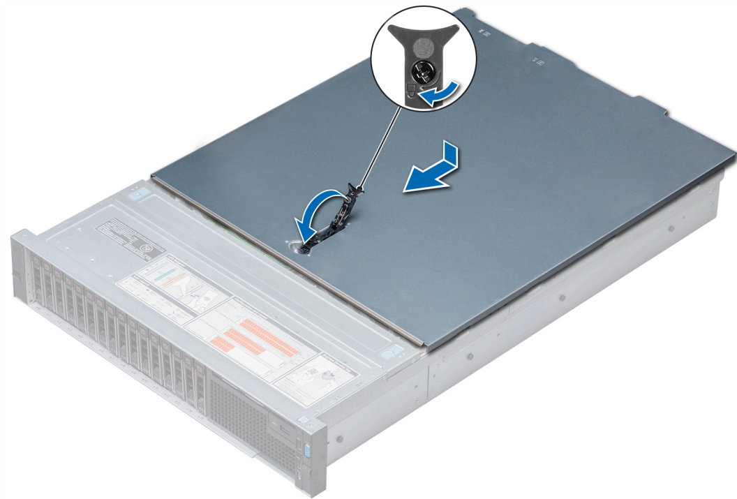
Figure 13. Installing the system cover
