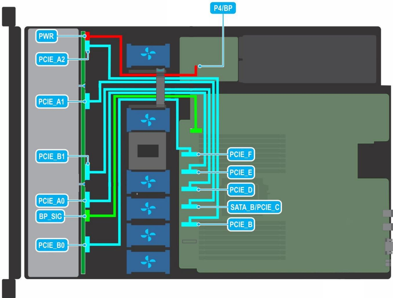
**Figure 2. Cable routing - 10 x 2.5 inch NVMe drive backplane**
