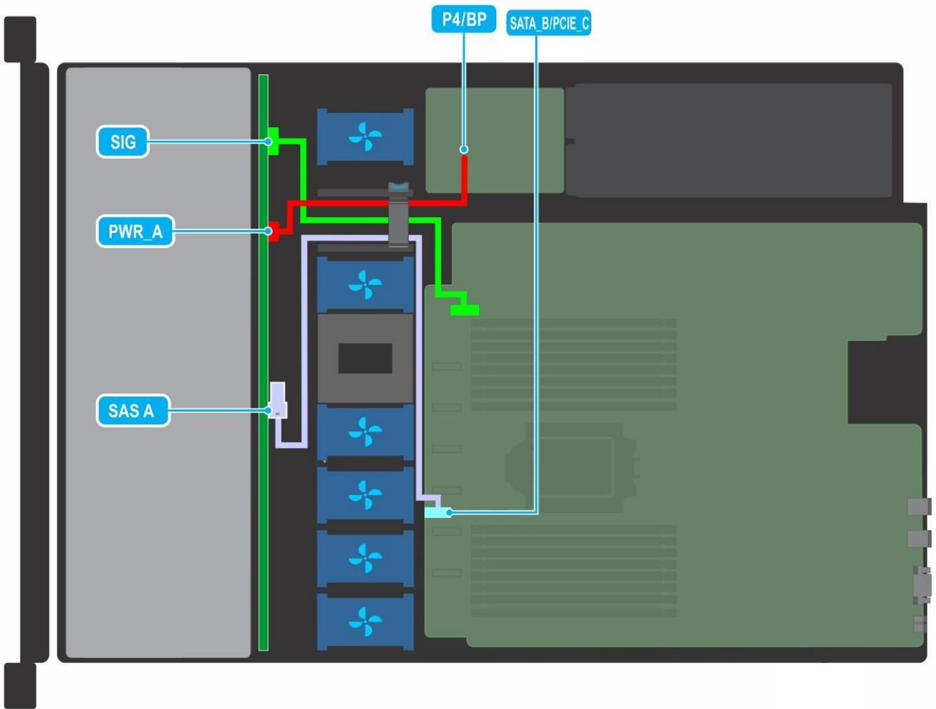
Figure 1. Cable routing - 4 x 3.5 inch SATA drive backplane
