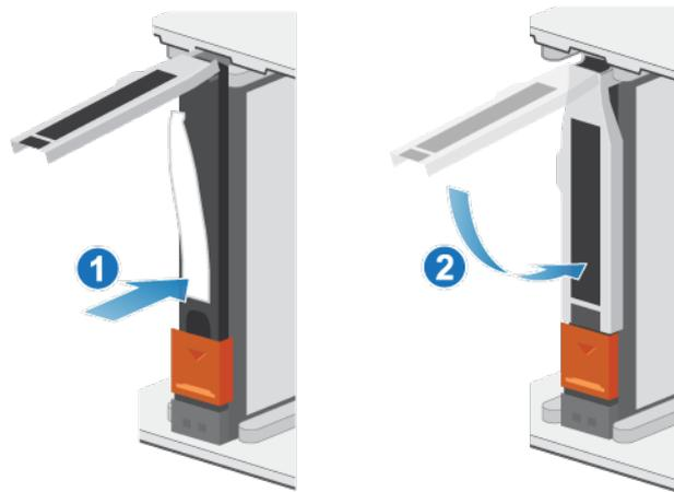
Figure 37. Installing a drive
