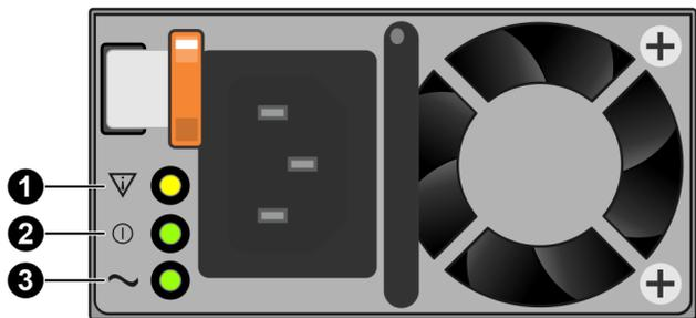
Figure 184. NVMe expansion enclosure power supply LEDs
