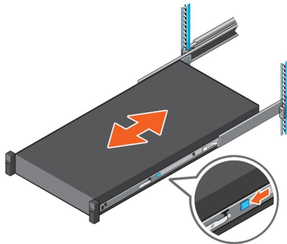
**Figure 31. Slide system into the rack**
