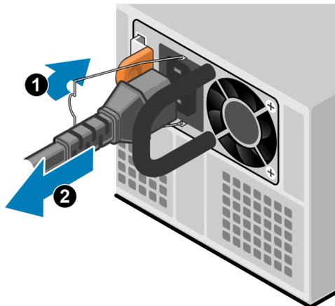
Figure 186. Removing a power supply
