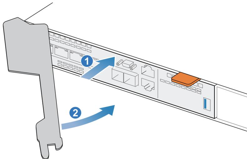
**Figure 230. Installing the embedded module**
