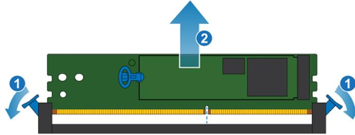
Figure 261. Removing the M.2 boot module adaptor
