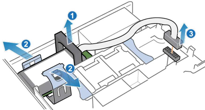
**Figure 273. Releasing the internal battery backup module**
