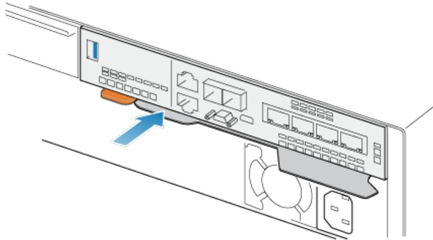
**Figure 81. Locking the release lever**
