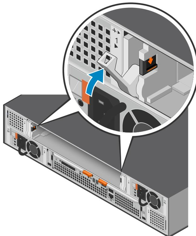
**Figure 204. Locking the DIB into place**
