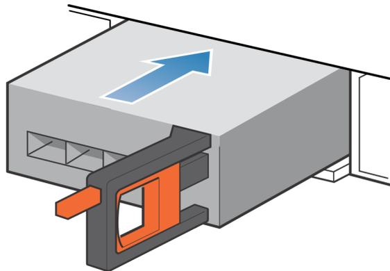
Figure 226. Installing an I/O module
