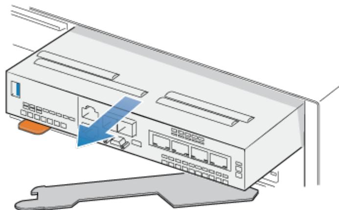
**Figure 66. Removing the embedded module from the system**
