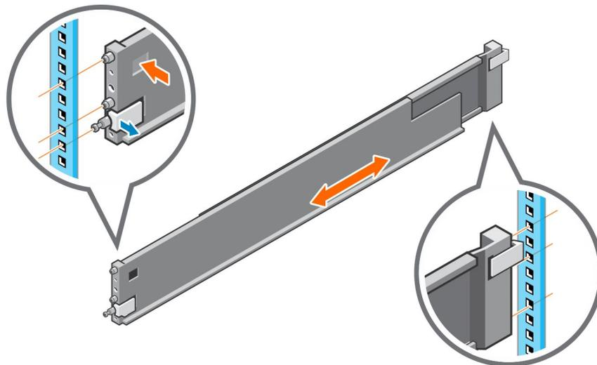
**Figure 8. Installing the rails**
