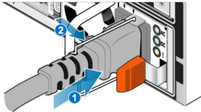
Figure 63. Inserting the power cable
