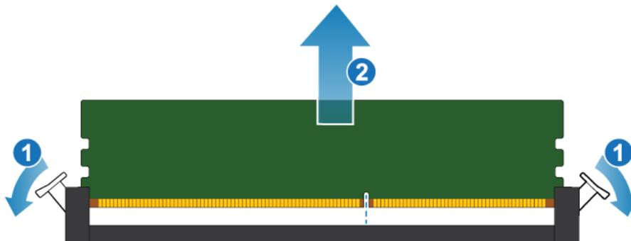
Figure 116. Removing the DIMM
