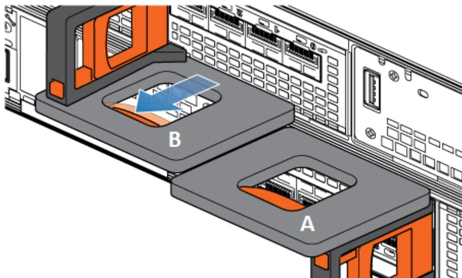
**Figure 149. Disengaging the locking mechanism for node B**
