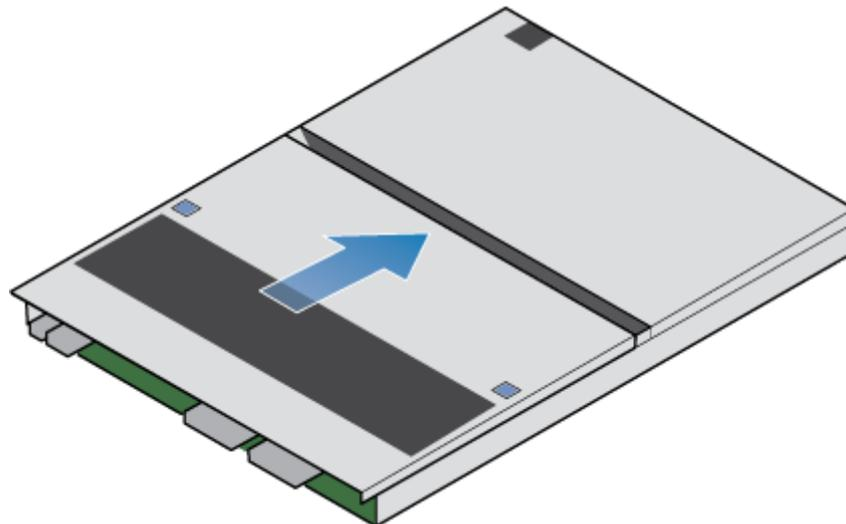
**Figure 268. Securing the top cover**
