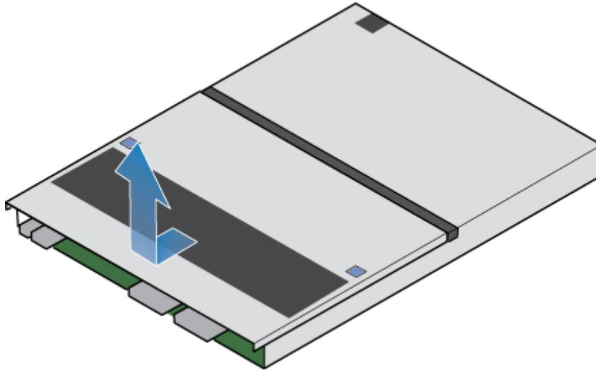
Figure 152. Removing the top cover
