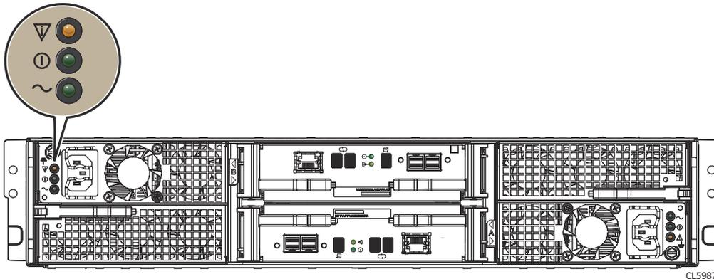
Figure 170. Fault LED on an AC power/cooling module
