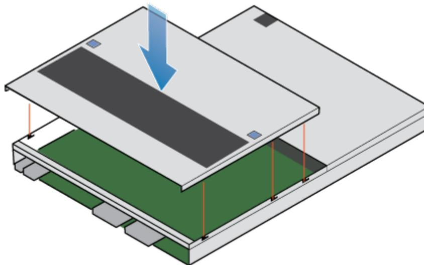
**Figure 118. Aligning the top cover**
