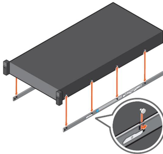
**Figure 43. Attach the inner rails to the system**
