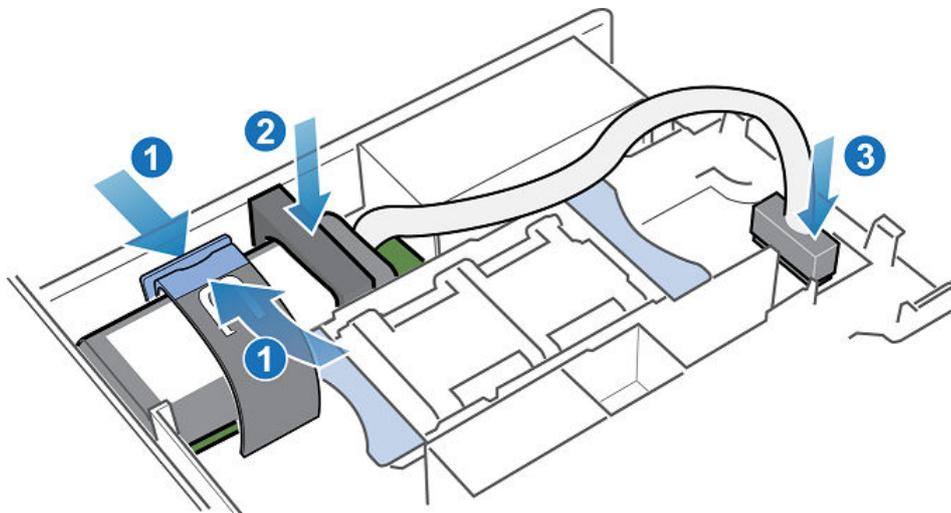
**Figure 240. Connecting the internal battery backup module cable to the motherboard**
