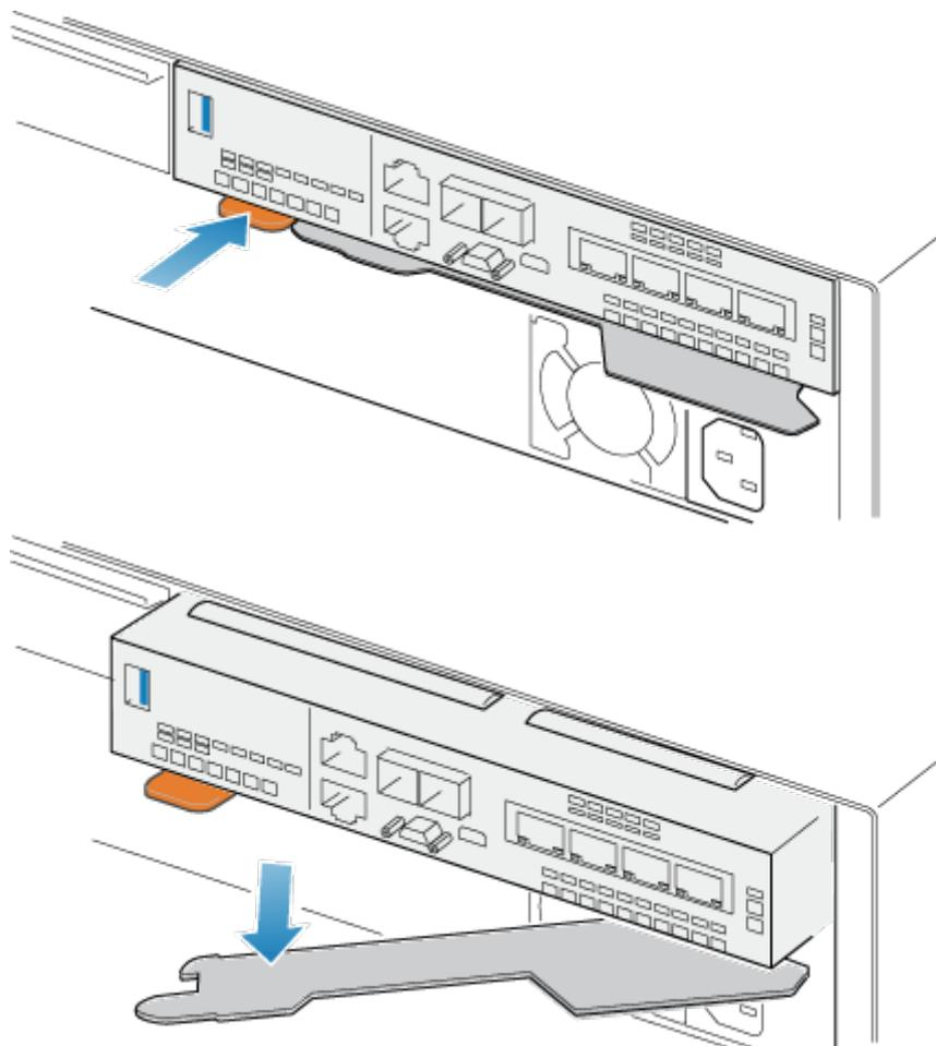
**Figure 74. Releasing the lever on the embedded module**
