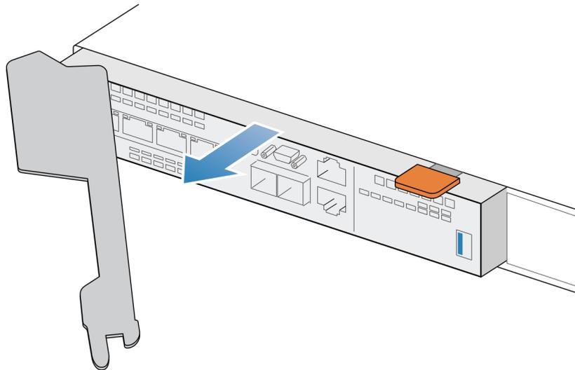
**Figure 229. Removing the embedded module from the system**
