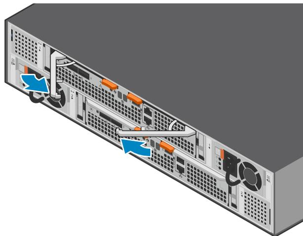
**Figure 211. Locking the Access Module into place**
