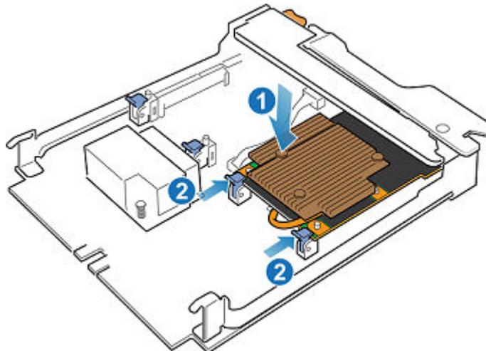
**Figure 70. Locking the 4-port card into position**
