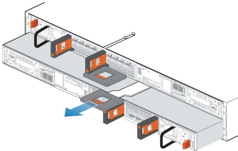
Figure 220. Removing the node
