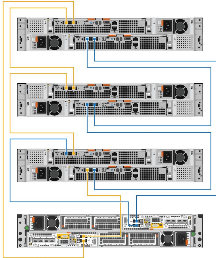
**Figure 48. Cabling three expansion enclosures**
