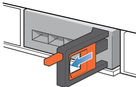
Figure 250. Releasing the I/O module
