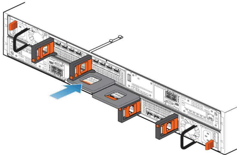
**Figure 270. Installing the node**
