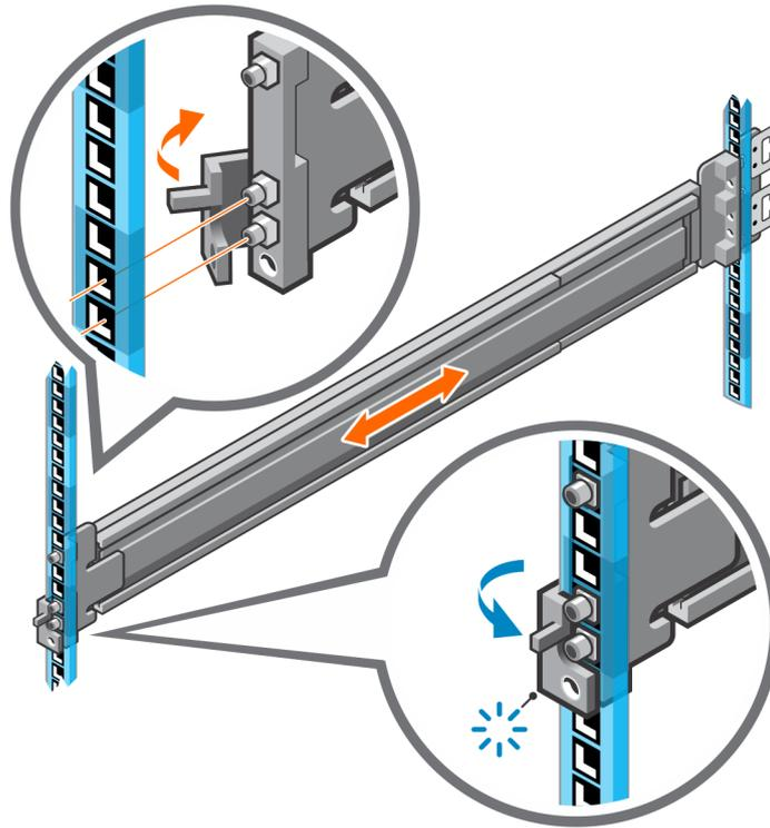
**Figure 26. Installing the NVMe expansion enclosure rails (front)**
