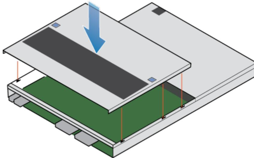
**Figure 267. Aligning the top cover**
