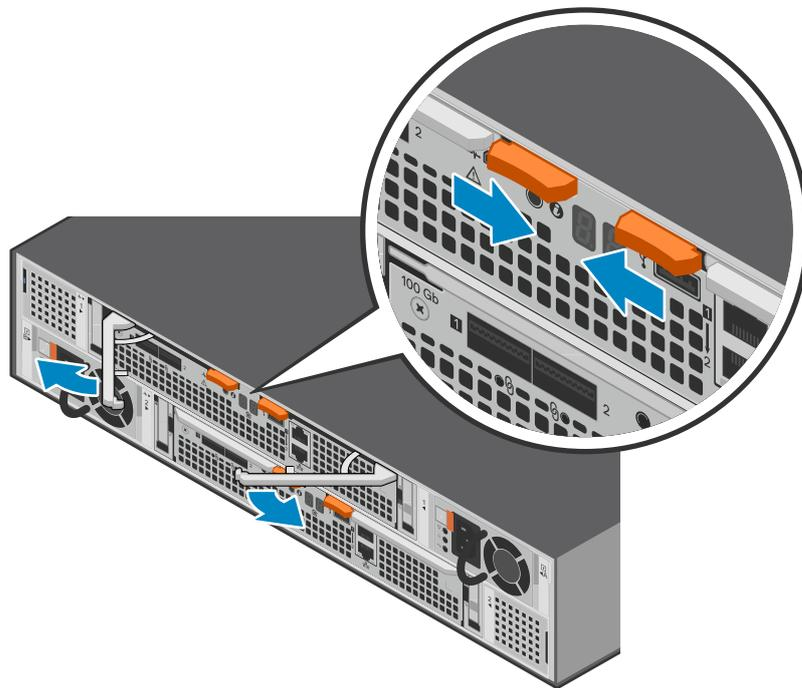
**Figure 205. Releasing the Access Module**
