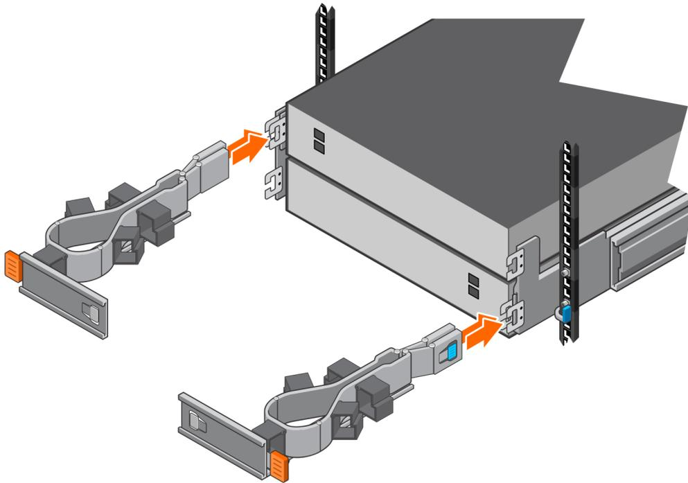
**Figure 46. Installing the cable management arms**
