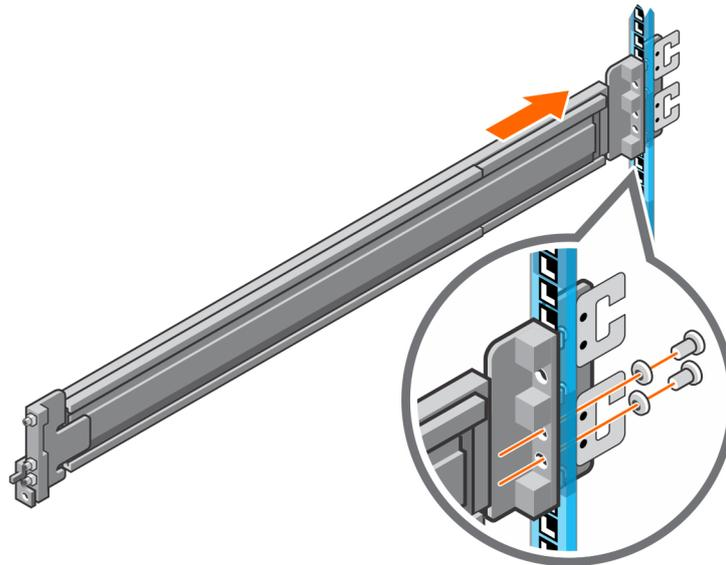
Figure 25. Installing the NVMe expansion enclosure rails (rear)
