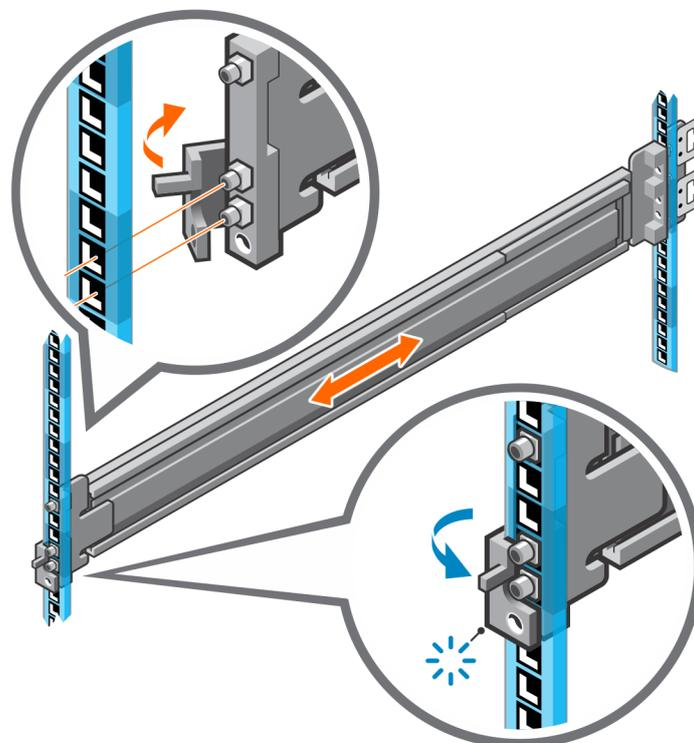
**Figure 40. Installing the NVMe expansion enclosure rails (front)**
