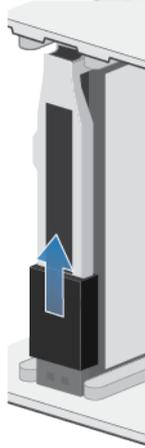
**Figure 52. Pushing up the drive latch cover**
