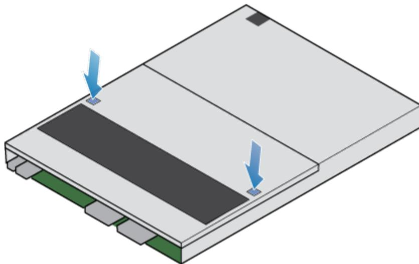
**Figure 258. Releasing the top cover**
