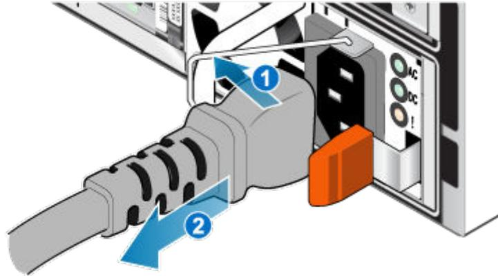
**Figure 122. Removing the power cable**
