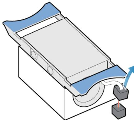
Figure 103. Disconnecting the fan power cable
