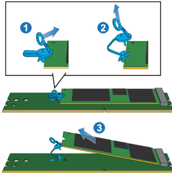
Figure 141. Removing the internal M.2 boot modules from the M.2 boot module adaptor
