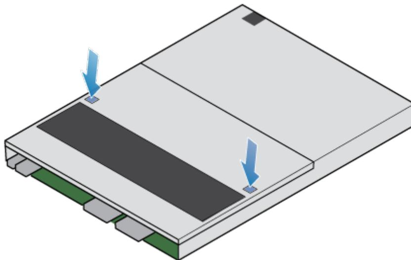
**Figure 151. Releasing the top cover**
