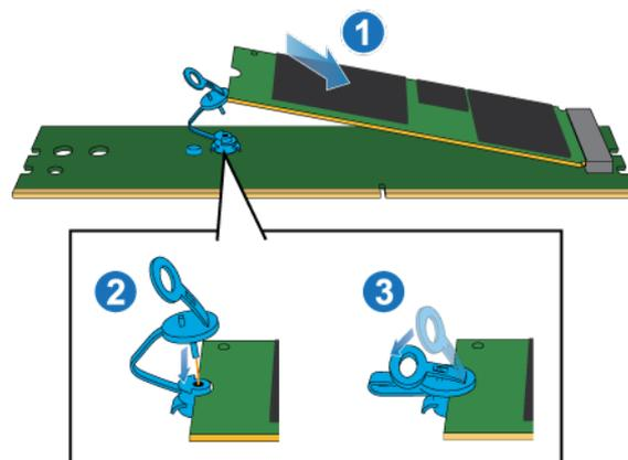
Figure 142. Installing the internal M.2 boot modules into the M.2 boot module adaptor
