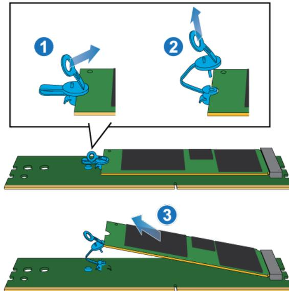
Figure 128. Removing the internal M.2 boot module from the M.2 boot module adaptor
