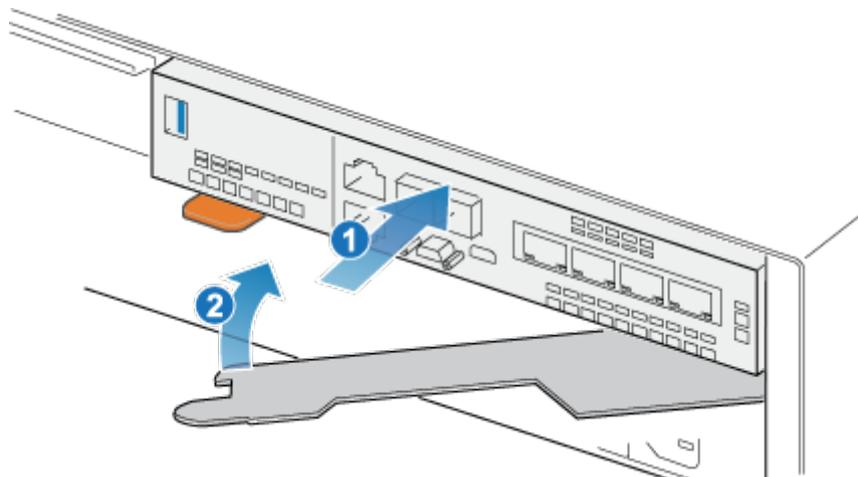
**Figure 80. Installing the embedded module**
