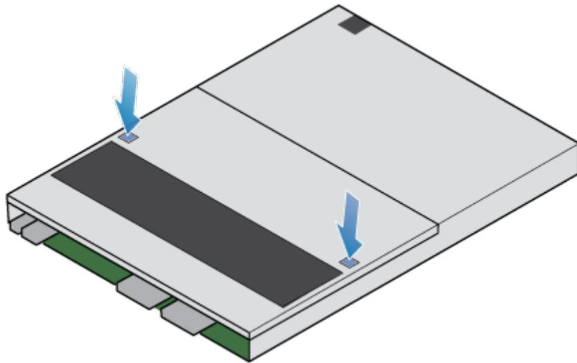
Figure 258. Releasing the top cover
