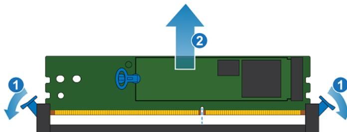
Figure 140. Removing the M.2 boot module adaptor
