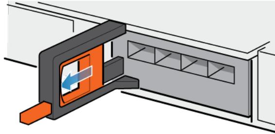
Figure 94. Releasing the I/O module
