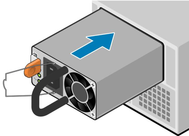
Figure 187. Installing a power supply
