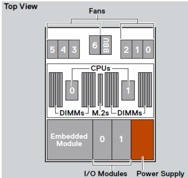
Figure 247. Top view of the node
