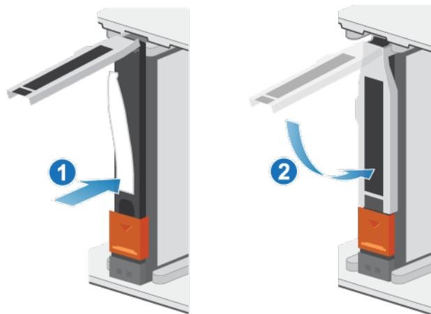
**Figure 212. Installing an NVMe NVRAM drive**
