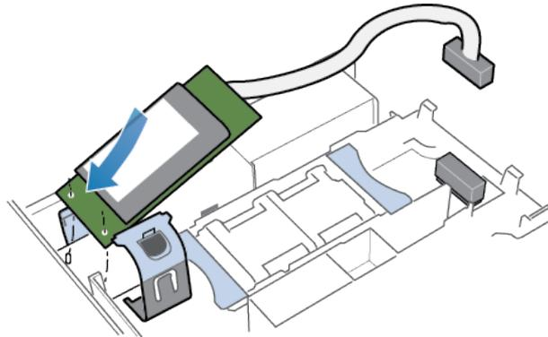
**Figure 275. Placing the internal battery backup module into position**
