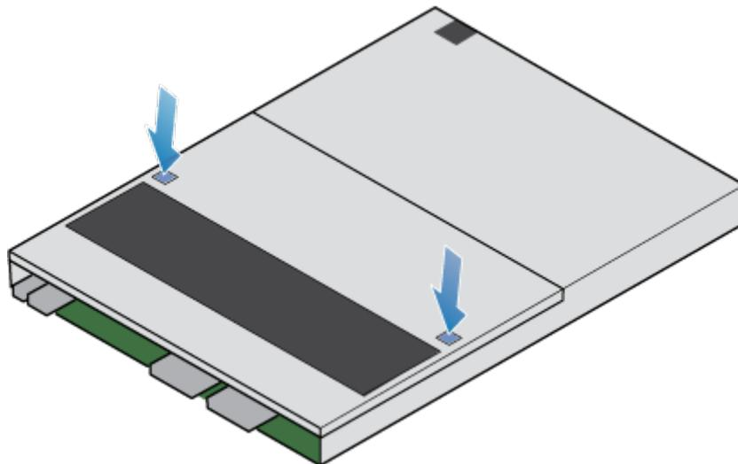
**Figure 138. Releasing the top cover**
