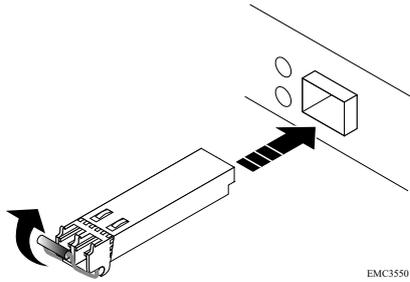
**Figure 92. Installing an SFP module**
