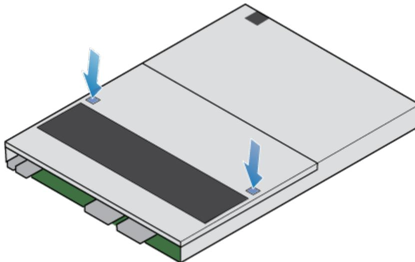
**Figure 138. Releasing the top cover**
