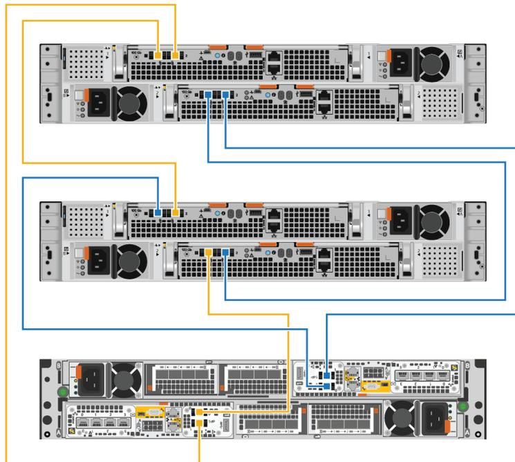
**Figure 34. Cabling two expansion enclosures**
