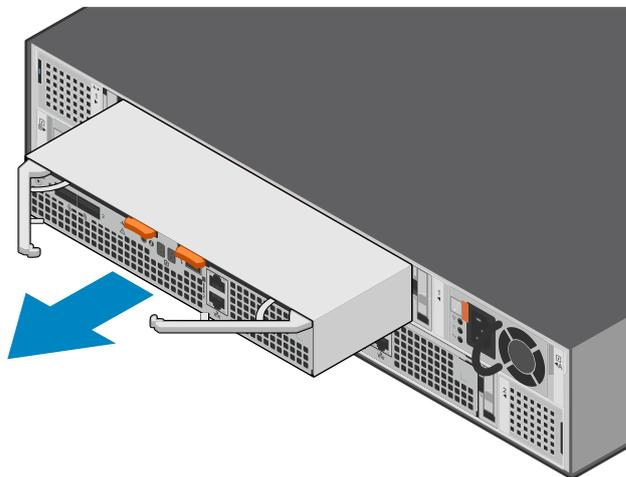
**Figure 198. Removing the Access Module**
