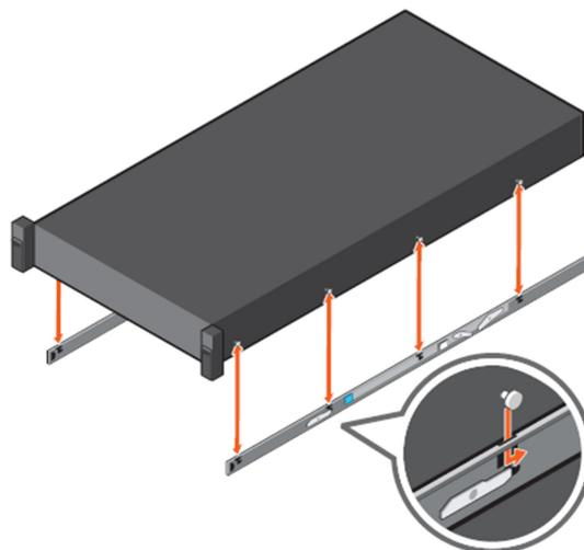
**Figure 29. Attach the inner rails to the system**
