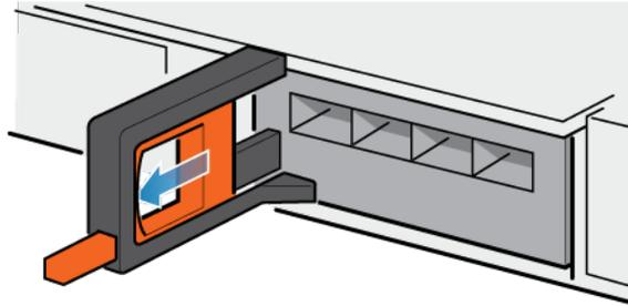
Figure 94. Releasing the I/O module
