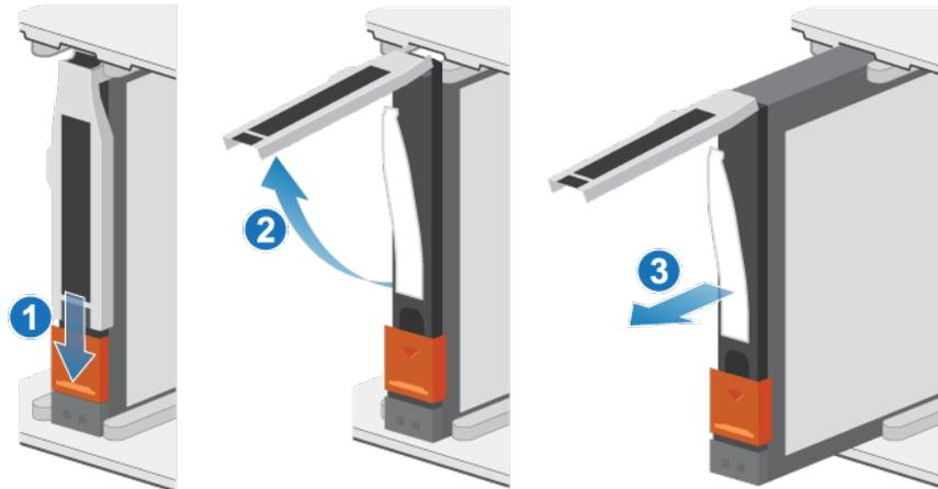
Figure 162. Removing a drive
