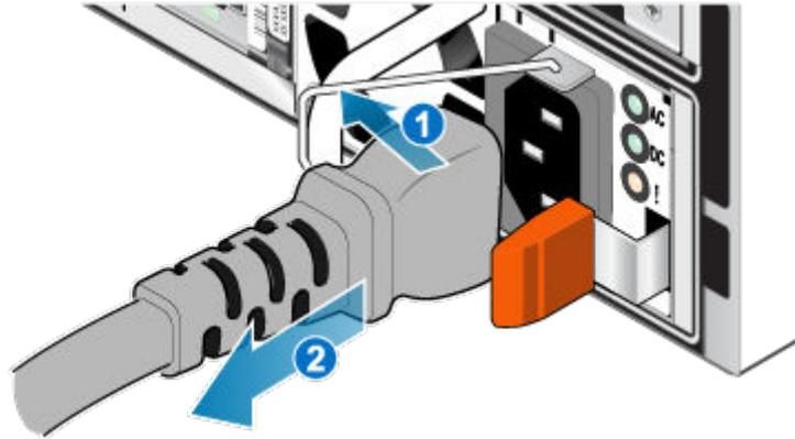
**Figure 148. Removing the power cable**
