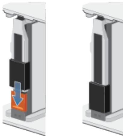
**Figure 58. Pushing the latch cover into place**
