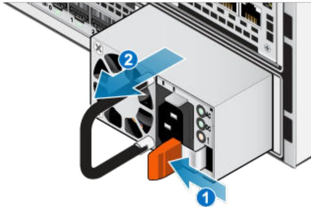
**Figure 61. Removing a power supply**
