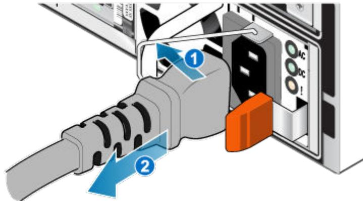
**Figure 218. Removing the power cable**
