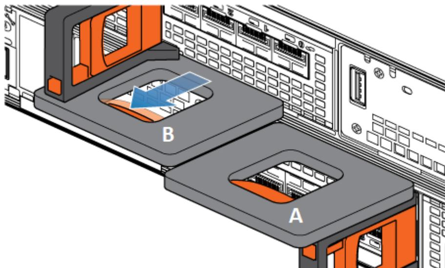
**Figure 99. Disengaging the locking mechanism for node B**
