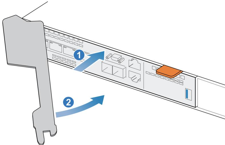
**Figure 230. Installing the embedded module**
