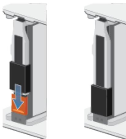
**Figure 213. Pushing the latch cover into place**
