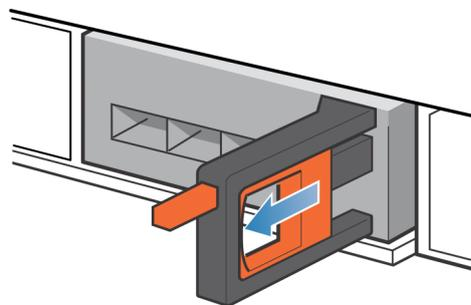
Figure 224. Releasing the I/O module
