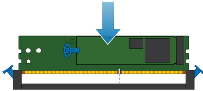
Figure 130. Installing the M.2 boot module adaptor
