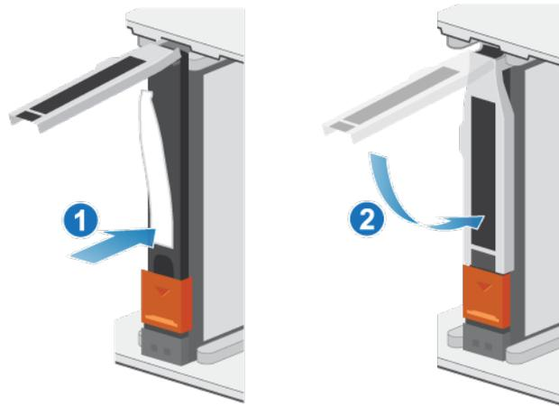
**Figure 54. Installing a 2.5" drive**
