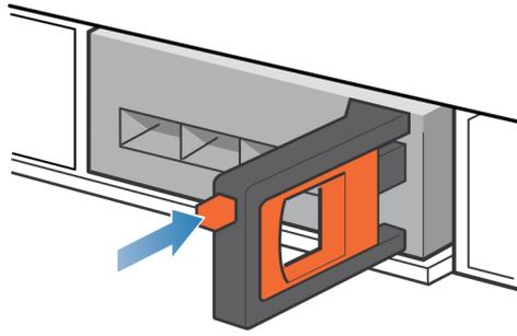
Figure 227. Locking in the I/O module
