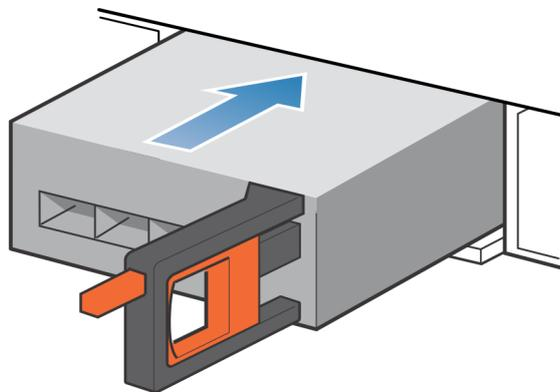
Figure 252. Installing an I/O module
