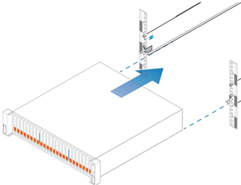
**Figure 10. Installing the enclosure**
