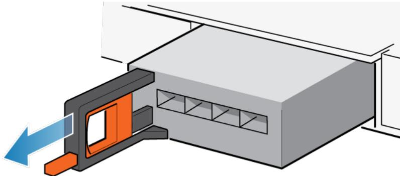
Figure 95. Removing the I/O module
