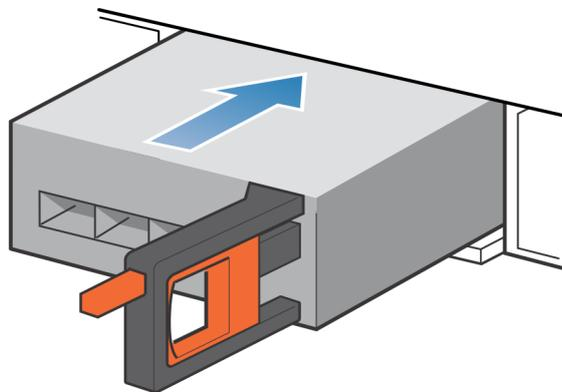
Figure 226. Installing an I/O module
