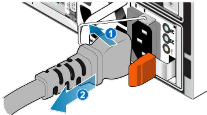
**Figure 214. Removing the power cable**
