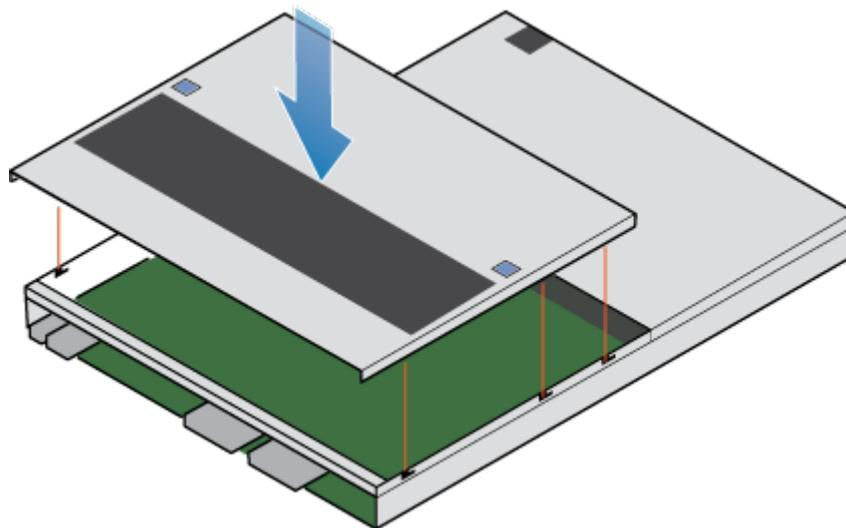
**Figure 118. Aligning the top cover**
