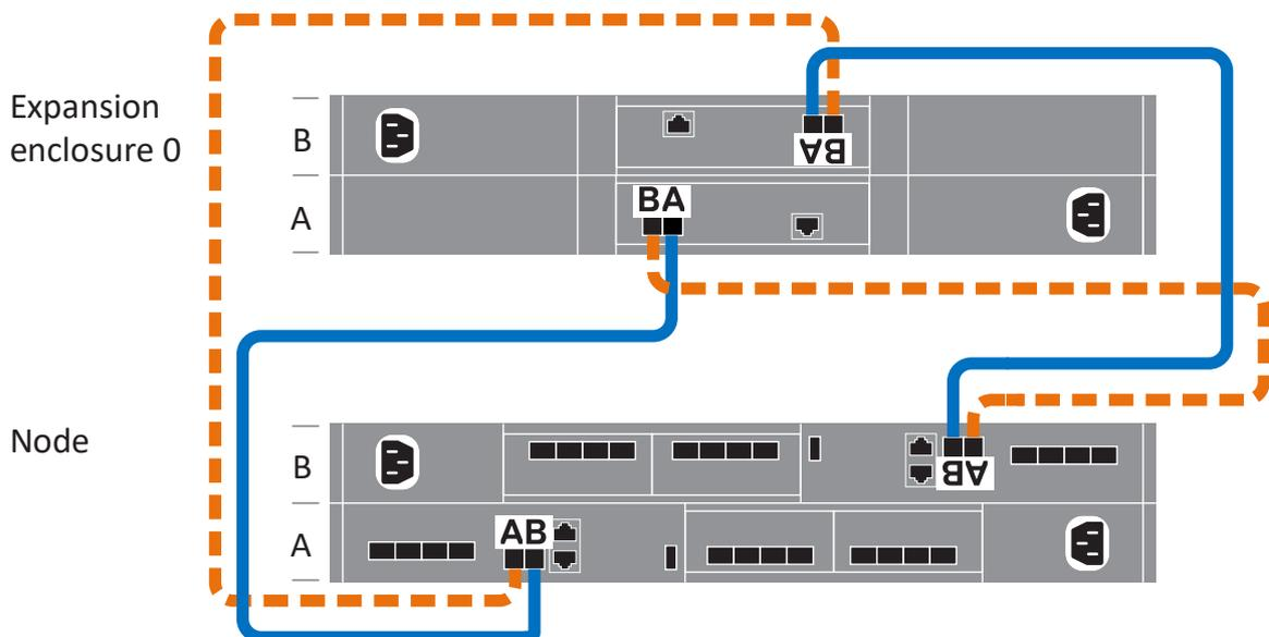
Figure 14. Cabling the base enclosure to one expansion enclosure
