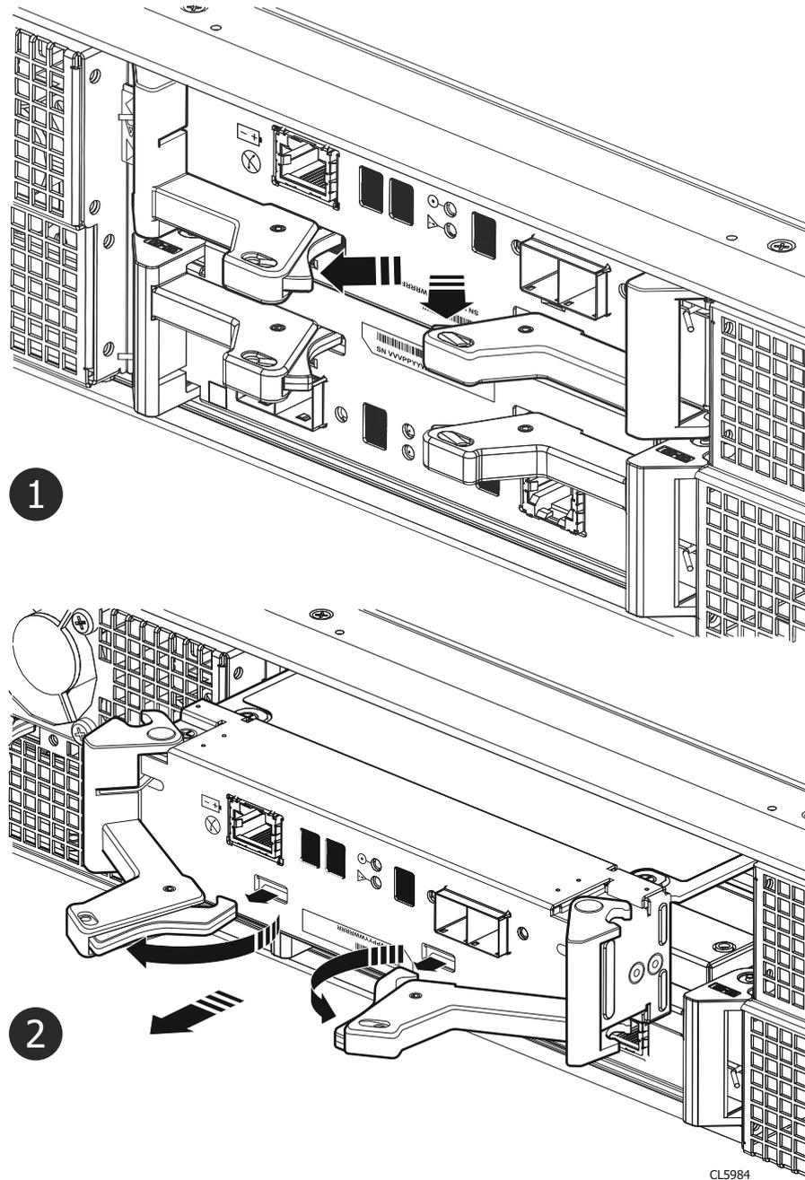
Figure 167. Removing an LCC
