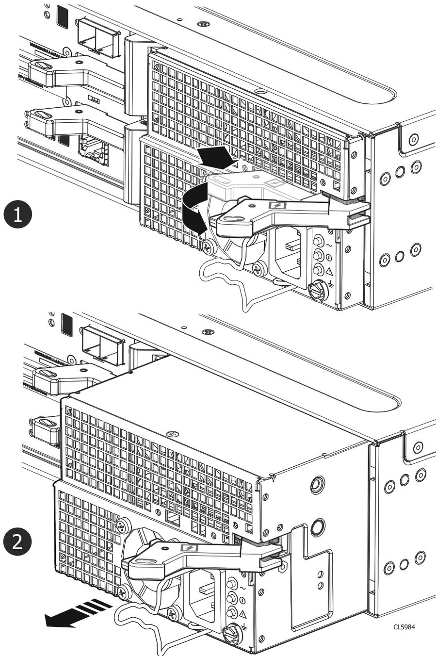
Figure 173. Removing an AC power/cooling module
