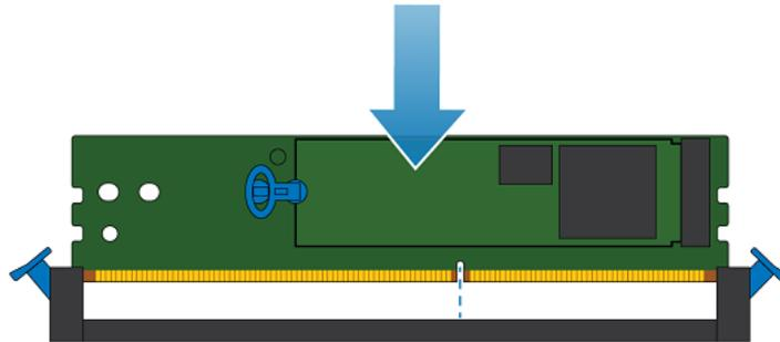
Figure 236. Installing the M.2 boot module adaptor
