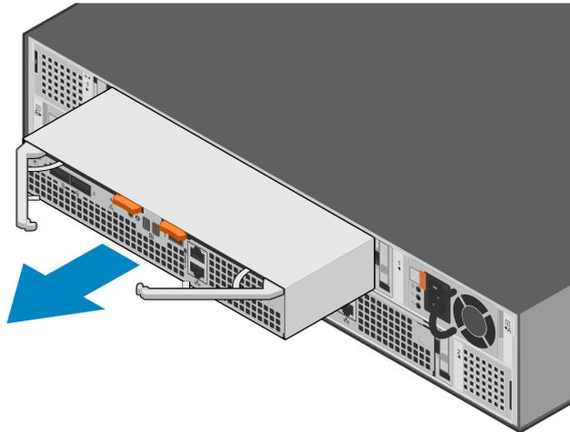
Figure 206. Removing the Access Module
