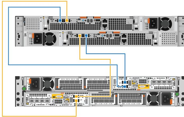
**Figure 33. Cabling a single expansion enclosure**
