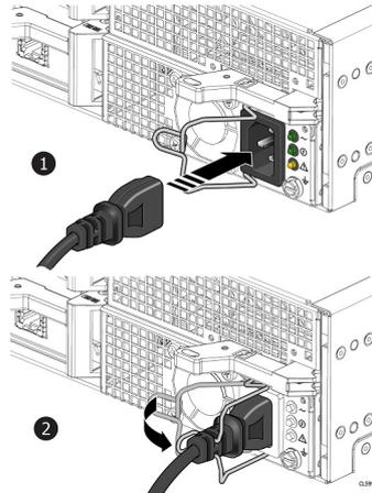
Figure 22. Attaching a power cable
