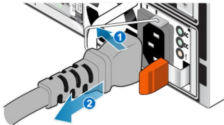
**Figure 218. Removing the power cable**
