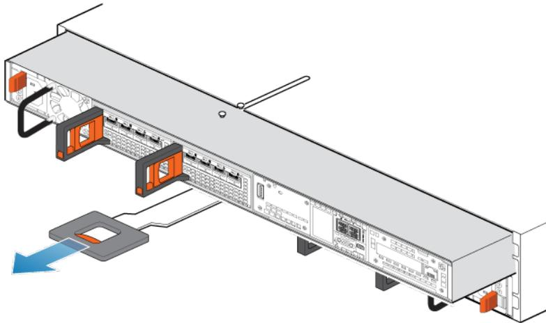
**Figure 124. Removing the node**
