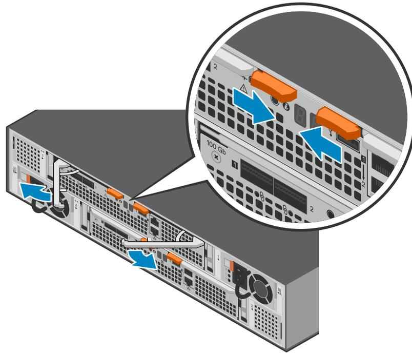
**Figure 197. Releasing the Access Module**
