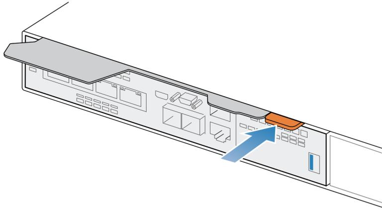
**Figure 257. Locking the release lever**
