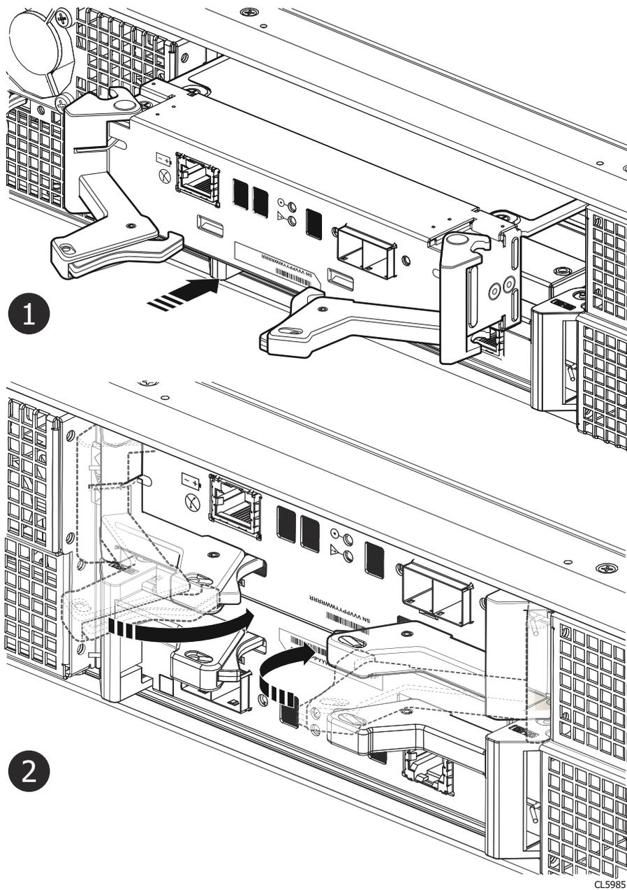
**Figure 168. Installing an LCC**
