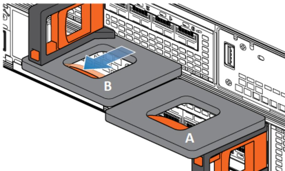
**Figure 123. Disengaging the locking mechanism for node B**
