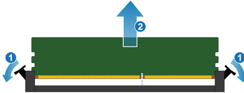
Figure 208. Removing the DIMM
