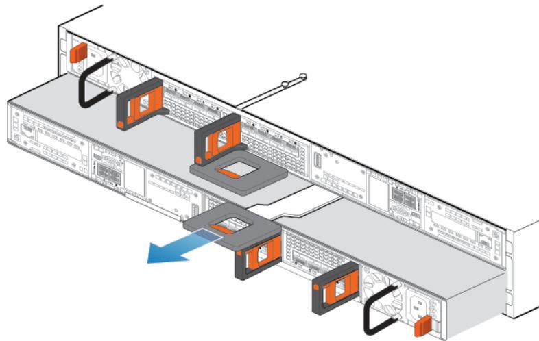
Figure 220. Removing the node
