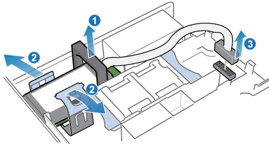
**Figure 237. Releasing the internal battery backup module**
