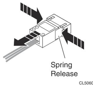
**Figure 172. Unplugging the power cord from a DC power supply/cooling module**
