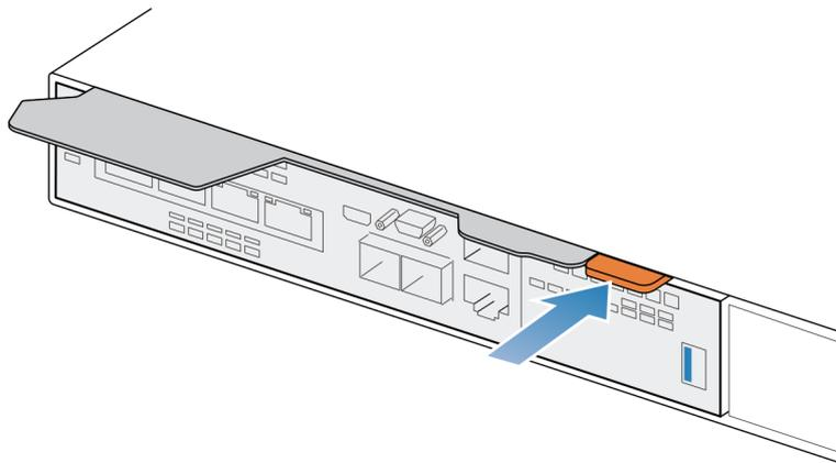
Figure 228. Releasing the lever on the embedded module
