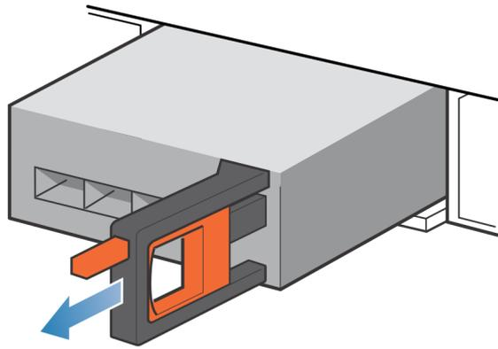
Figure 225. Removing the I/O module
