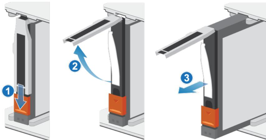
**Figure 53. Removing a 2.5" drive**
