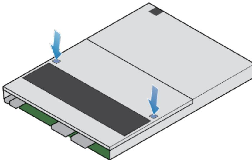
Figure 232. Releasing the top cover
