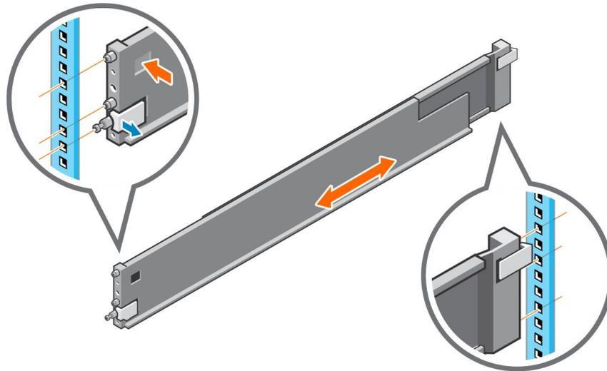
**Figure 1. Installing the rails**
