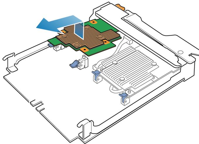
Figure 86. Removing the 2-port 100GbE card
