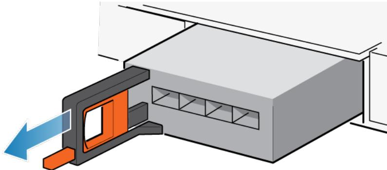
Figure 95. Removing the I/O module
