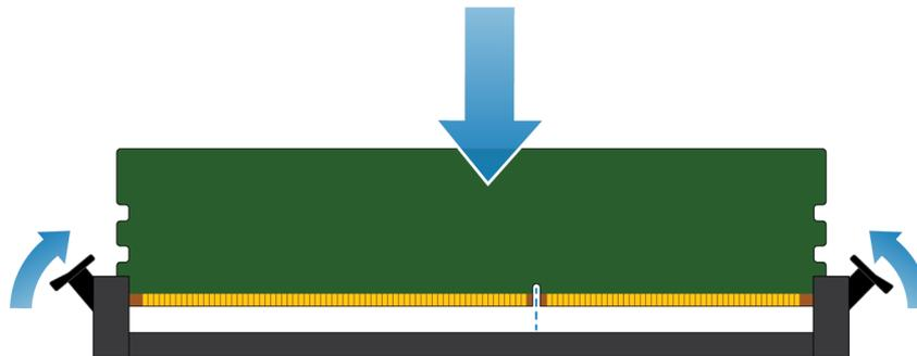
Figure 209. Installing the DIMM
