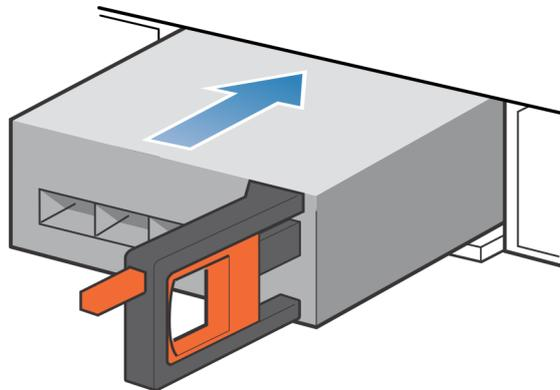
Figure 252. Installing an I/O module
