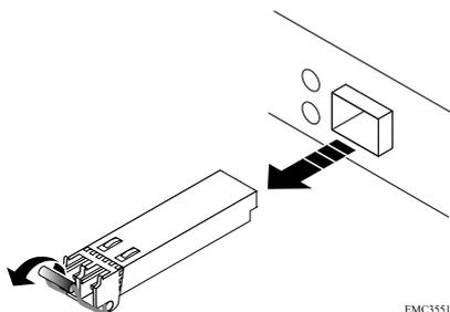
Figure 91. Removing an SFP module
