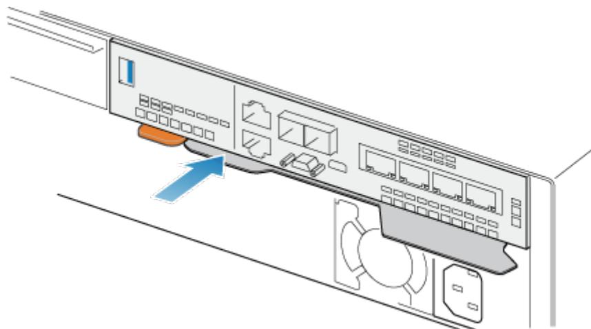
**Figure 90. Locking the release lever**
