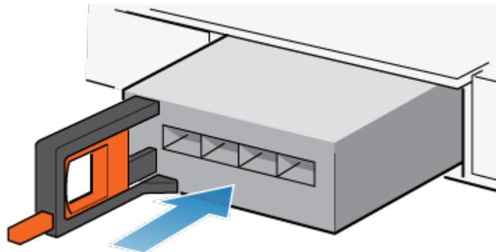
Figure 96. Installing an I/O module
