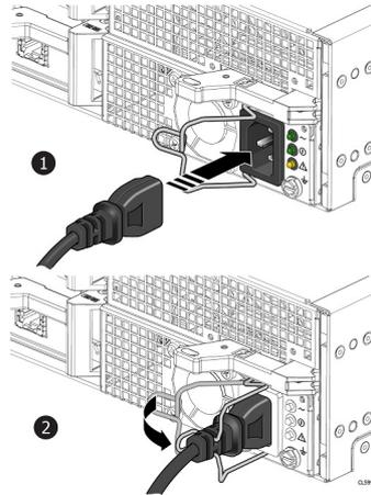
Figure 22. Attaching a power cable
