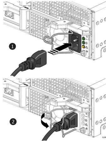
**Figure 15. Attaching a power cable**
