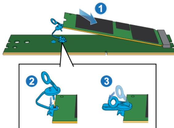
Figure 129. Installing the internal M.2 boot module into the M.2 boot module adaptor
