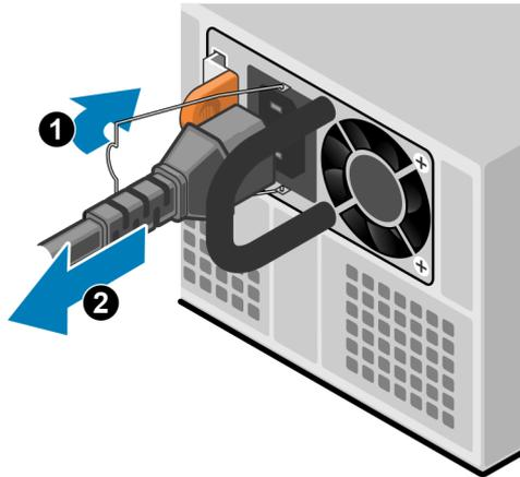
Figure 185. Removing the power cable
