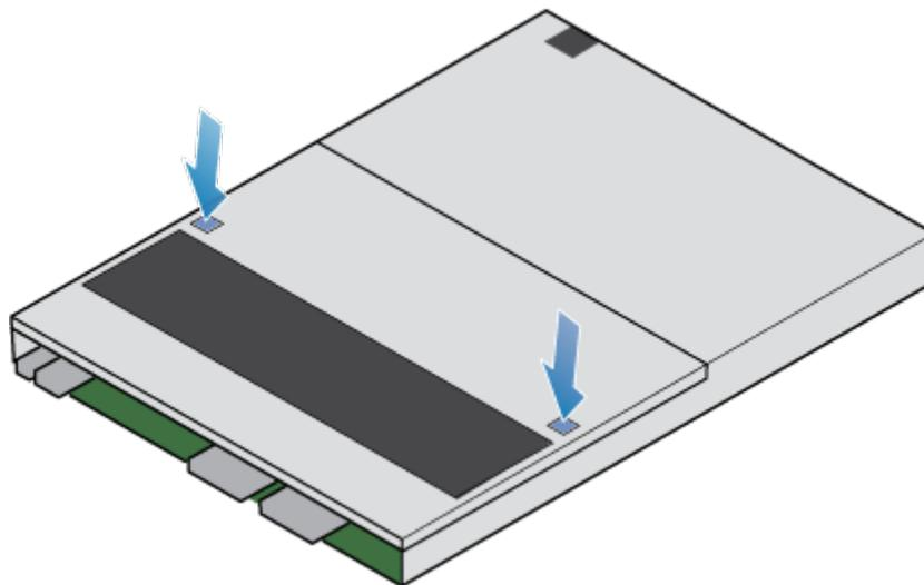
**Figure 101. Releasing the top cover**
