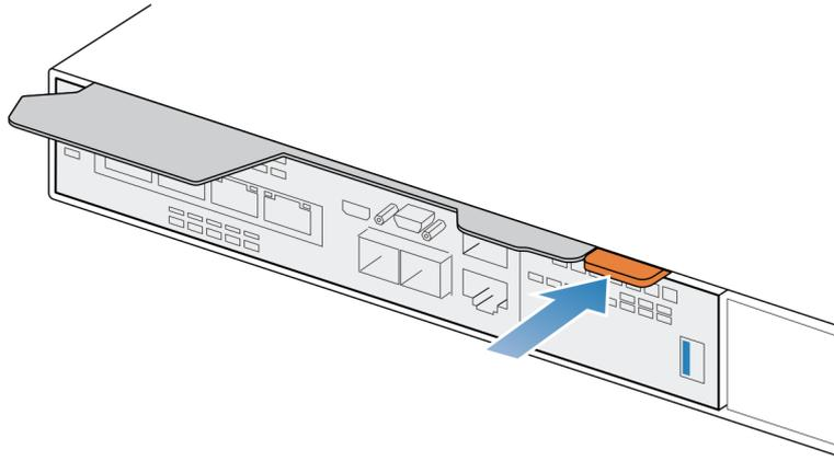
Figure 231. Locking the release lever
