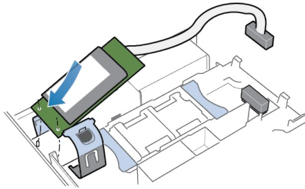
**Figure 265. Positioning the internal battery backup module**
