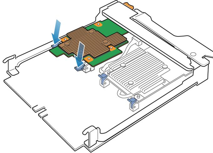
Figure 85. Opening the retaining tabs
