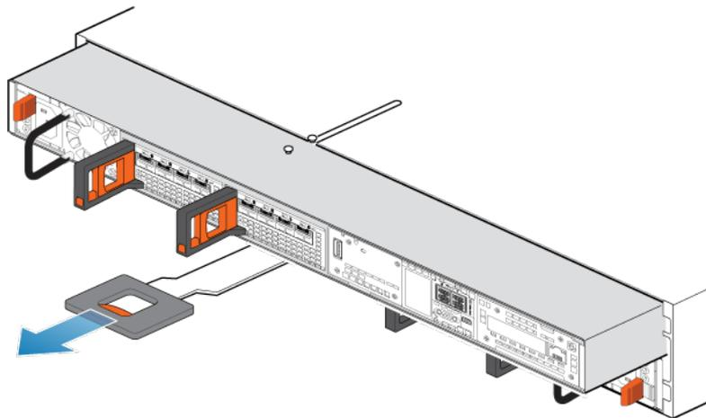
**Figure 246. Removing the node**
