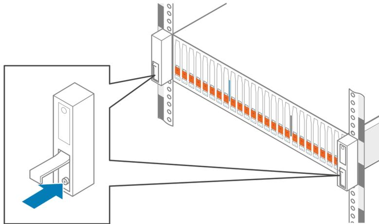
Figure 11. Tightening the captive screws
