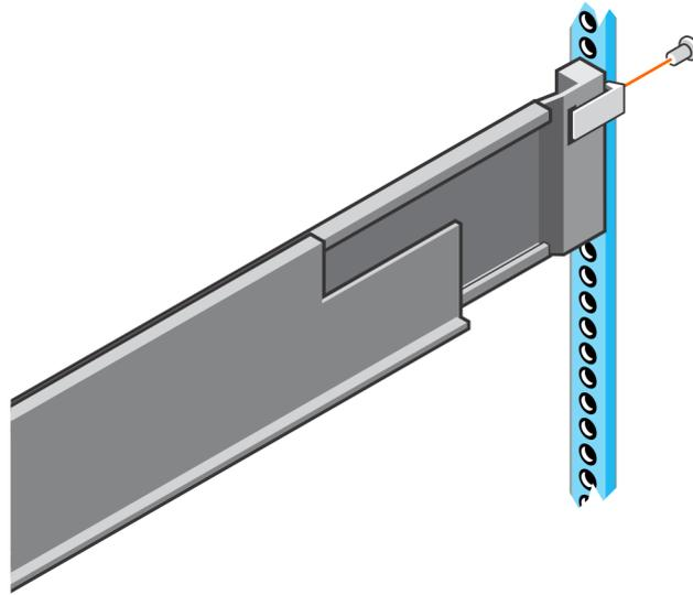
**Figure 9. Installing the security screws**
