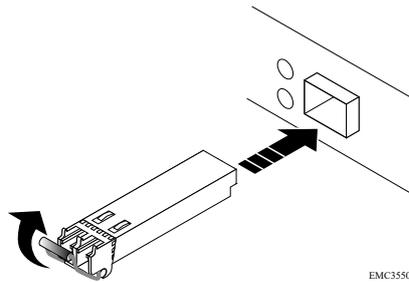
**Figure 92. Installing an SFP module**
