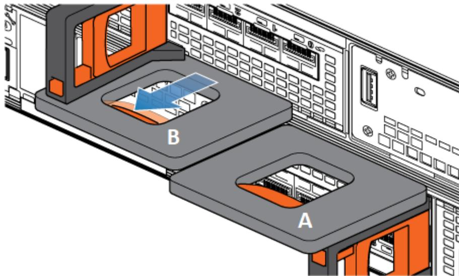
**Figure 111. Disengaging the locking mechanism for node B**
