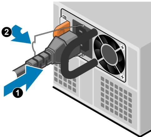
Figure 188. Inserting the power cable
