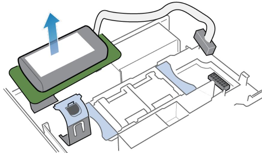
**Figure 264. Removing the internal battery backup module from the motherboard**
