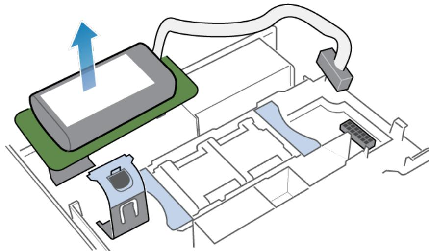
**Figure 238. Removing the internal battery backup module from the motherboard**
