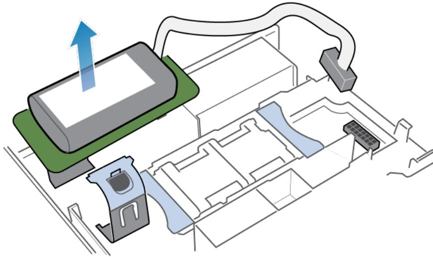
**Figure 274. Removing the internal battery backup module from the motherboard**
