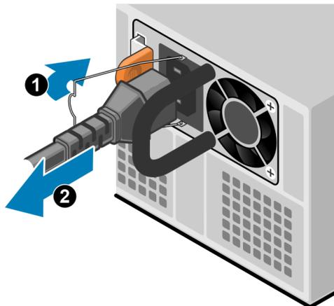
Figure 186. Removing a power supply
