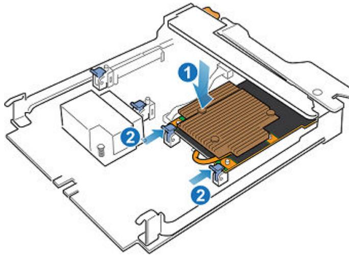
**Figure 79. Locking the 4-port card into position**
