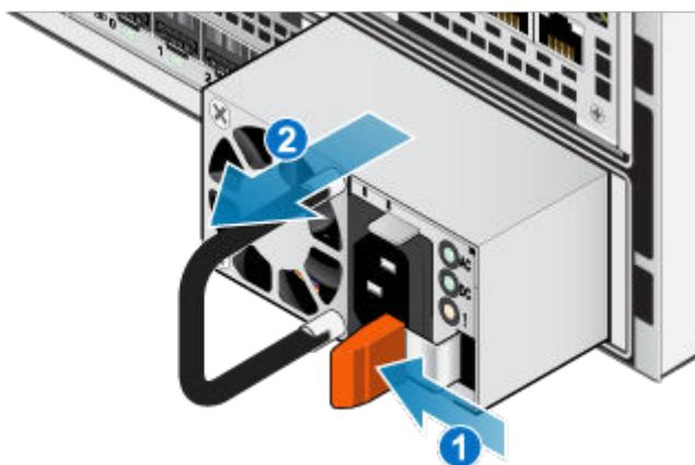
Figure 248. Removing a power supply
