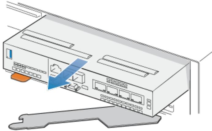
**Figure 75. Removing the embedded module from the system**
