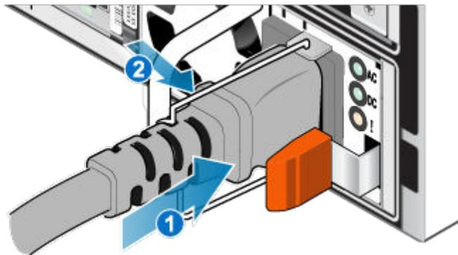
Figure 63. Inserting the power cable
