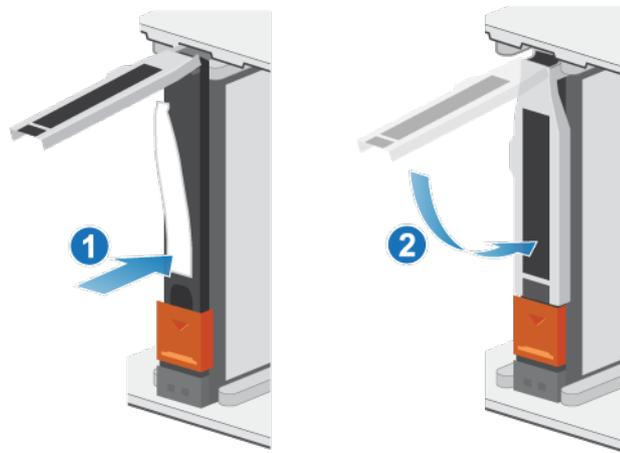
Figure 178. Installing a drive
