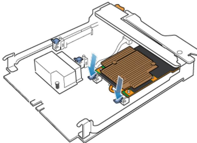
**Figure 76. Opening the retaining tabs**
