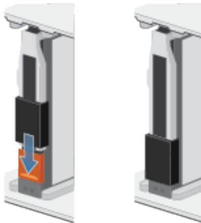
**Figure 55. Pushing the latch cover into place**
