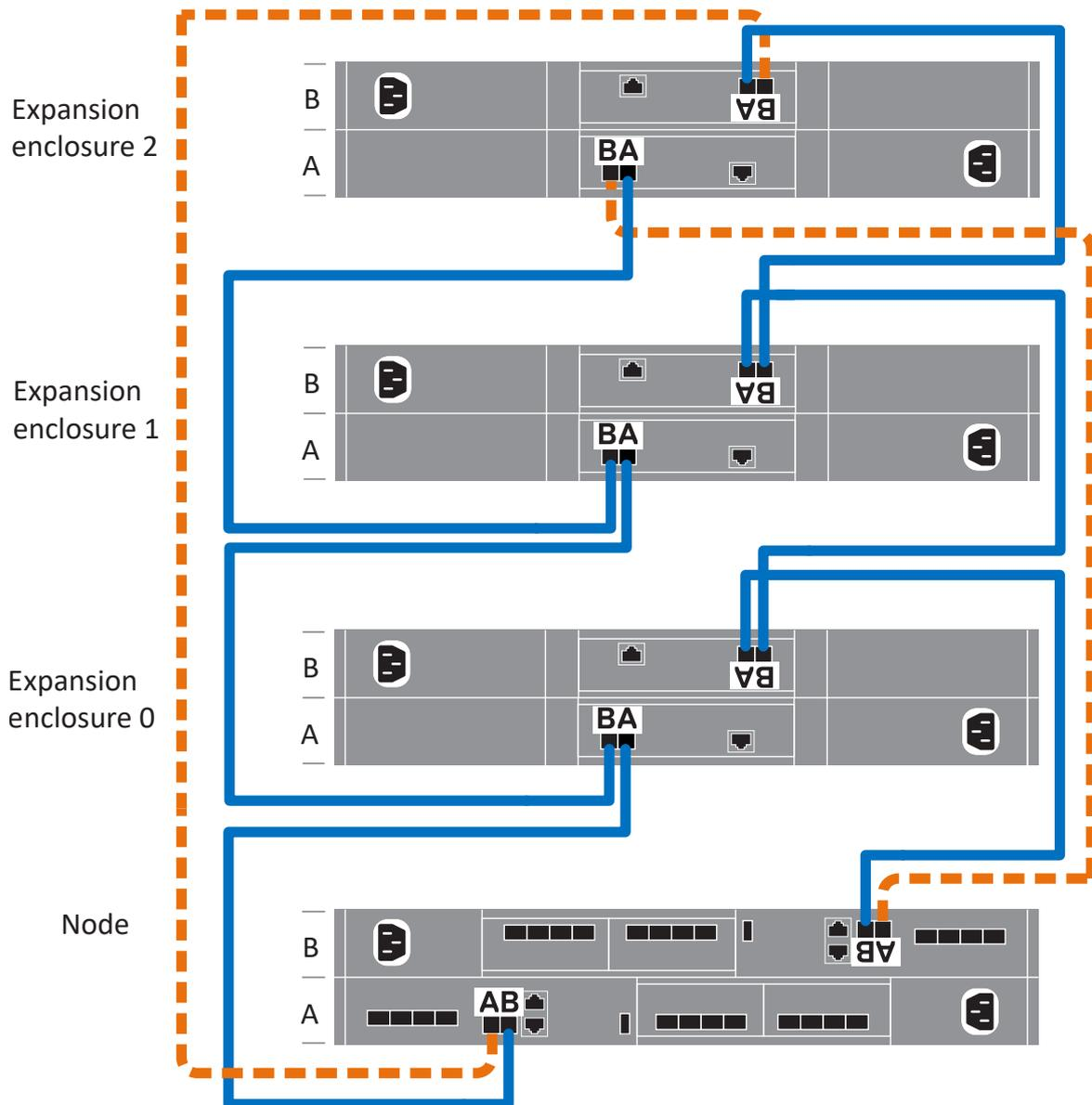
Figure 24. Cabling the base enclosure to three expansion enclosures
