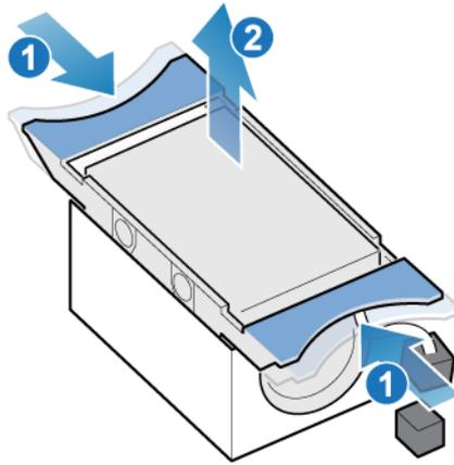
Figure 104. Removing the fan from the motherboard
