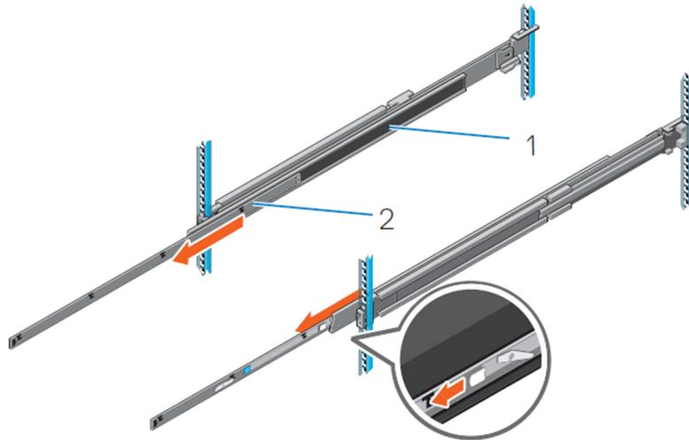
**Figure 42. Pull out the intermediate rail**
