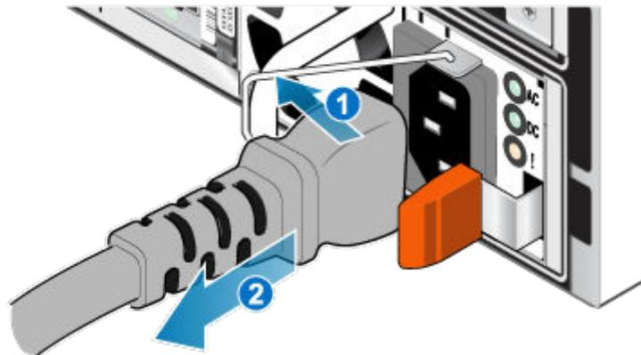
**Figure 214. Removing the power cable**
