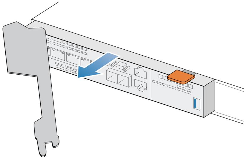
**Figure 255. Removing the embedded module from the system**
