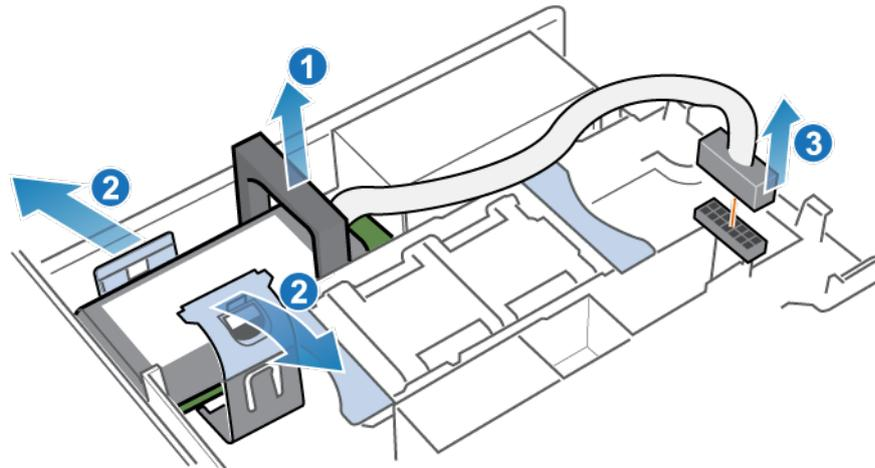
**Figure 273. Releasing the internal battery backup module**
