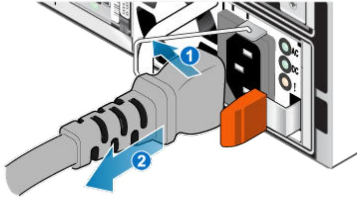
**Figure 98. Removing the power cable**
