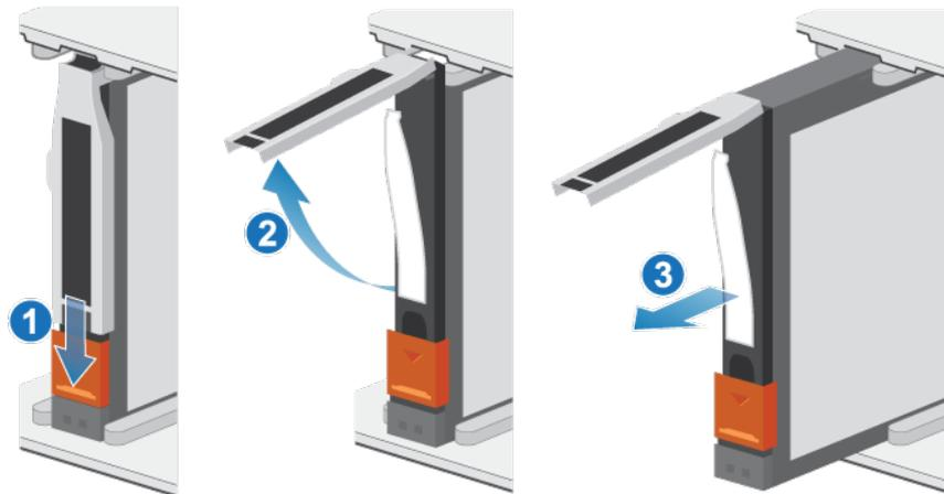
Figure 162. Removing a drive
