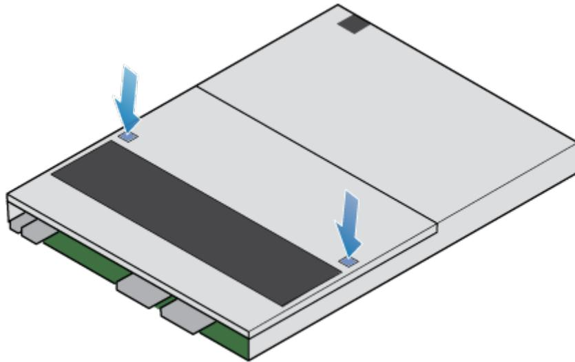
**Figure 113. Releasing the top cover**
