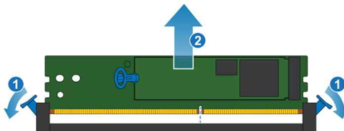
Figure 260. Removing the M.2 boot module adaptor
