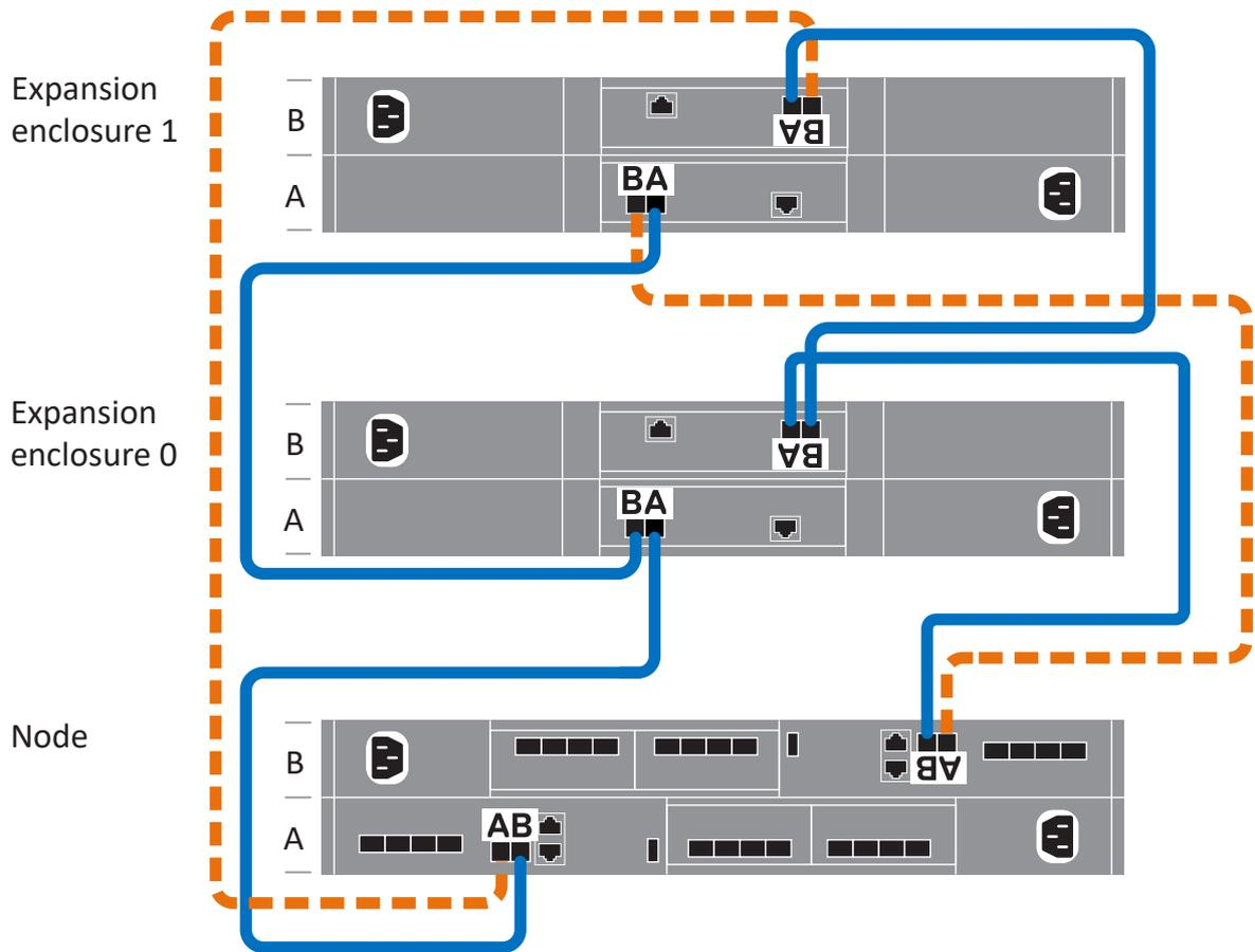
Figure 23. Cabling the base enclosure to two expansion enclosures
