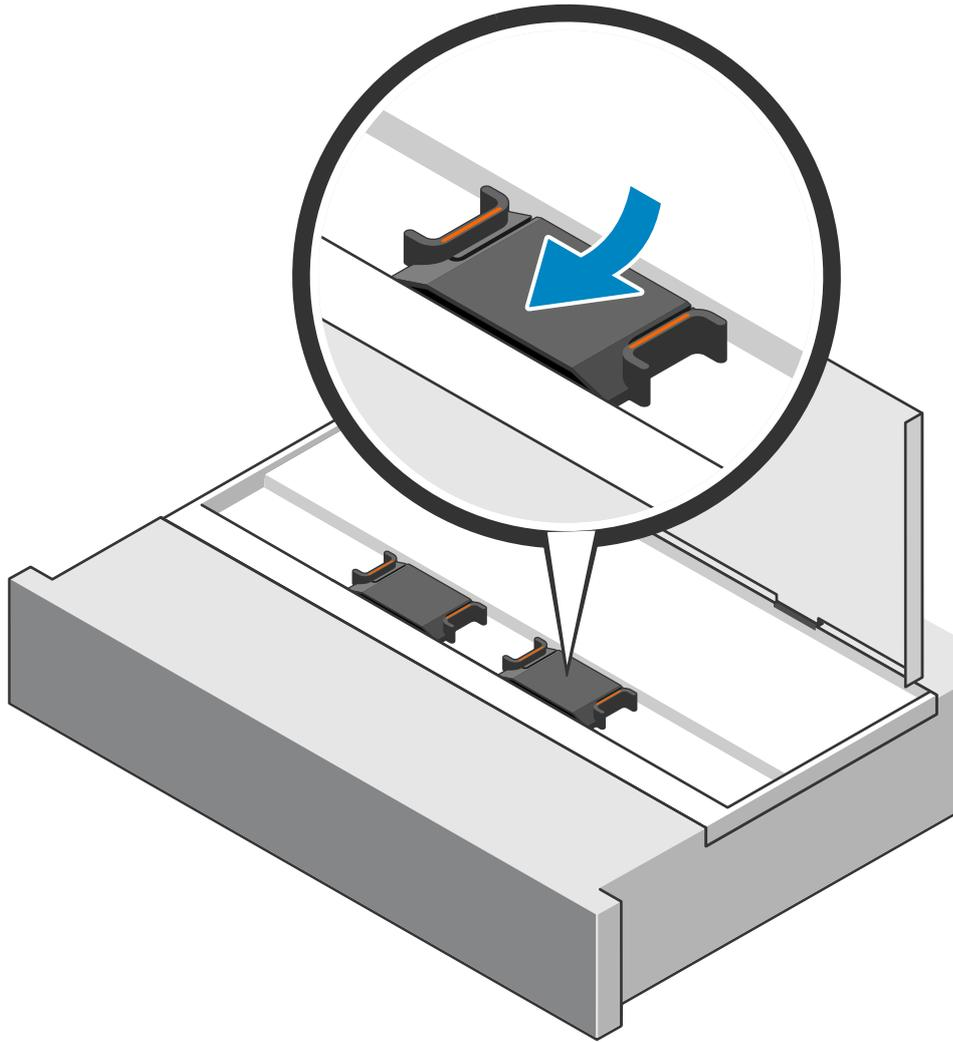
**Figure 195. Installing the Clock Distribution Board**
