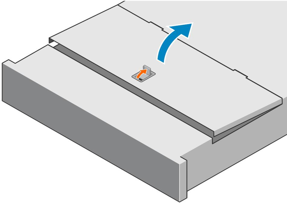
**Figure 189. Lifting the system cover**
