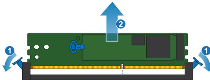
Figure 234. Removing the M.2 boot module adaptor
