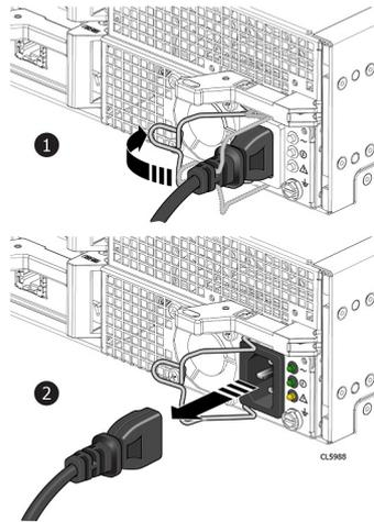
**Figure 171. Unplugging the power cord from an AC power supply/cooling module**
