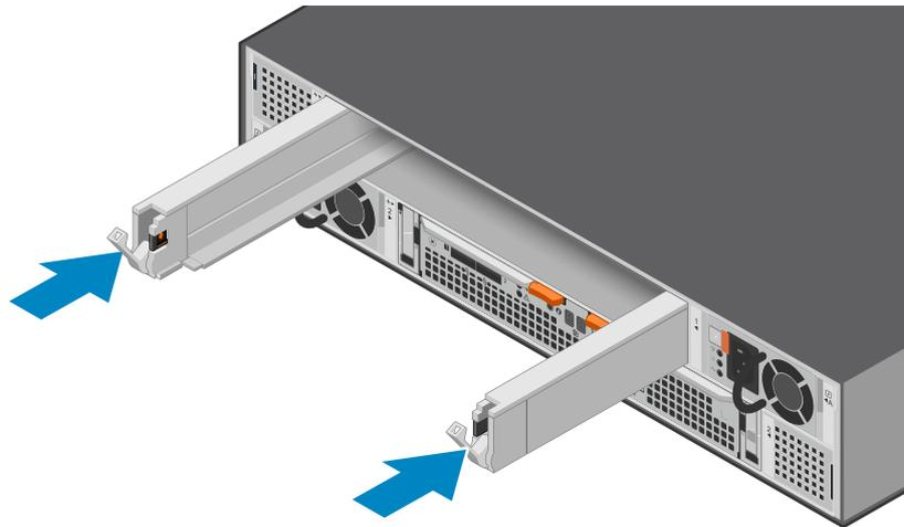
**Figure 203. Installing the DIB**
