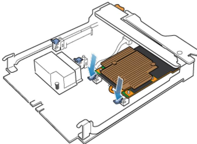
**Figure 76. Opening the retaining tabs**
