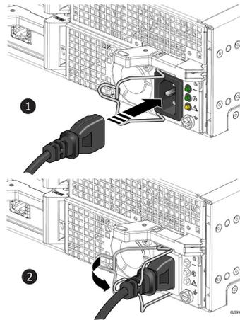
Figure 175. Plugging in the power cable
