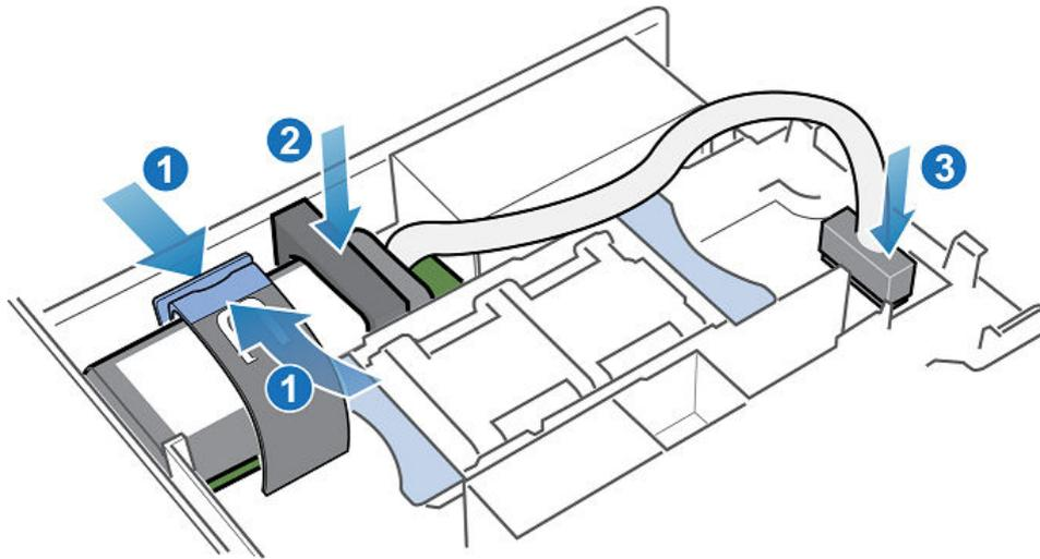
**Figure 276. Connecting the internal battery backup module cable to the motherboard**
