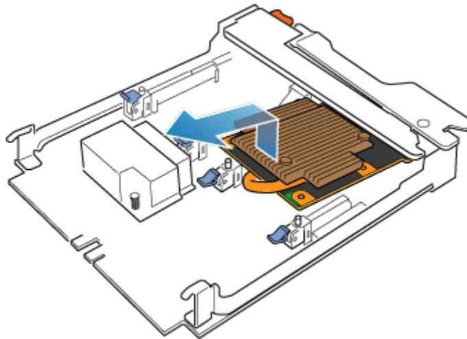
Figure 68. Removing the 4-port card
