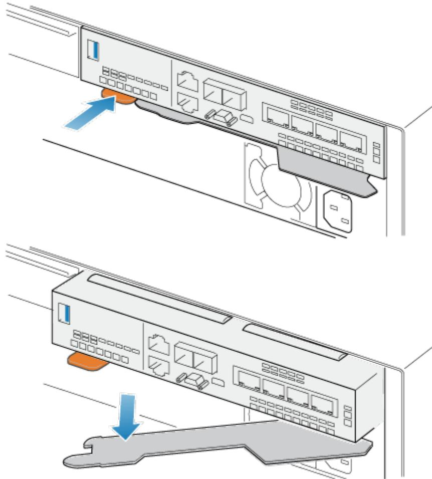
**Figure 65. Releasing the lever on the embedded module**
