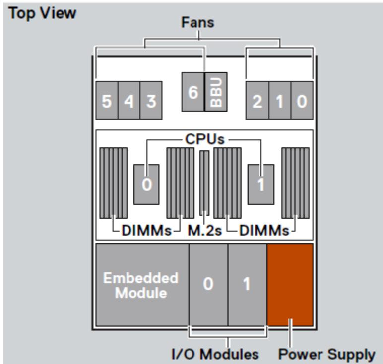
Figure 221. Top view of the node
