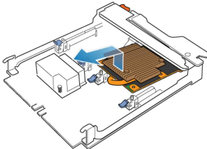
Figure 68. Removing the 4-port card
