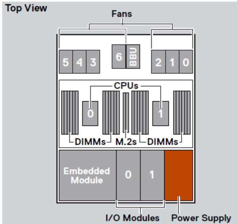
Figure 115. Top view of the node
