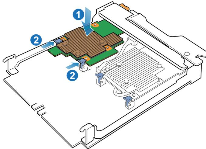
**Figure 88. Locking the 2-port 100GbE card into position**
