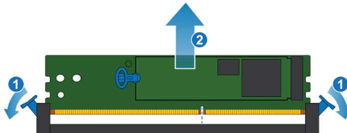
Figure 127. Removing the M.2 boot module adaptor
