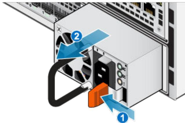
Figure 222. Removing a power supply
