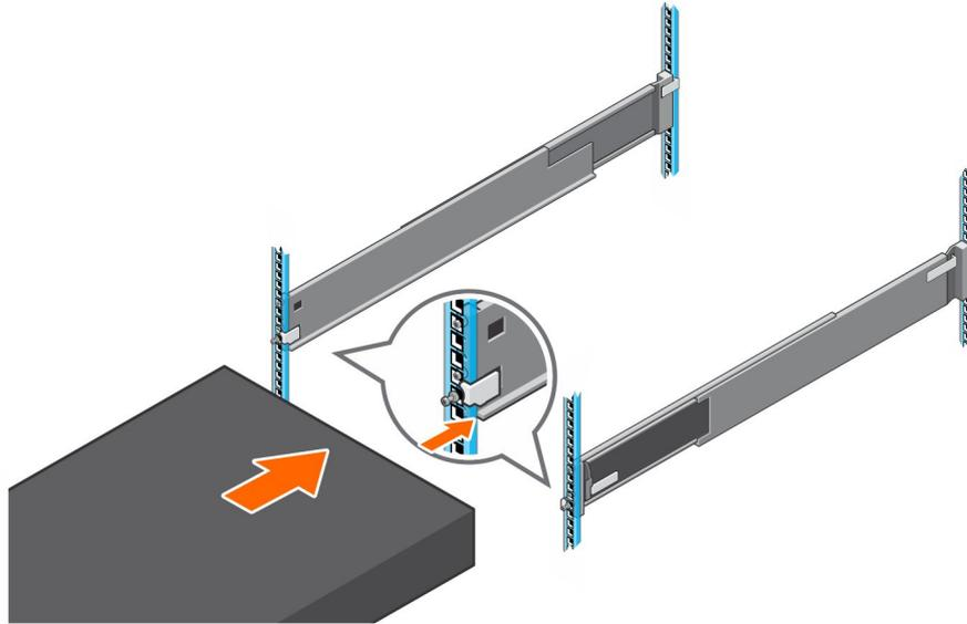
**Figure 19. Securing the system in the rack**
