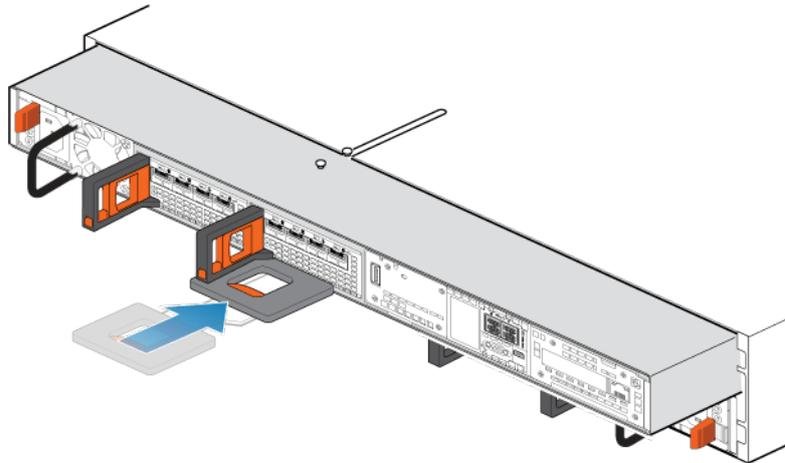
Figure 146. Sliding the node halfway into the chassis
