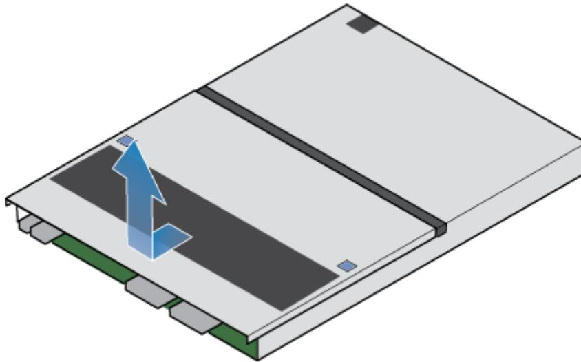
Figure 139. Removing the top cover
