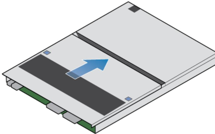
Figure 119. Securing the top cover
