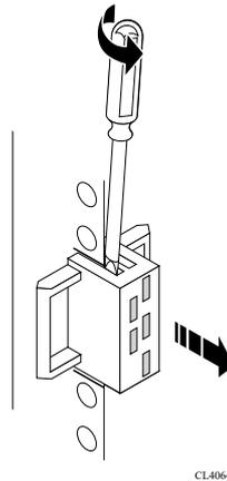
Figure 16. Prying off a latch bracket
