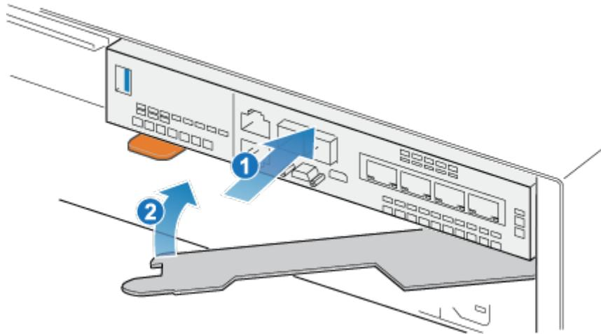
**Figure 89. Installing the embedded module**
