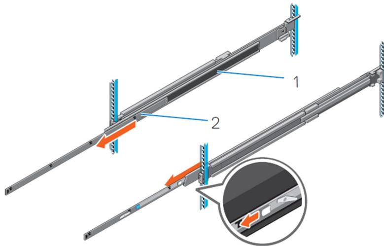
**Figure 28. Pull out the intermediate rail**
