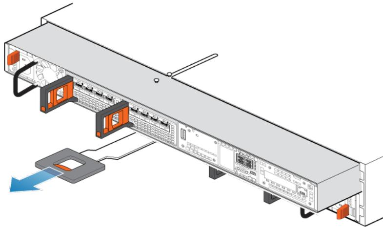
**Figure 112. Removing the node**
