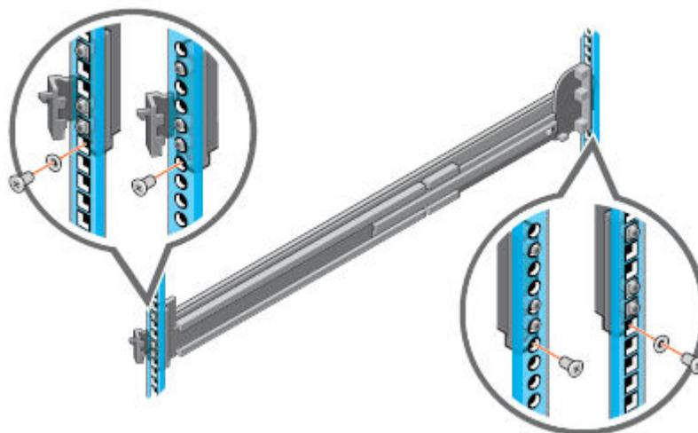
**Figure 27. Adding the retaining screws**
