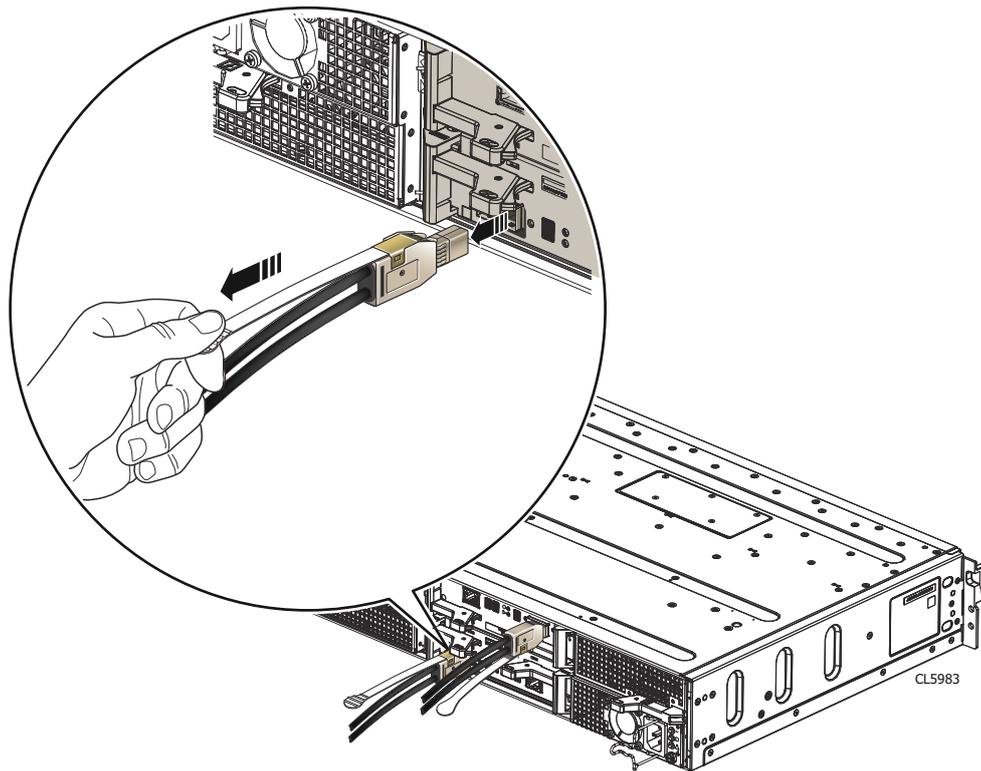
**Figure 166. Disconnecting an LCC cable**
