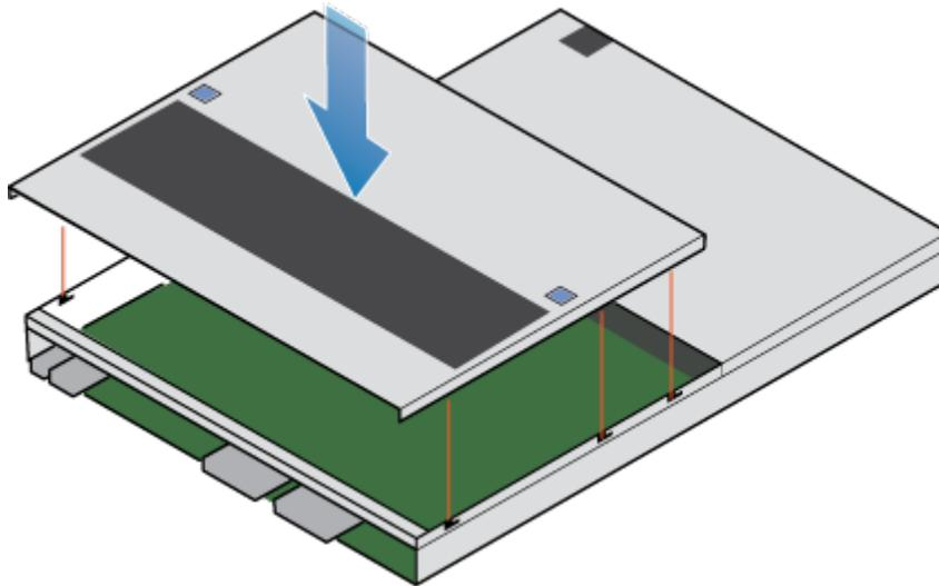
Figure 241. Aligning the top cover
