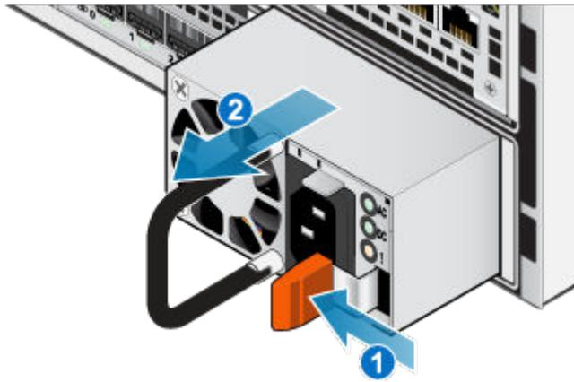
Figure 215. Removing the power supply
