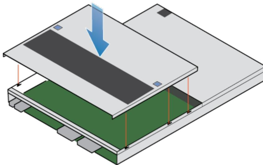
Figure 144. Aligning the top cover
