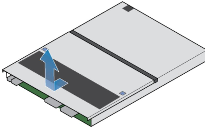
Figure 126. Removing the top cover
