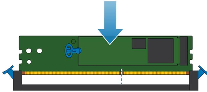
Figure 143. Installing the M.2 boot module adaptor
