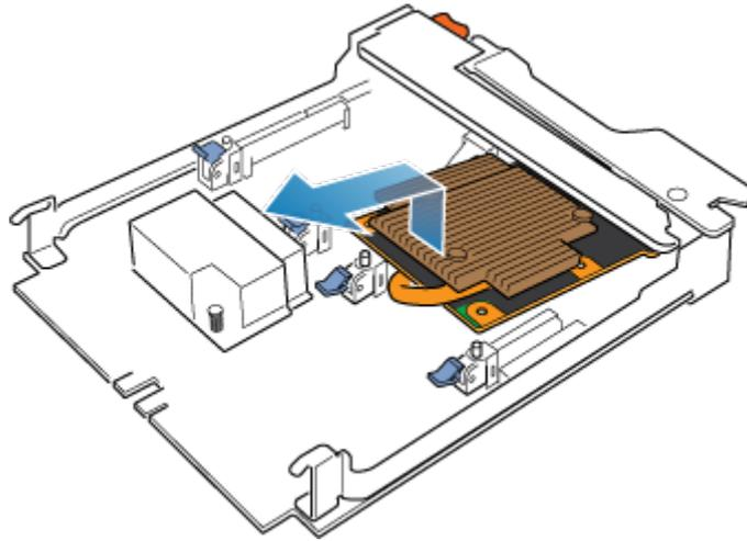
Figure 77. Removing the 4-port card
