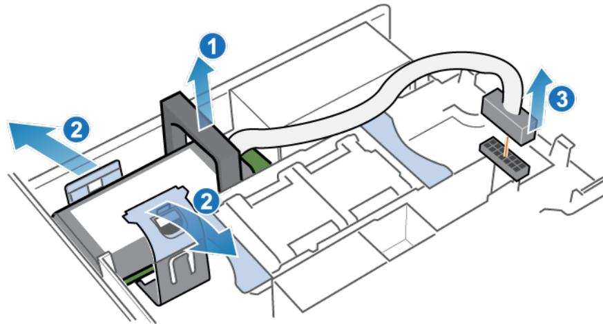
**Figure 263. Releasing the internal battery backup module**
