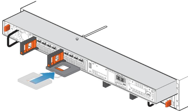
**Figure 243. Sliding the node halfway into the chassis**
