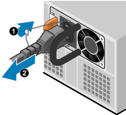
Figure 185. Removing the power cable
