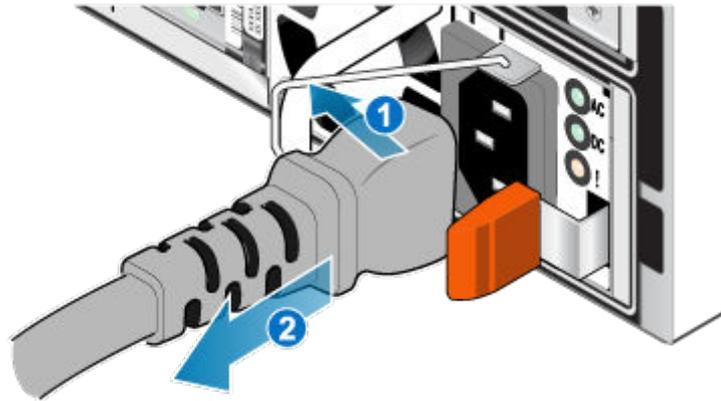
**Figure 135. Removing the power cable**
