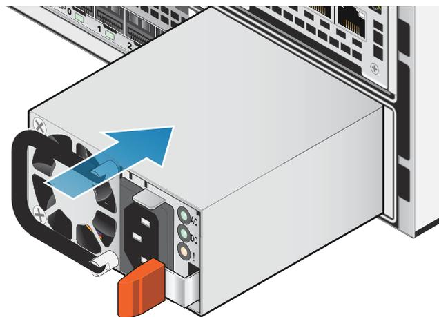
Figure 216. Installing a power supply
