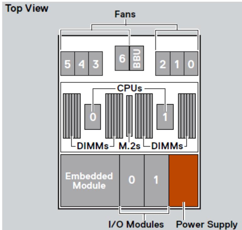
Figure 221. Top view of the node
