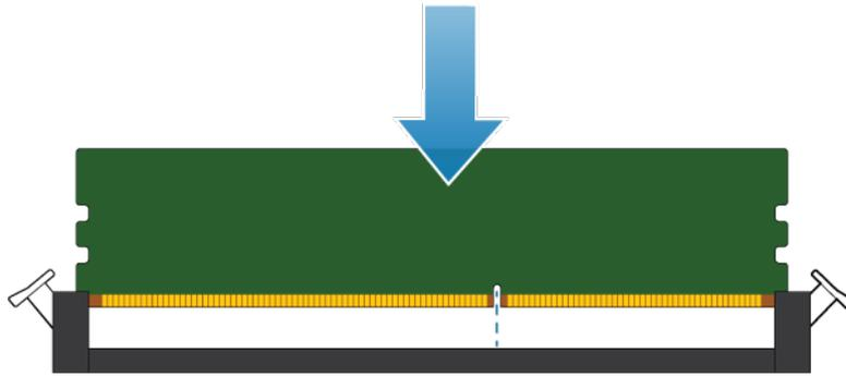
**Figure 117. Installing the DIMM**
