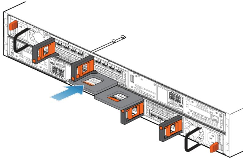
**Figure 134. Installing the node**
