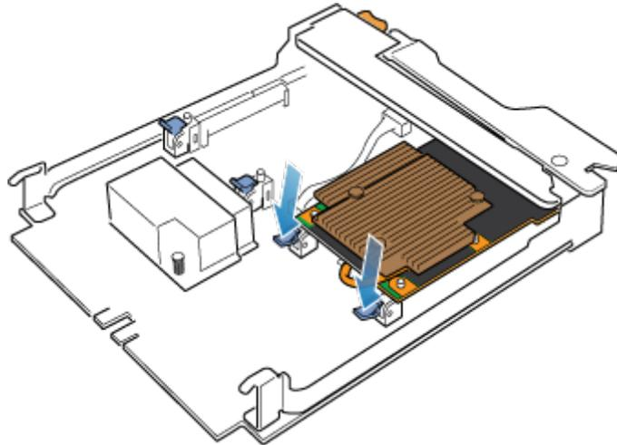
Figure 67. Opening the retaining tabs
