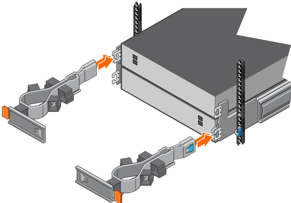
**Figure 32. Installing the cable management arms**
