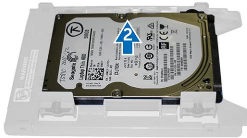
7. If a 3.5–inch hard drive is installed, flex the hard-drive bracket on both sides to loosen the hard drive.
