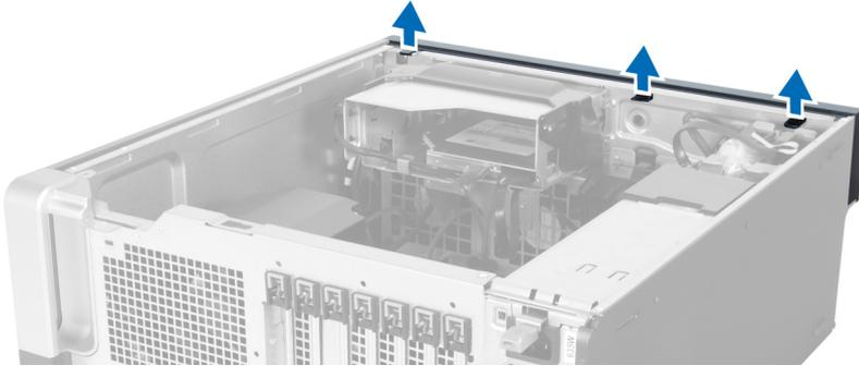
4. Rotate and pull the bezel panel away from the computer to release the hooks on the opposite edge of the bezel from the chassis.
