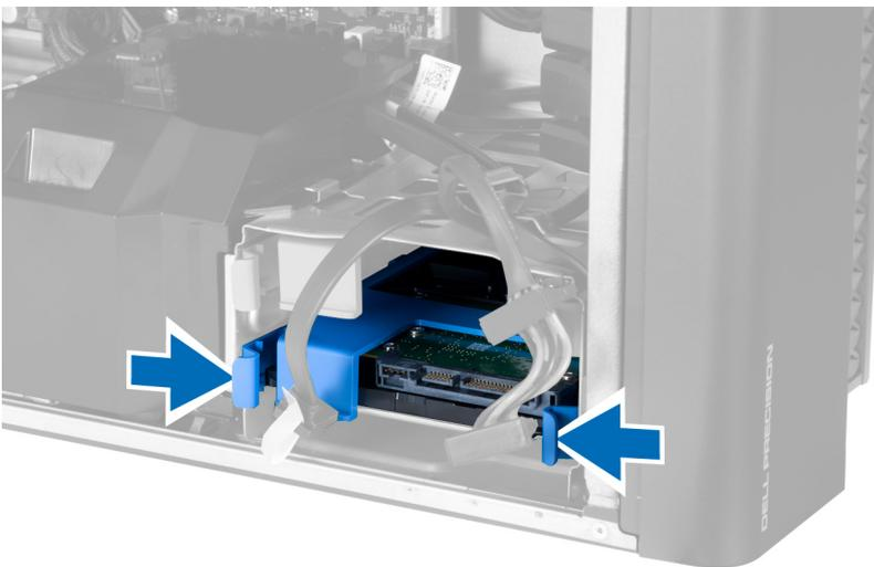
5. Slide the hard drive out of the compartment.
