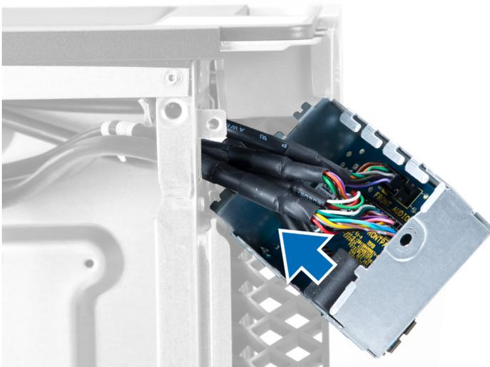
5. Disconnect the cables to release the I/O panel to remove it from the computer.
