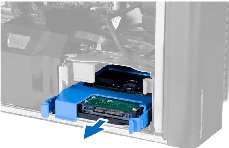
6. If a 2.5-inch hard drive is installed, flex the hard-drive bracket on both sides to loosen the hard drive and lift it to remove it from the hard-drive bracket [1, 2].
