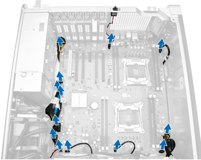
4. Remove the screws that secure the system board to the chassis.
