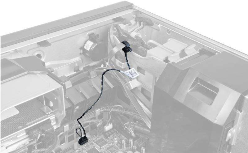
4. Disconnect the HDD thermal sensor cable from the system board.
