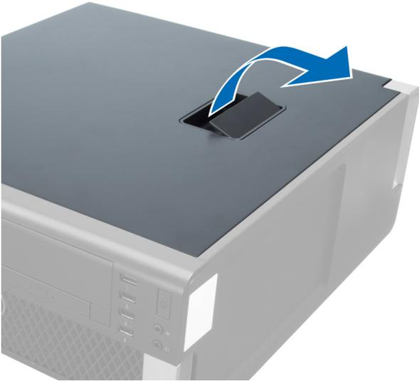
3. Lift the cover upward to a 45-degree angle, and remove it from the computer.
