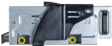
10. Remove the screws that secure the optical drive to the optical-drive cage.
