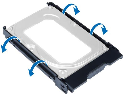
8. Lift the hard drive in an upward direction to remove it from the hard-drive bracket.
