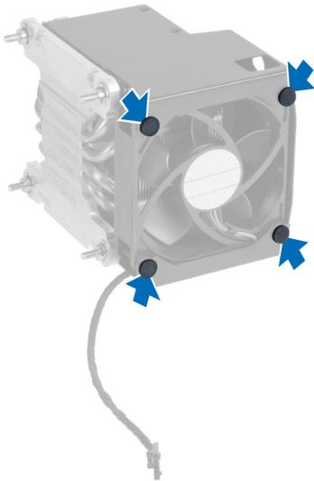
4. Slide the heatsink fan from the heatsink assembly.
