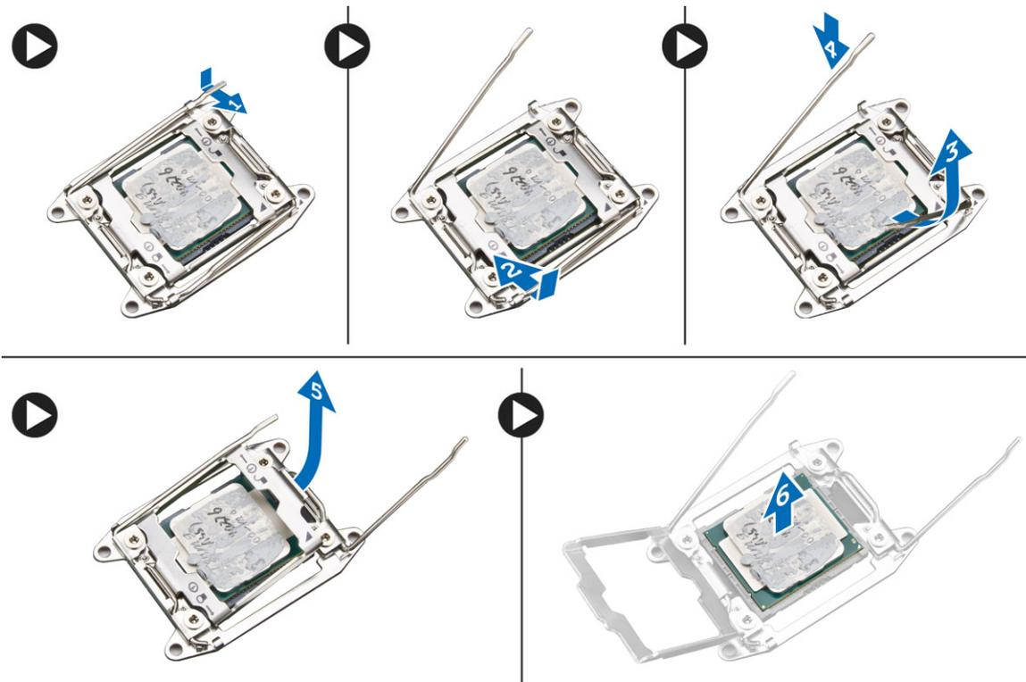
**NOTE:** Damaging pins during removal of the processor can cause damage to the processor.
