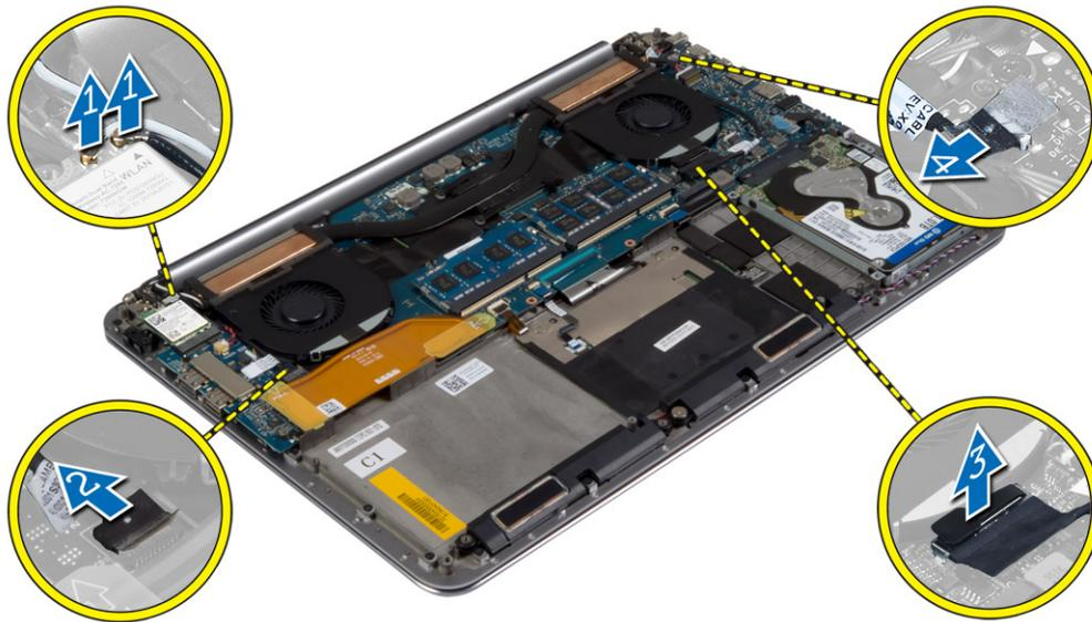
4. Remove the screws that secure the display hinges to the palmrest assembly.
