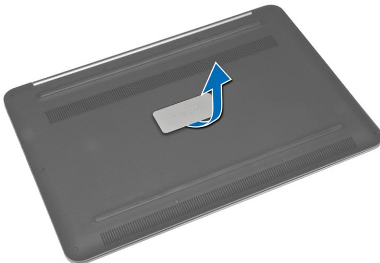
4. Remove the screws that secure the base cover to the computer. Release and remove the base cover from the computer.
