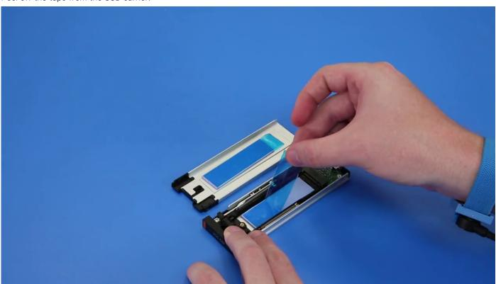
$\boldsymbol{c.}\,$  Peel off the adhesive tape from the SSD carrier cover.
