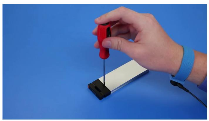
$\boldsymbol{c.}$  Slide the SSD cover from the top of the carrier.
