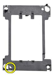
3. Flip both the processor and the carrier over so that the pins on the processor and the logo side of the carrier are facing up.
