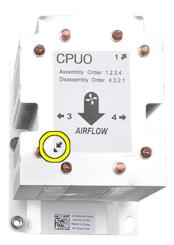
**6.** Insert the processor and carrier assembly into the heat sink so that the hooks on the four corners of the carrier are locked into the openings of heat sink.
