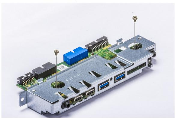
**b.** Release and remove the I/O panel out of the bracket.
