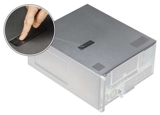
4. Pull the latch [1] upward and rotate it to release the cover [2].
