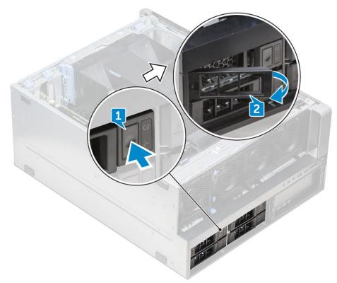
**b.** Pull the latch to slide the carrier out of the HDD slot.
