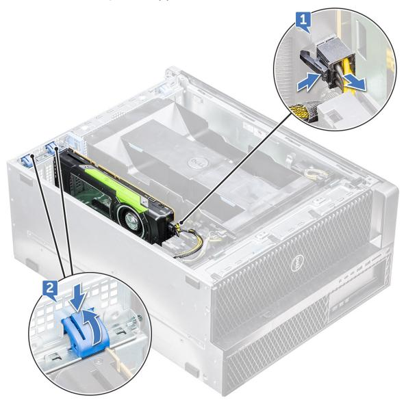
c. Lift the GPU from the PCle slot on the system board.
