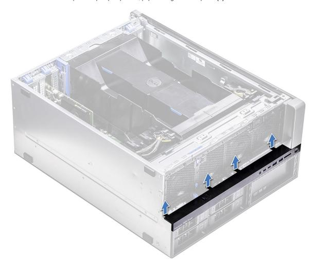
4. Slightly slide the panel, and lift it away from the chassis.
