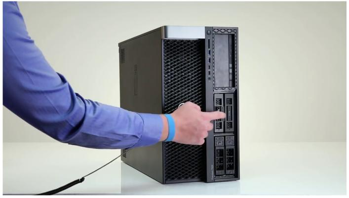
$\mbox{\bf b.}\;\;\mbox{Pull the M.2 SSD}$  carrier out of the NVMe flexbay.
