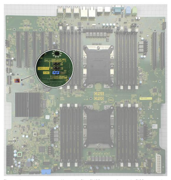
Plugging the power management cable into the Clear CMOS jumper will cause the BIOS to reset when sending a remote restart request to the Teradici card. You will then have to reset the time and BIOS settings.
