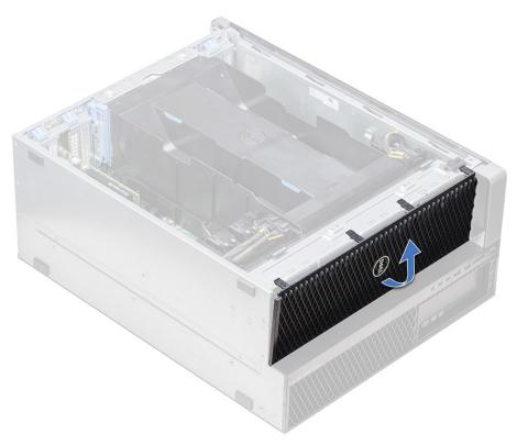
**b.** Rotate the bezel forward and lift the front bezel away from the system.
