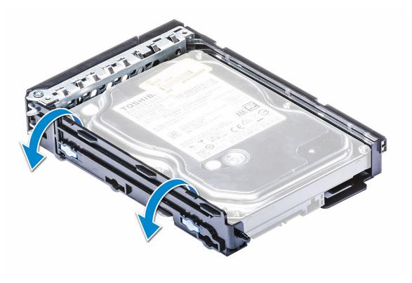
**b.** Lift the hard drive out of the carrier.
