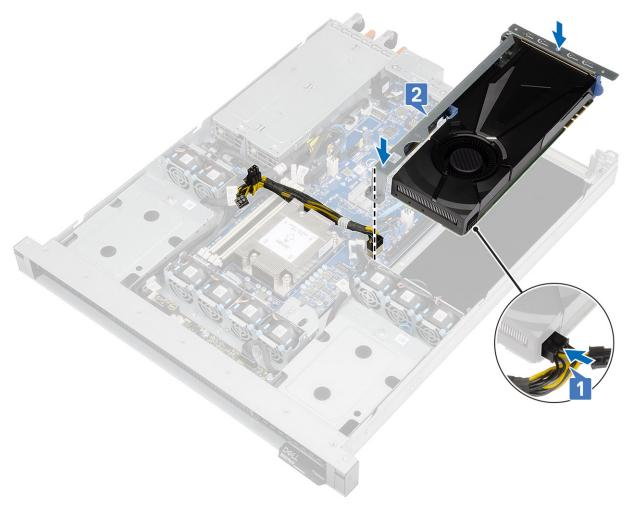
7. Route the GPU power cable through the retention clips on the graphics card fan cage.
