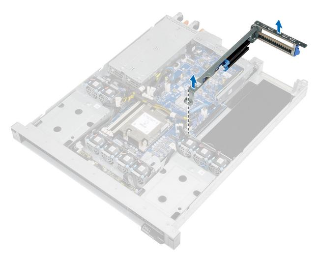
$\textbf{5.} \ \ \text{Pull the release tab [1] to open the riser1 slot and lift the riser blanks [2] from the slot.}$
