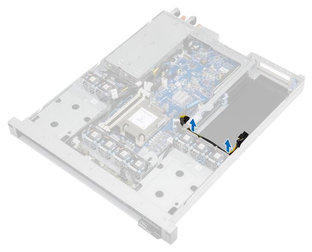
$\textbf{4.} \quad \text{Holding the blue contact points remove the riser1 module from the slot.}$
