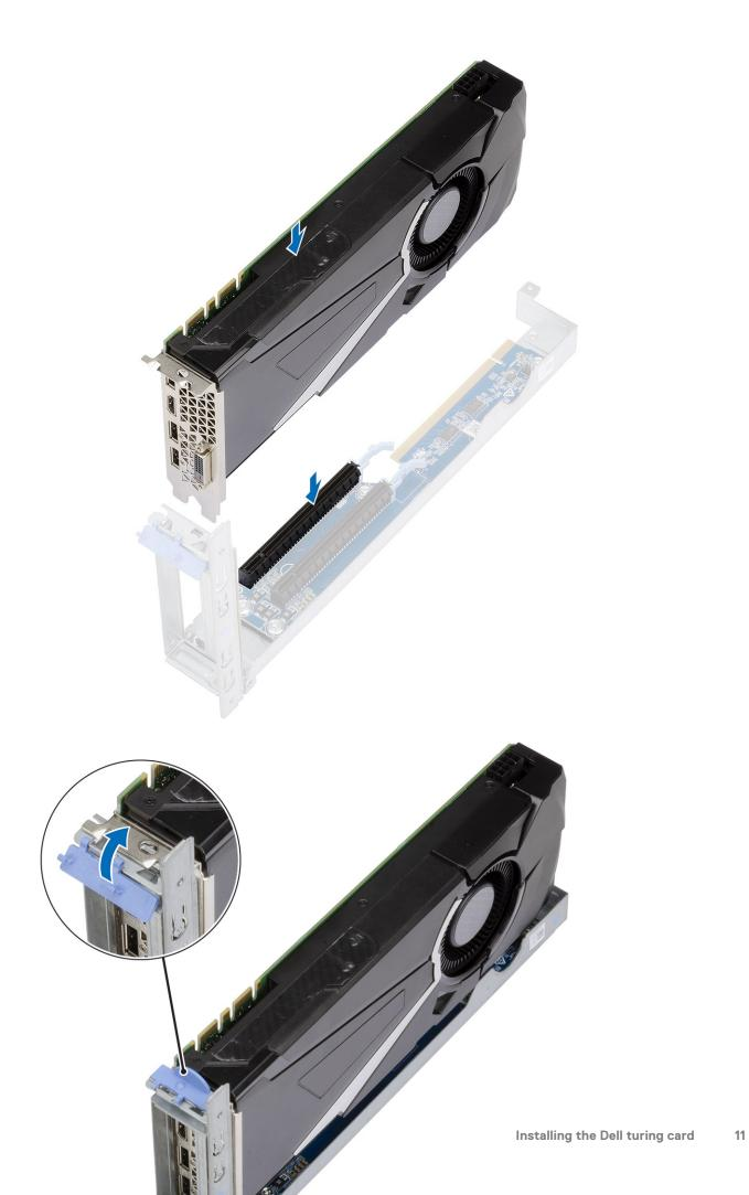
c) Connect the power cable to the turing card module [1]. Align the riser1 module with the alignment pins on the chassis and insert the riser1 module into the slot [2].
