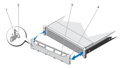
Figure 7. Removing and Installing the Front Bezel
