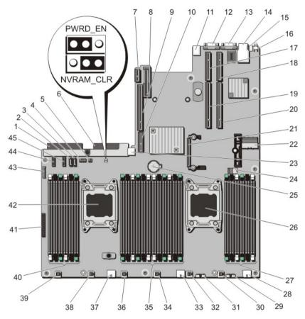
Figure 51. System Board Jumpers and Connectors
