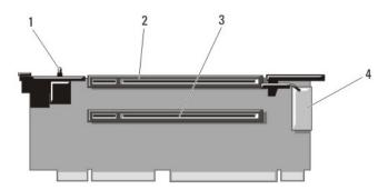
Figure 27. Identifying Connectors on the Expansion Card Riser 2
