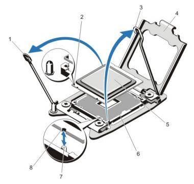
Figure 37. Removing and Installing a Processor
