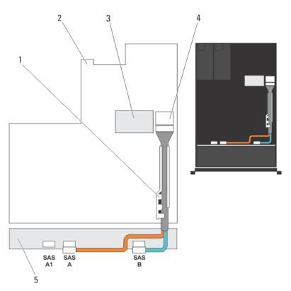
Figure 45. Cabling Diagram—3.5 linch (x12) SAS/SATA Backplane
