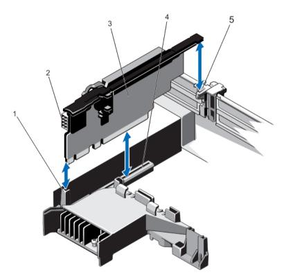
Figure 28. Removing and Installing the Expansion Card Riser 3
