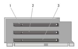
Figure 25. Identifying Connectors on the Expansion Card Riser 1
