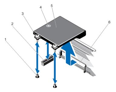
Figure 34. Removing and Installing the Network Daughter Card
