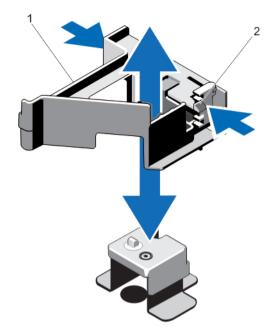
Figure 19. Removing and Installing the PCIe Card Holder
