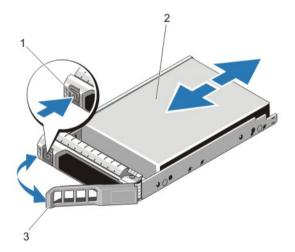
Figure 15. Removing and Installing a Hot-Swap Hard Drive
