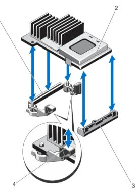
Figure 33. Removing and Installing the Integrated Storage Controller Card
