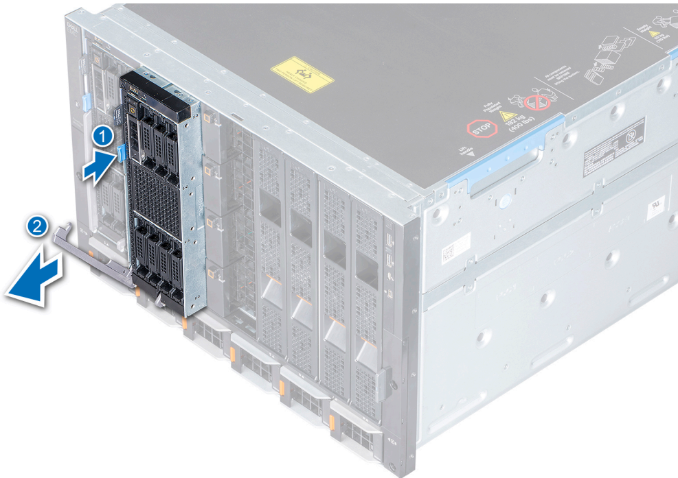
Figure 13. Removing the sled from the enclosure
