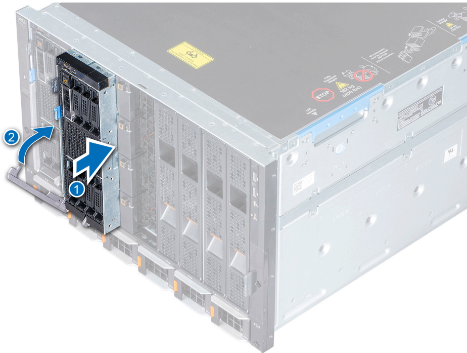
Figure 16. Installing the sled into the enclosure
