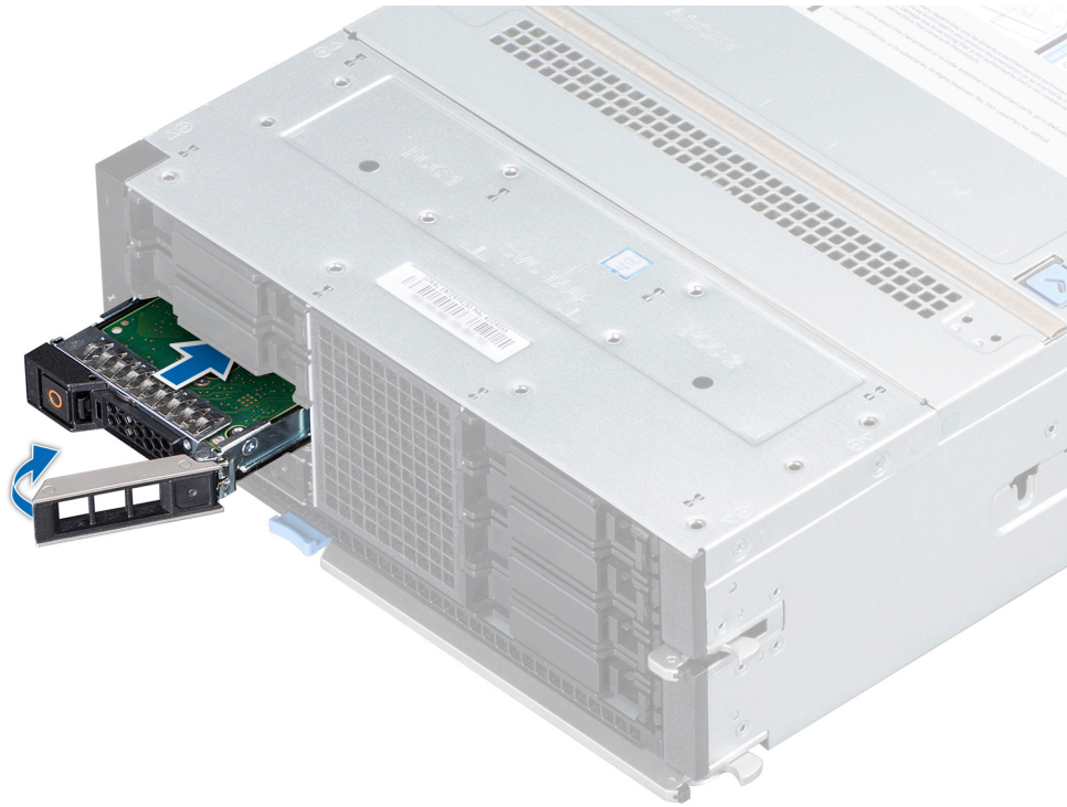
Figure 28. Installing a drive carrier
