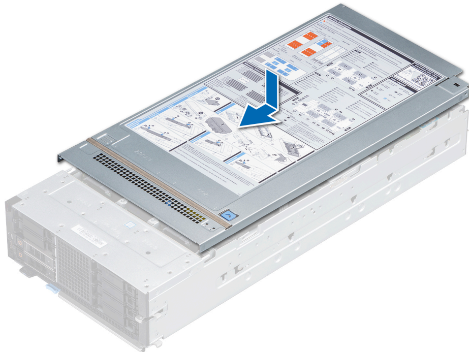
Figure 18. Installing the sled cover
