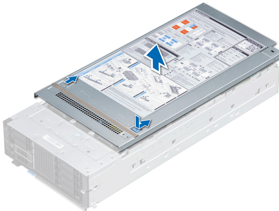
Figure 17. Removing the sled cover
