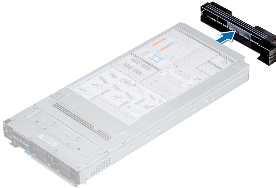
Figure 14. Removing the I/O connector cover from sled
