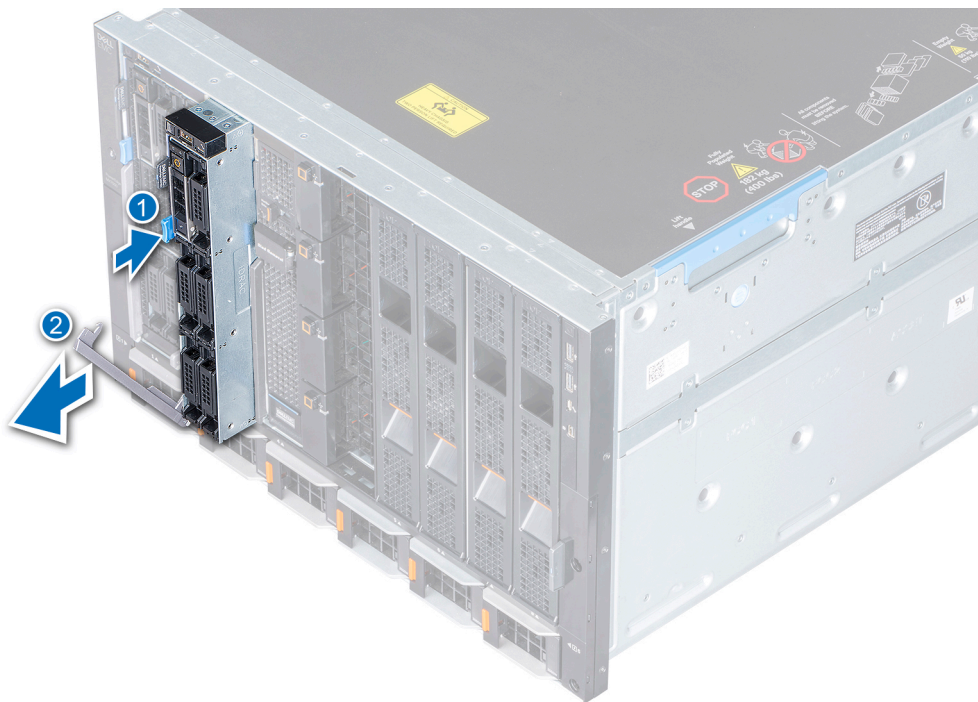
Figure 12. Removing the sled from enclosure
