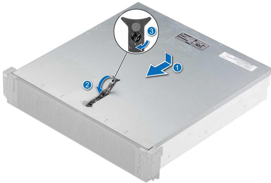
Figure 29. Installing the system cover for Rear Accessed configuration
