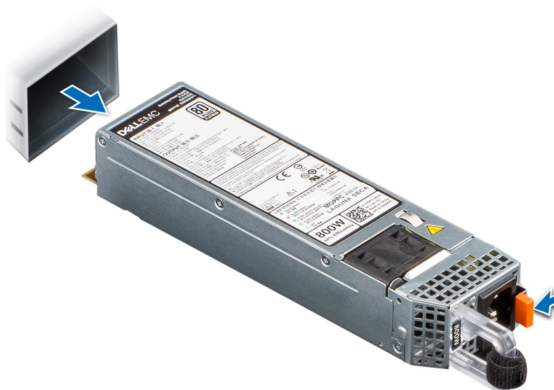
Figure 133. Removing a power supply unit
