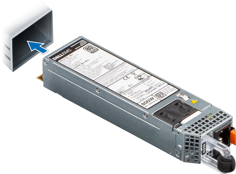
Figure 134. Installing a power supply unit
