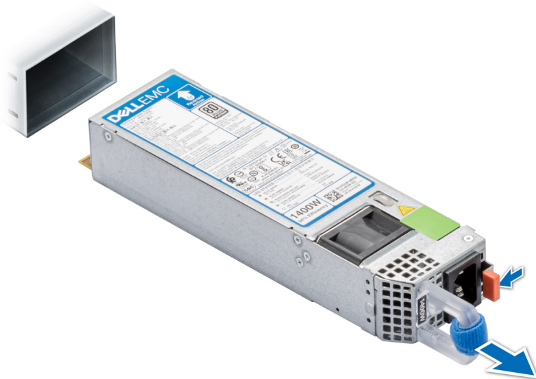
Figure 100. Removing a power supply unit from Front Accessed configuration
