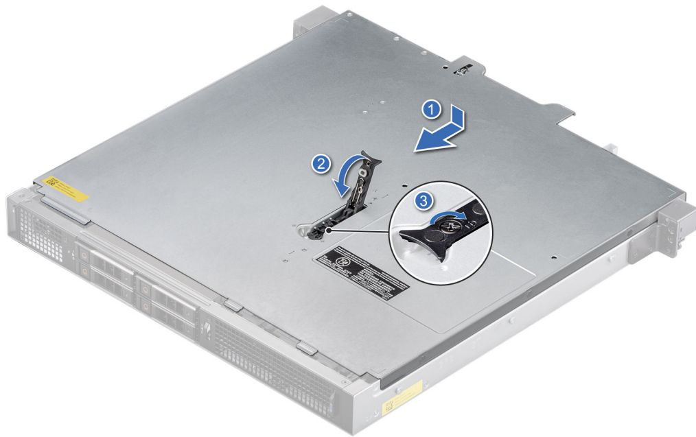
Figure 22. Installing the system cover for Front Accessed configuration
