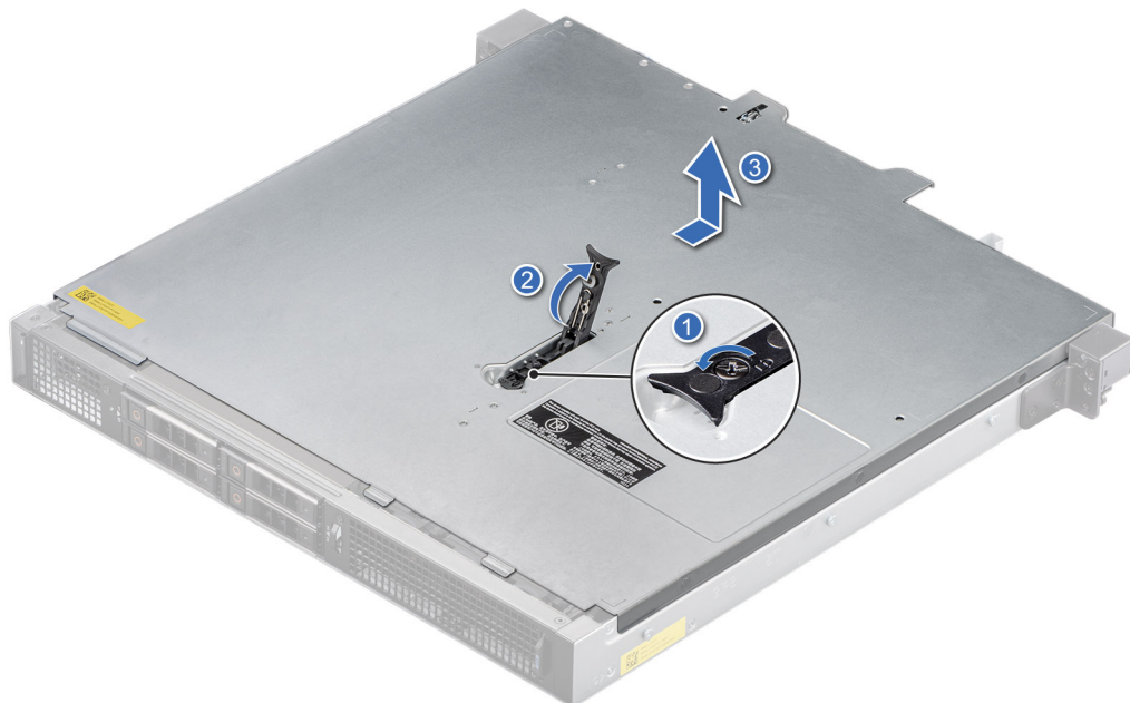
Figure 20. Removing the system cover for Front Accessed configuration
