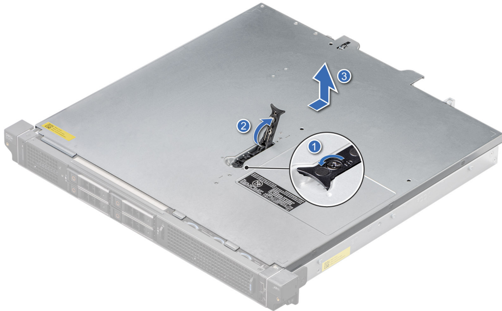
Figure 19. Removing the system cover for Rear Accessed configuration
