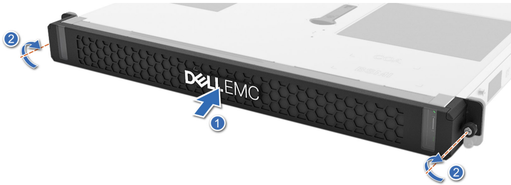
Figure 16. Installing the front bezel for Rear Accessed configuration
