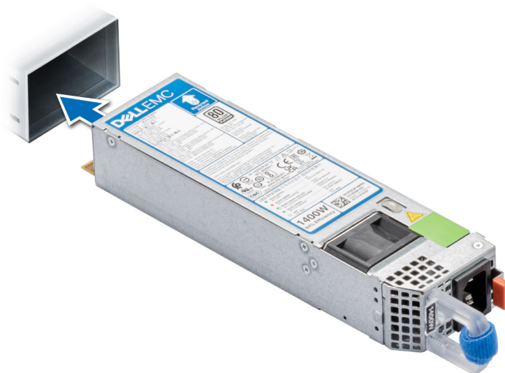
Figure 102. Installing a power supply unit for Front Accessed configuration
