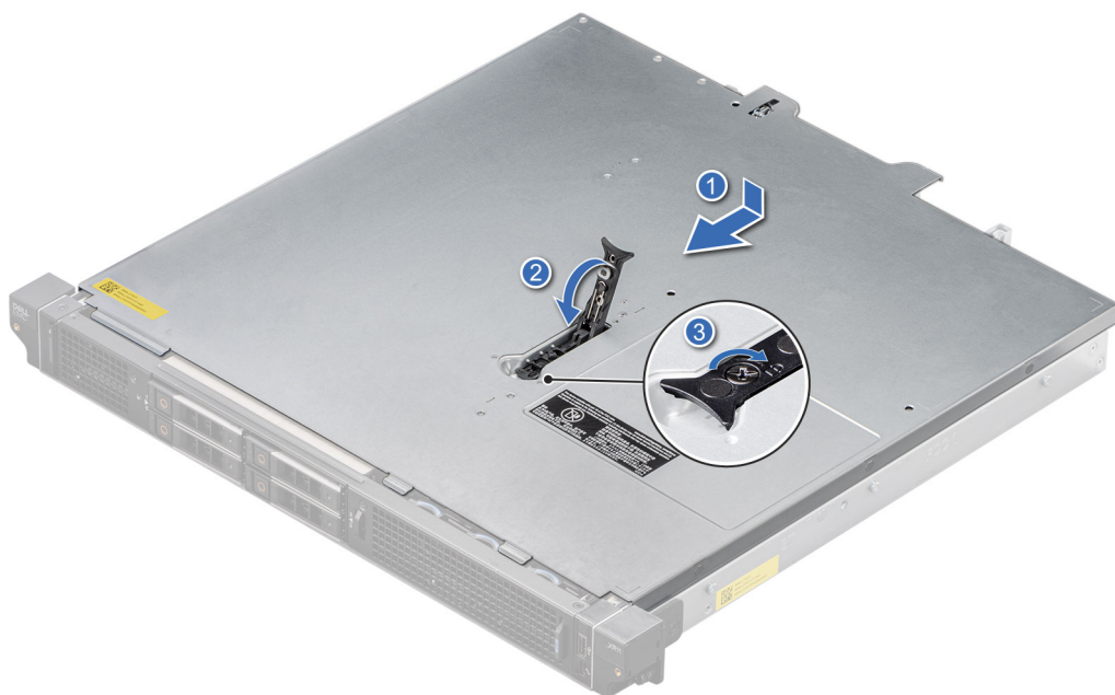
Figure 21. Installing the system cover for Rear Accessed configuration
