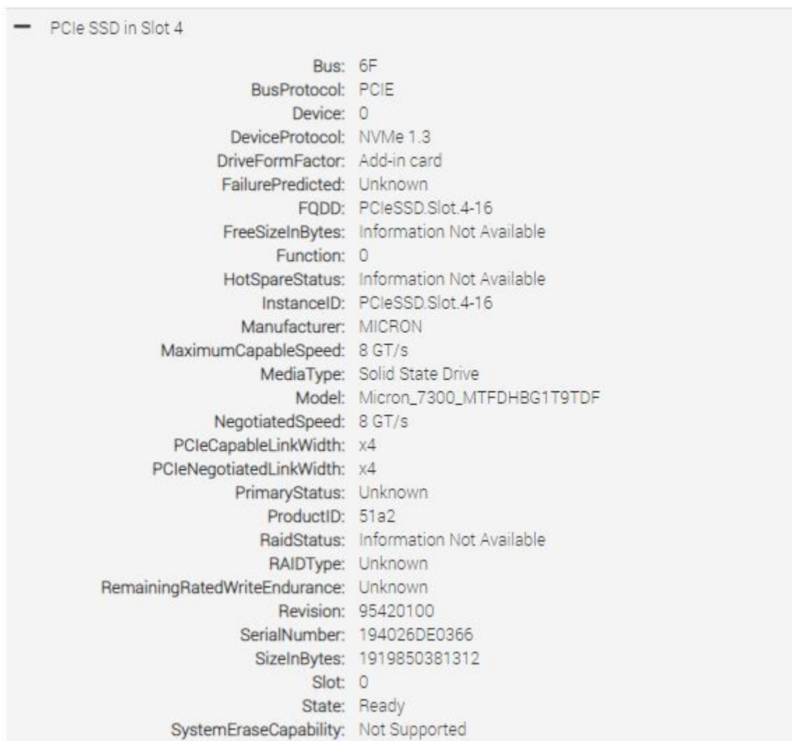
Figure 15. Adapter for NVMe M.2, PCIe storage options in iDRAC inventory
