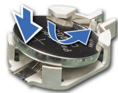
Figure 109. System battery installation
