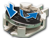
Figure 61. System battery installation
