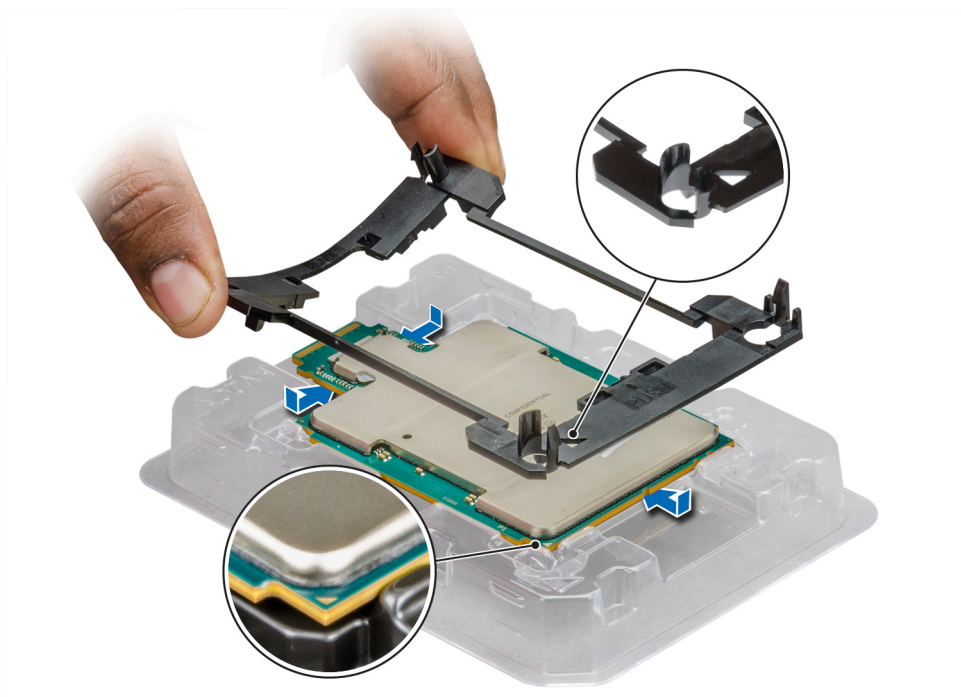
Figure 56. Installing the processor bracket
