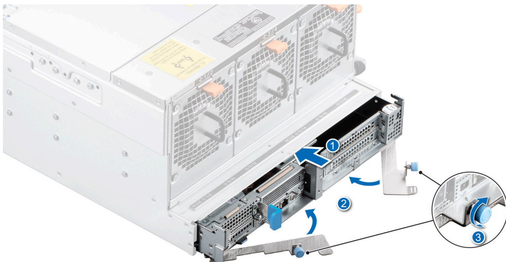
Figure 20. Installing the sled
