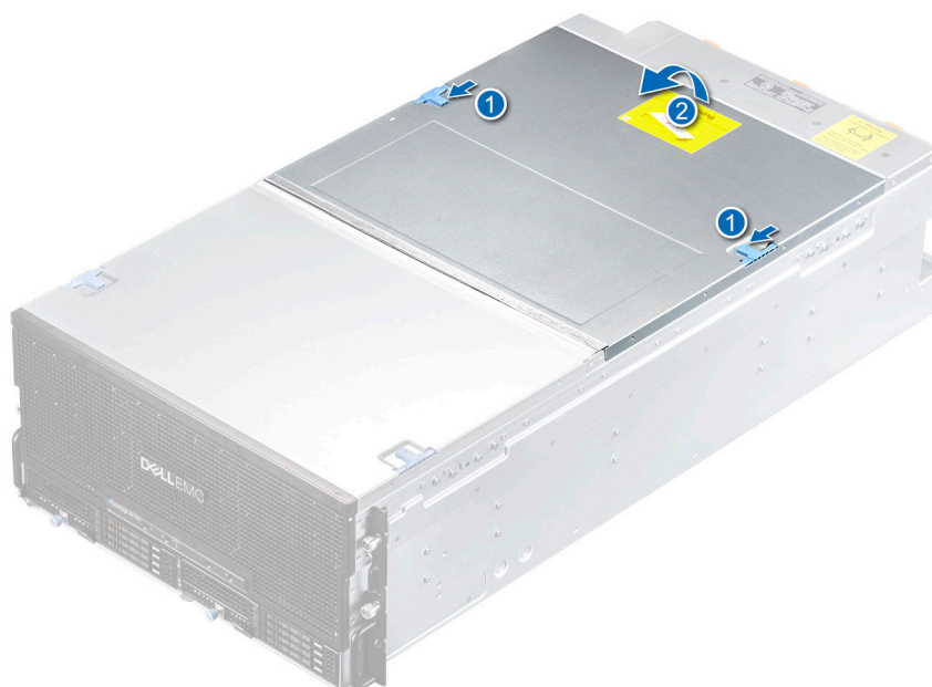
Figure 39. Removing the rear system cover
