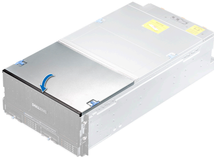
Figure 38. Front system cover installation
