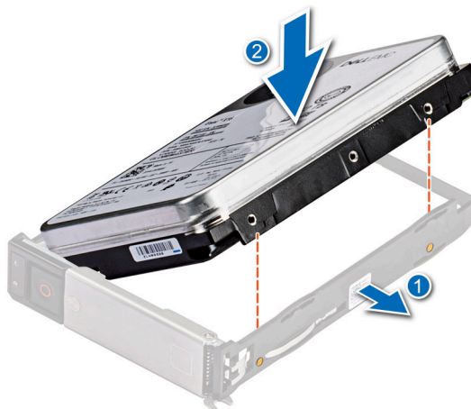
Figure 49. Installing a 3.5-inch drive into the drive carrier
