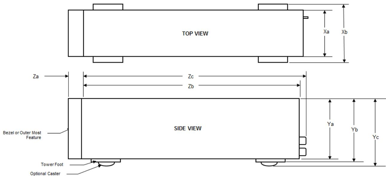
Figure 1. Dimensions of the Dell EMC PowerEdge T640 system
