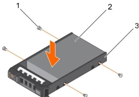
**图 45: 将热插拔硬盘驱动器安装到热插拔硬盘驱动器托盘中**
