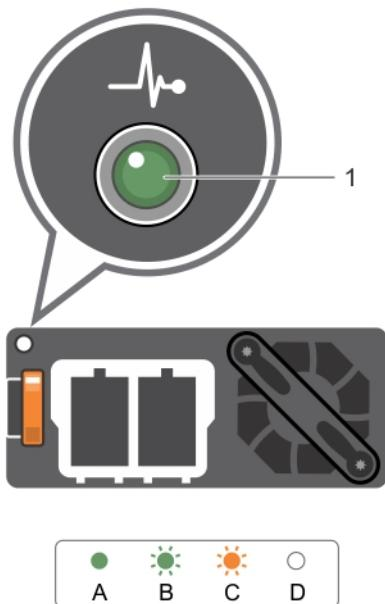
**图 8: DC PSU 状态指示灯**
