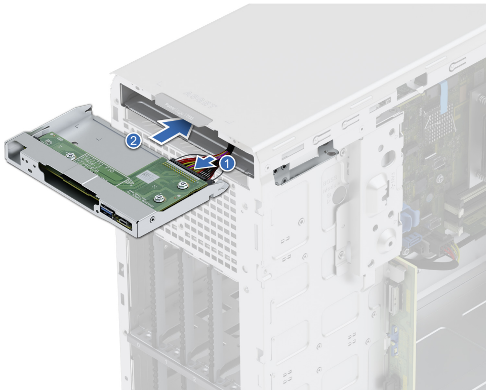
Figure 100. Installing the control panel cage
