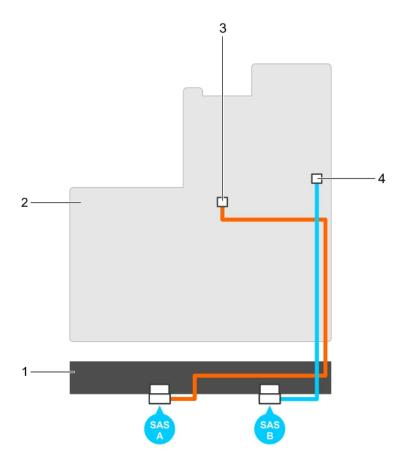
Figure 1. Cabling the S130 controller
