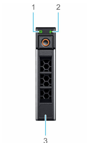
Figure 12. Drive indicators on the drive and the mid drive tray backplane
