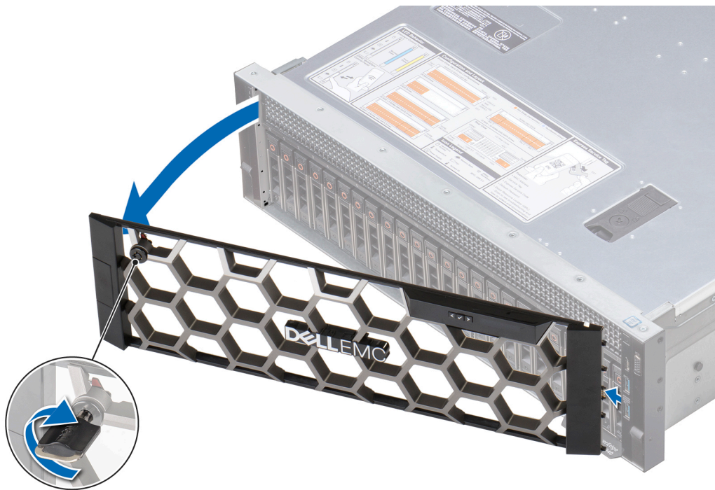
Figure 21. Removing the optional front bezel with the LCD panel
