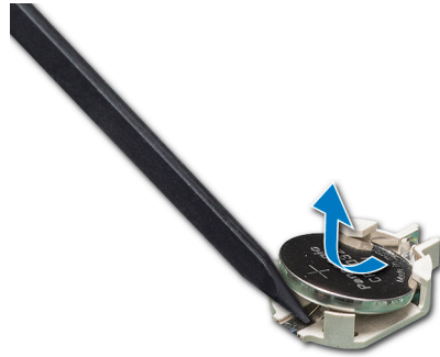
Figure 101. Removing the system battery
