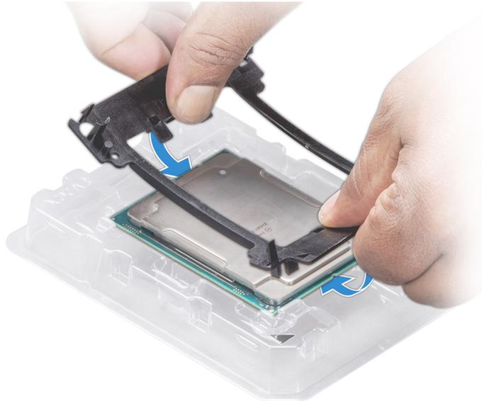
**Figure 70. Installing the processor bracket**
