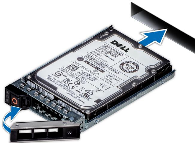
**Figure 38. Installing a drive carrier**
