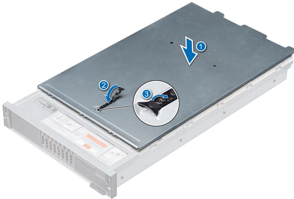
**Figure 20. Installing system cover**
