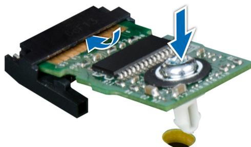
Figure 112. Installing the TPM
