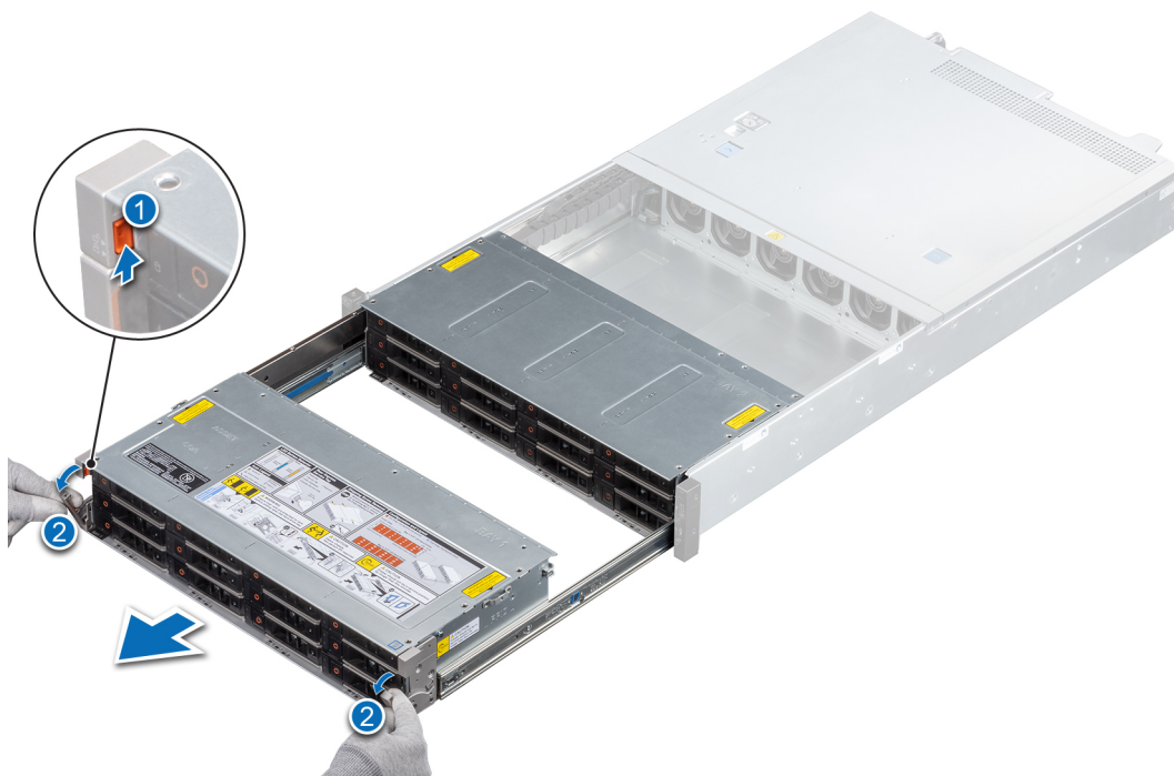
Figure 39. Opening the drive bays
