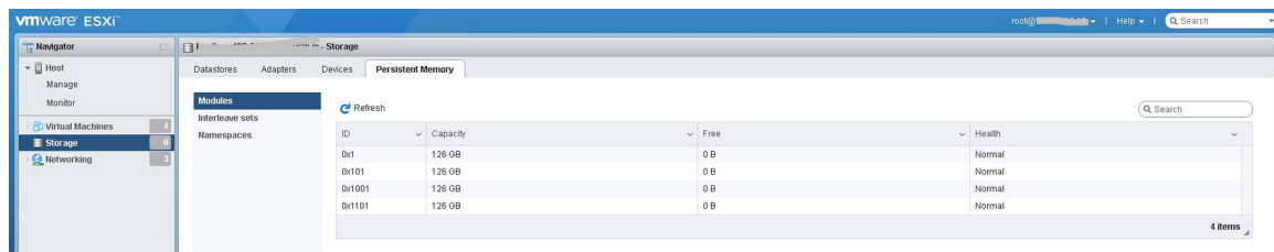
Figure 24. Persistent Memory modules populated in the system
