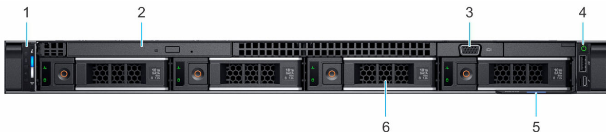
Figure 1. Front view of 4 x 3.5-inch drive system
