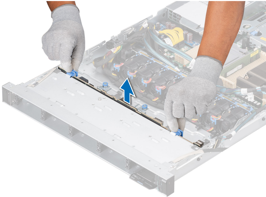
Figure 35. Removing the backplane
