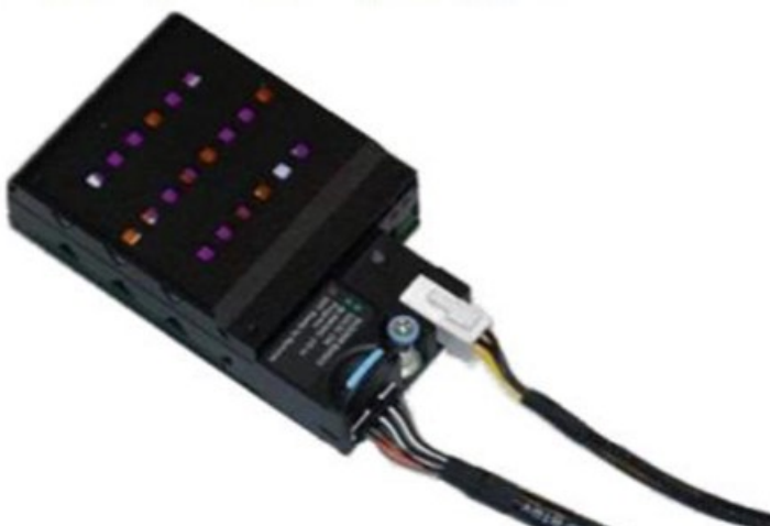
Figure 150. Connect power and signal cables to NVDIMM battery
