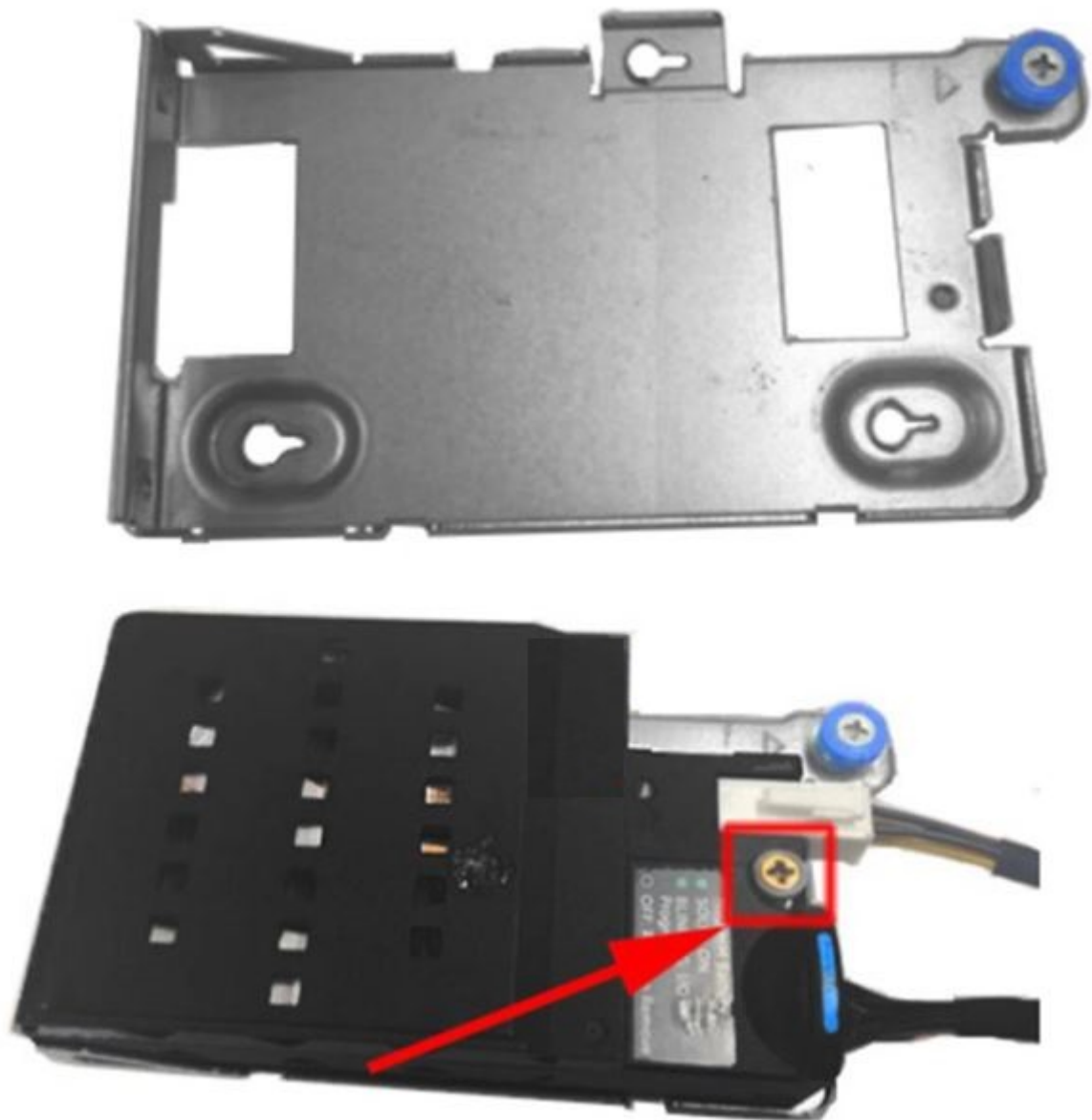
图 151: Installing battery on the battery tray
