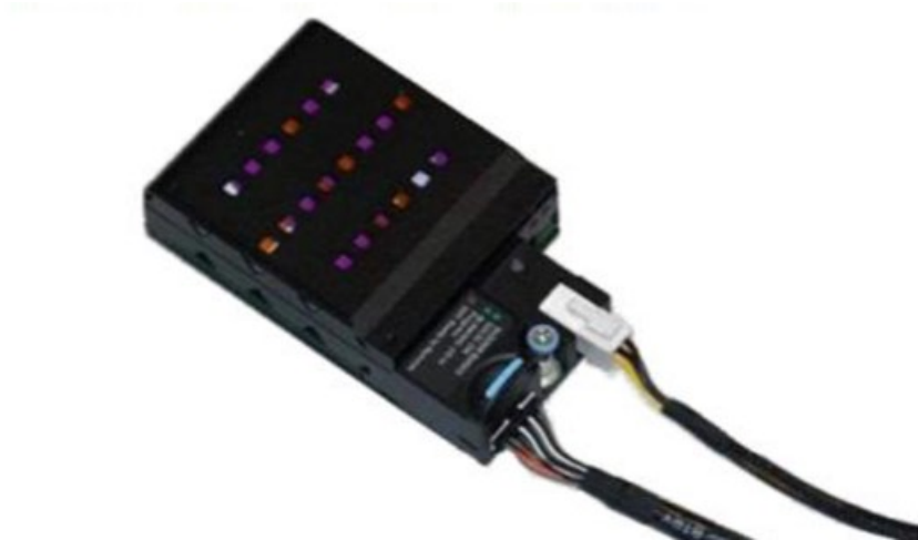
图 150: Connect power and signal cables to NVDIMM battery
