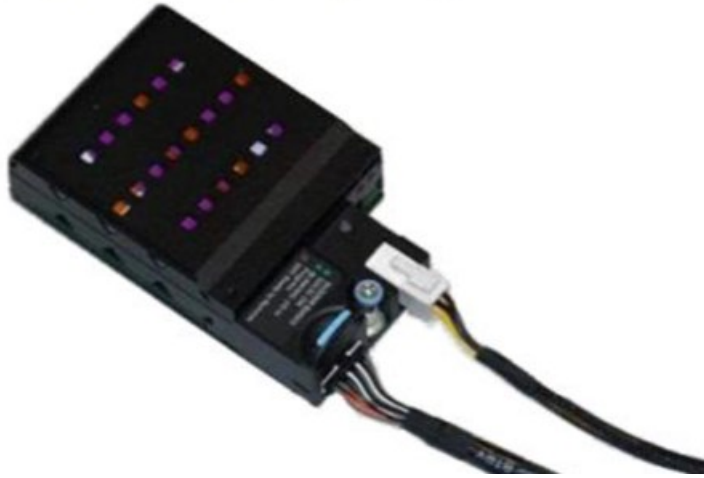
Rakam 150. Connect power and signal cables to NVDIMM battery
