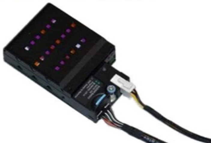
図 150. Connect power and signal cables to NVDIMM battery
