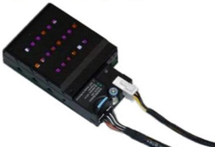
Ilustración 150. Connect power and signal cables to NVDIMM battery
