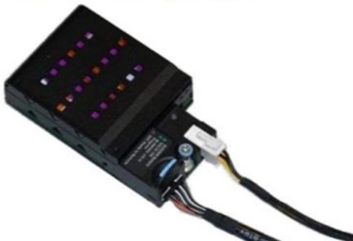
Abbildung 150. Connect power and signal cables to NVDIMM battery
