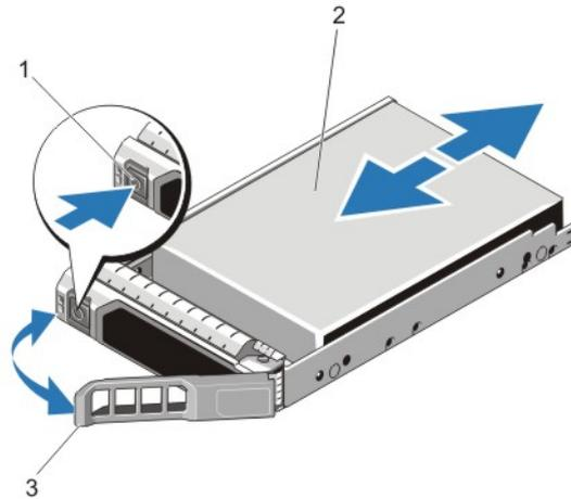
**Figure 23. Removing and Installing a Hot-Swap Hard Drive**
