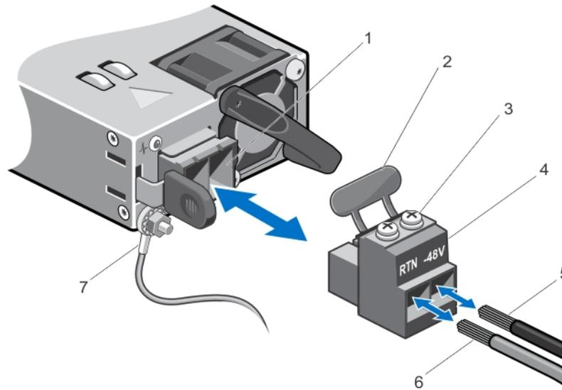
**Figure 42. Assembling the DC Input Power Wires**
