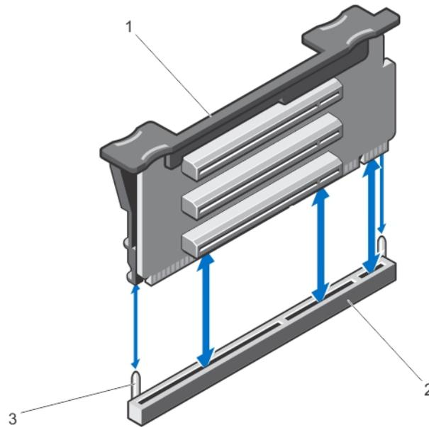
**Figure 33. Removing and Installing the Expansion-Card Riser 2**
