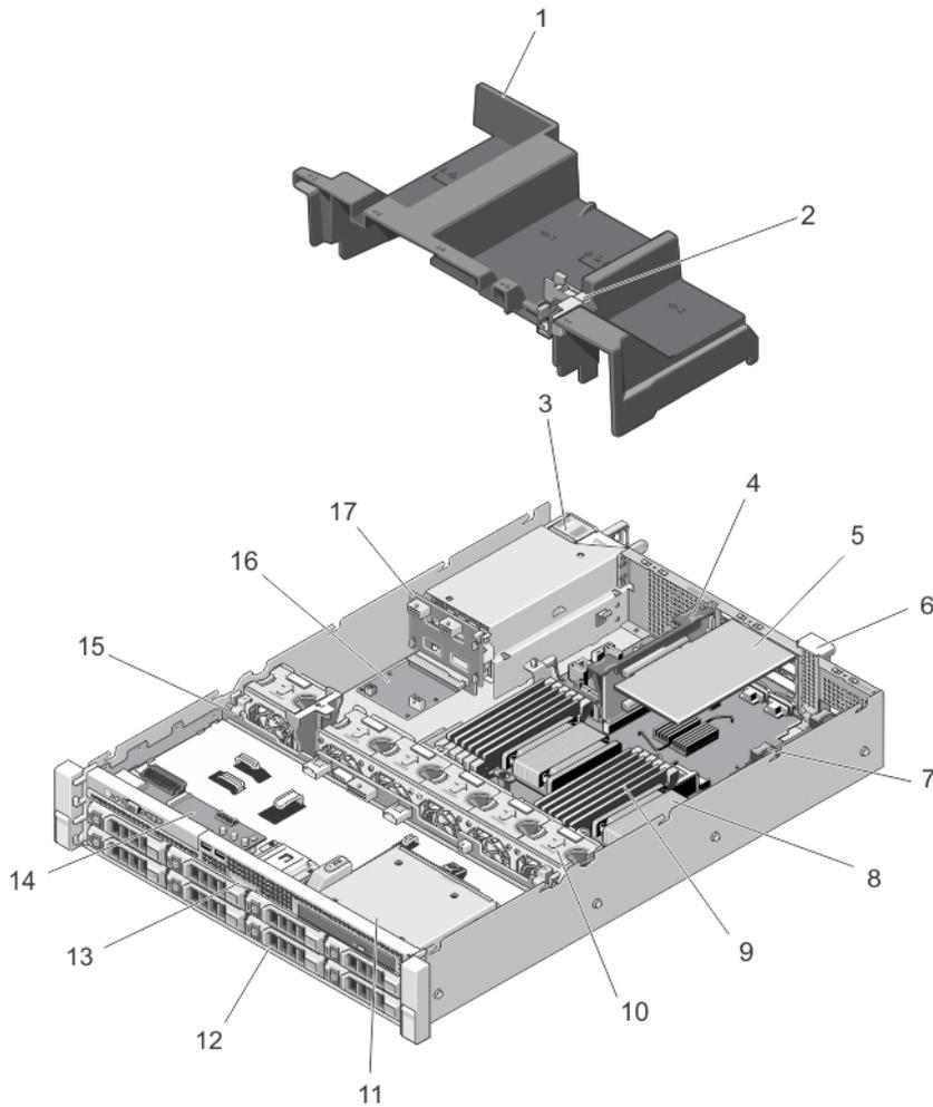
**Figure 13. Inside the System—Redundant Power Supply Unit Chassis**
