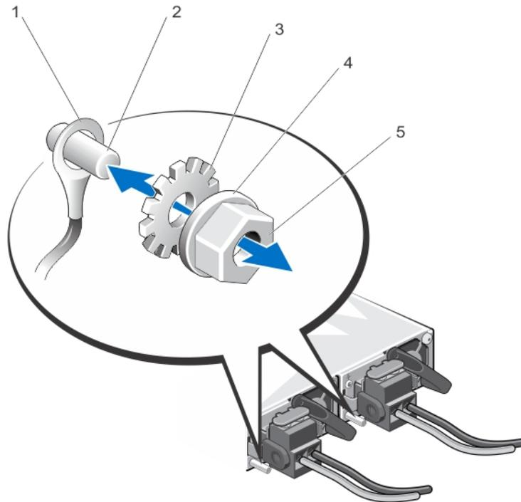
**Figure 41. Assembling and Connecting the Safety Ground Wire**
