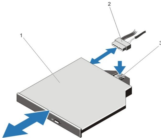
**Figure 27. Removing and Installing the Optical Drive**
