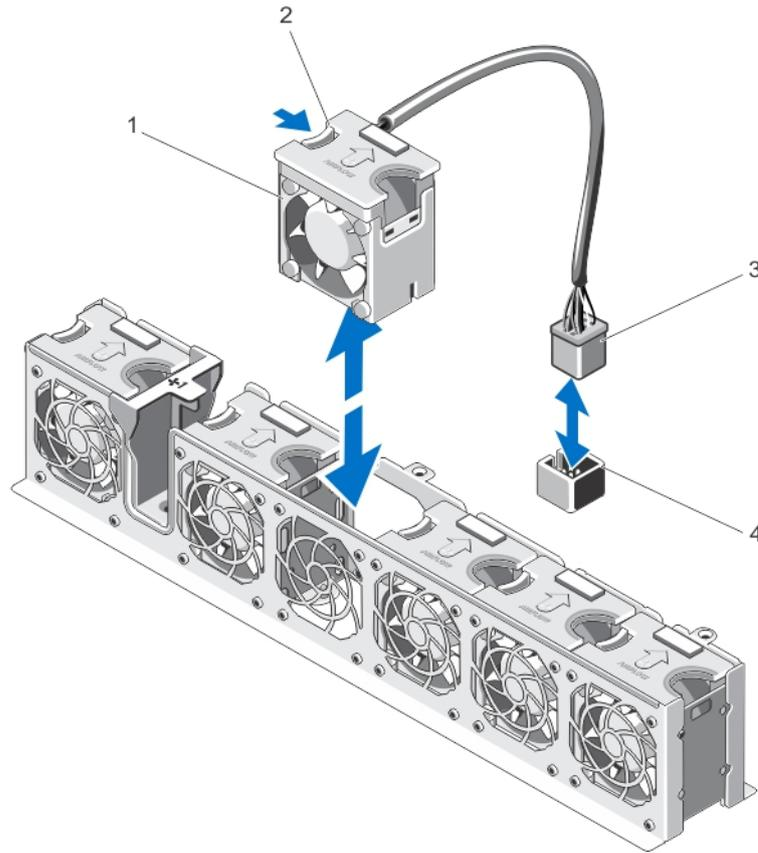
**Figure 28. Removing and Installing a Cooling Fan**
