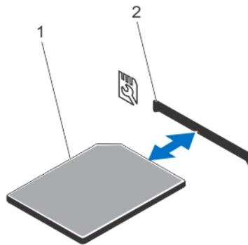
Figure 35. Removing and Installing the SD vFlash Card
