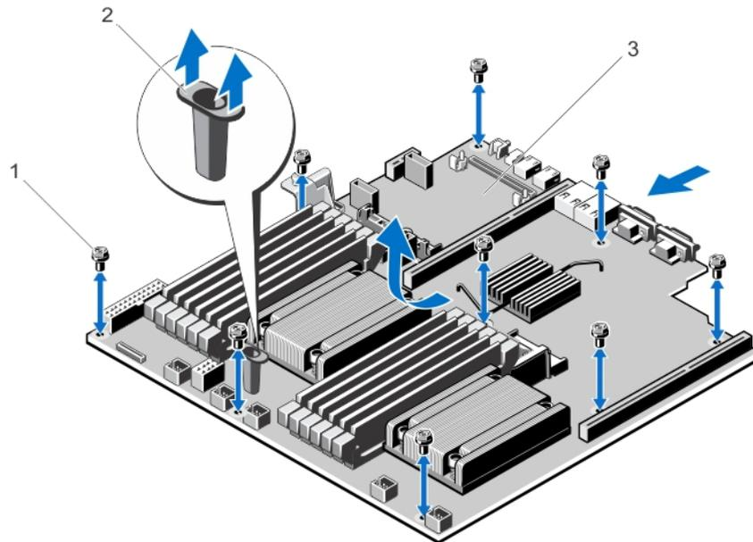
**Figure 55. Removing and Installing the System Board**
