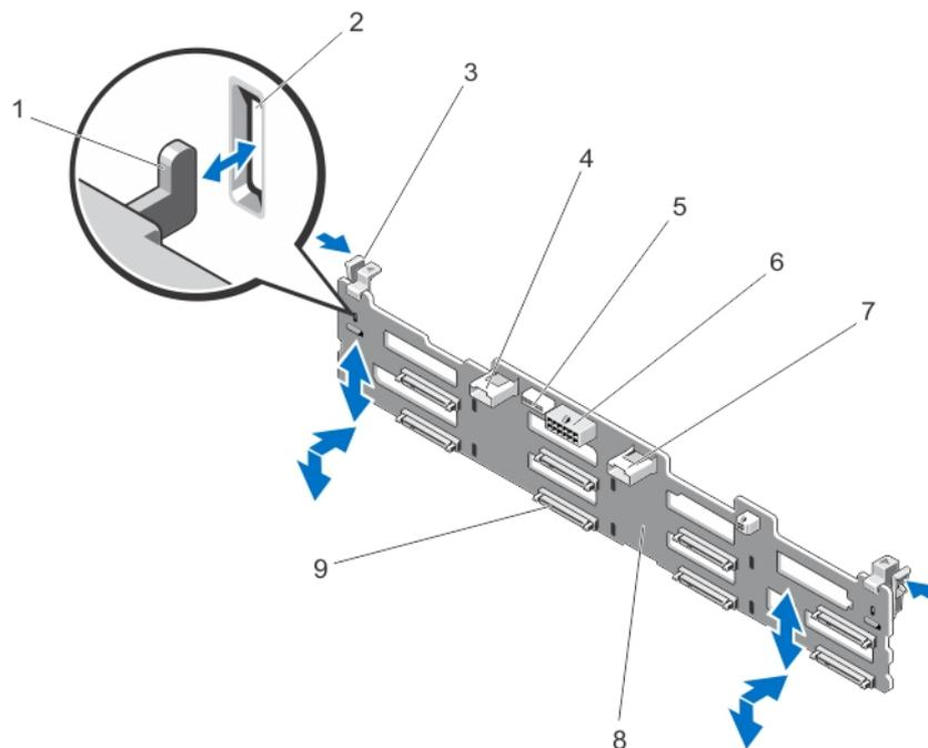
**Figure 51. Removing and Installing the Hard-Drive Backplane**
