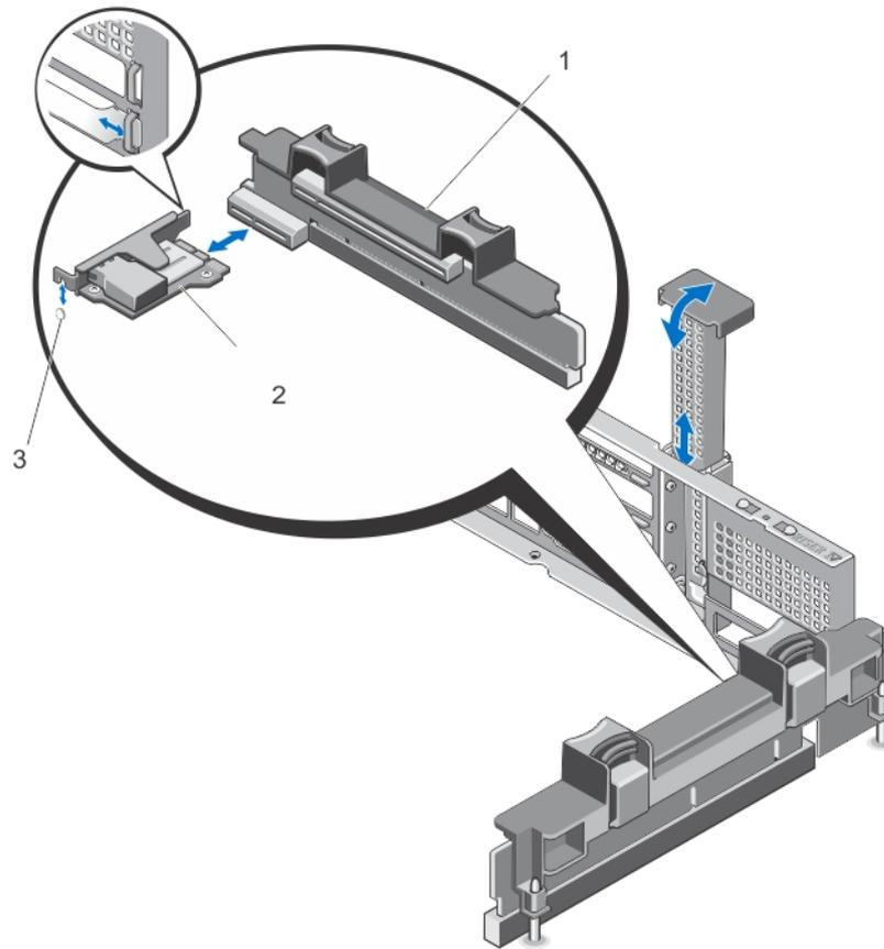
**Figure 34. Removing and Installing the iDRAC Ports Card**
