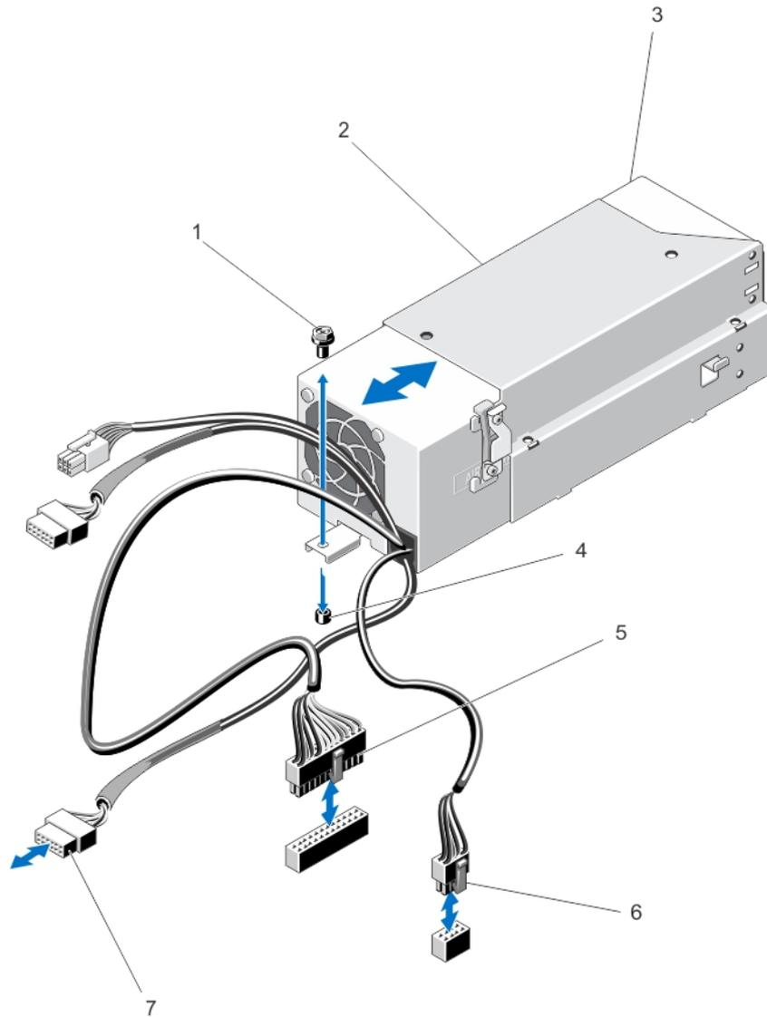
**Figure 48. Removing and Installing a Non-Redundant Power Supply**
