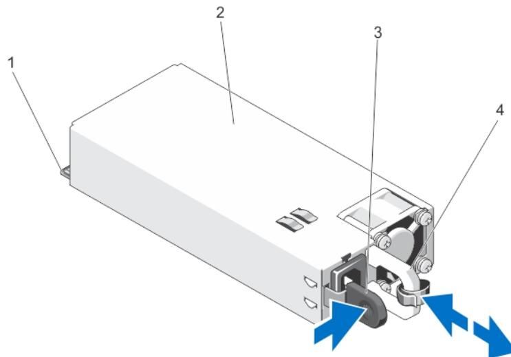
Figure 40. Removing and Installing an AC Power Supply
