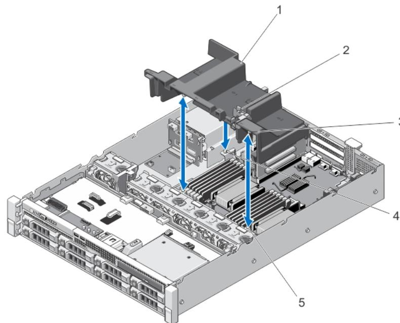
**Figure 15. Removing and Installing the Cooling Shroud**
