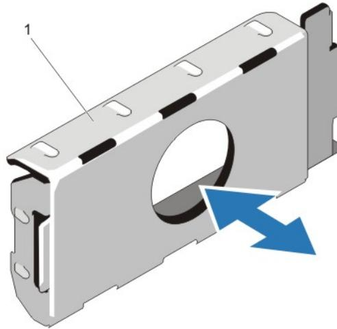
**Figure 44. Removing and Installing the Power Supply Blank**
