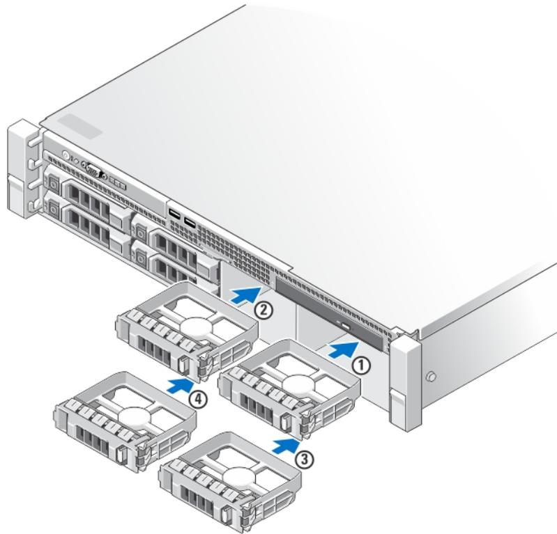
Figure 21. Hard-Drive Blank Installation Sequence
