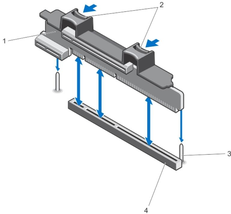
**Figure 32. Removing and Installing the Expansion-Card Riser 1**
