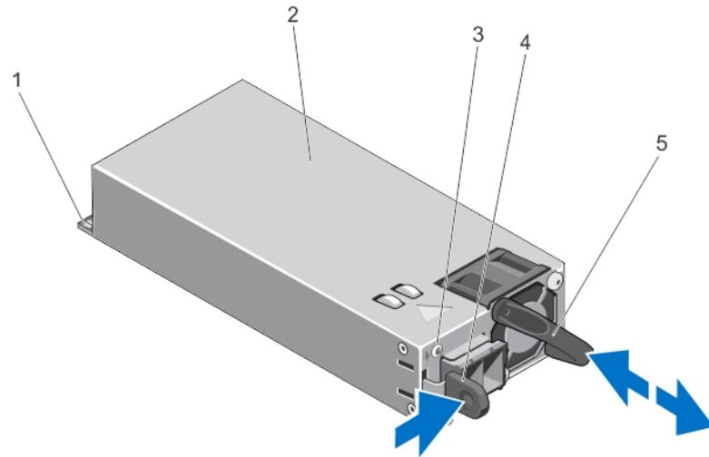
**Figure 43. Removing and Installing a DC Power Supply**
