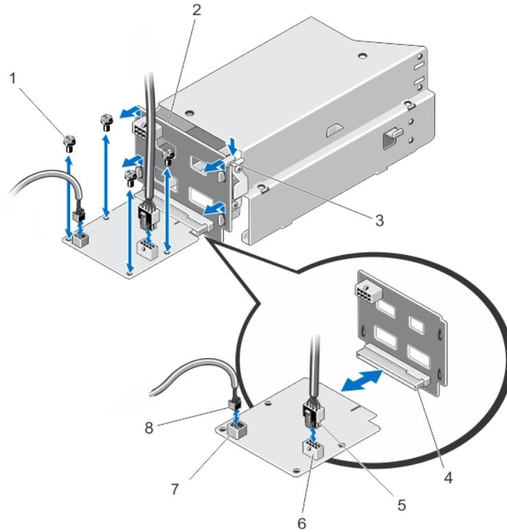
**Figure 45. Removing and Installing the Power-Distribution Board**
