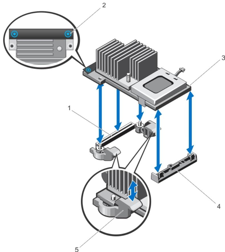
**Figure 37. Removing and Installing the Integrated Storage Controller**
