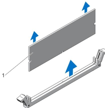
**Figure 18. Removing The Memory Module**
