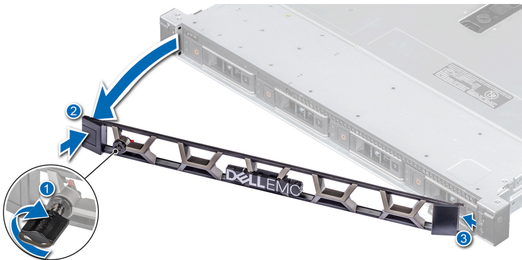
Figure 9. Removing the front bezel
