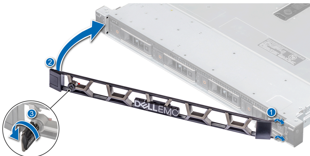
Figure 10. Installing the front bezel
