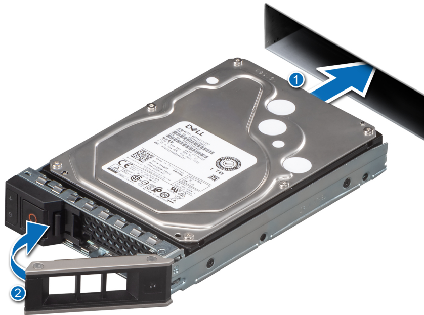
Figure 22. Installing the hot-swappable drive
