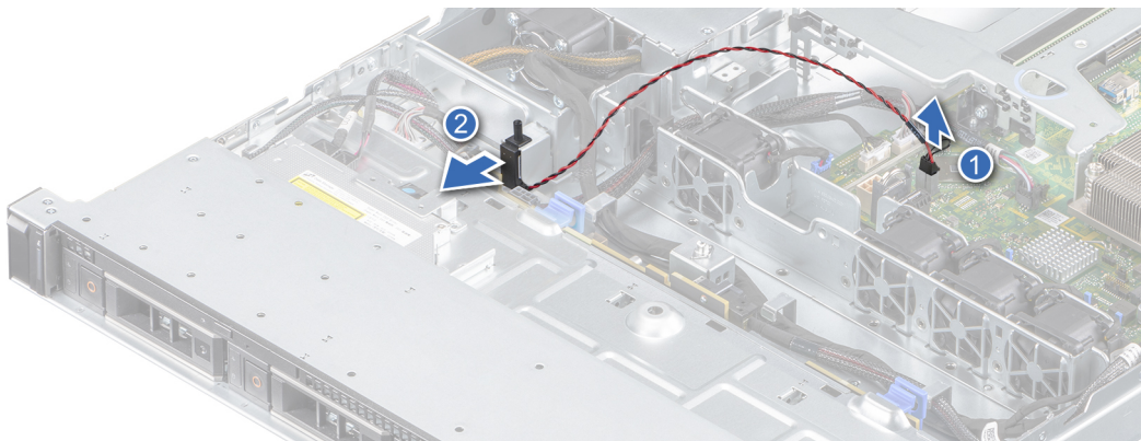
Figure 33. Removing the intrusion switch
