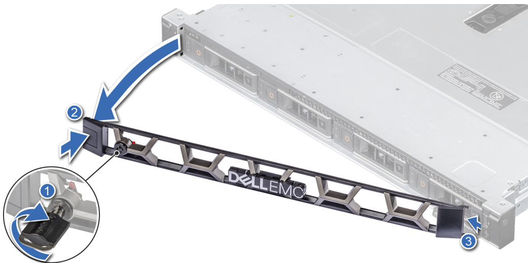
Figure 9. Removing the front bezel
