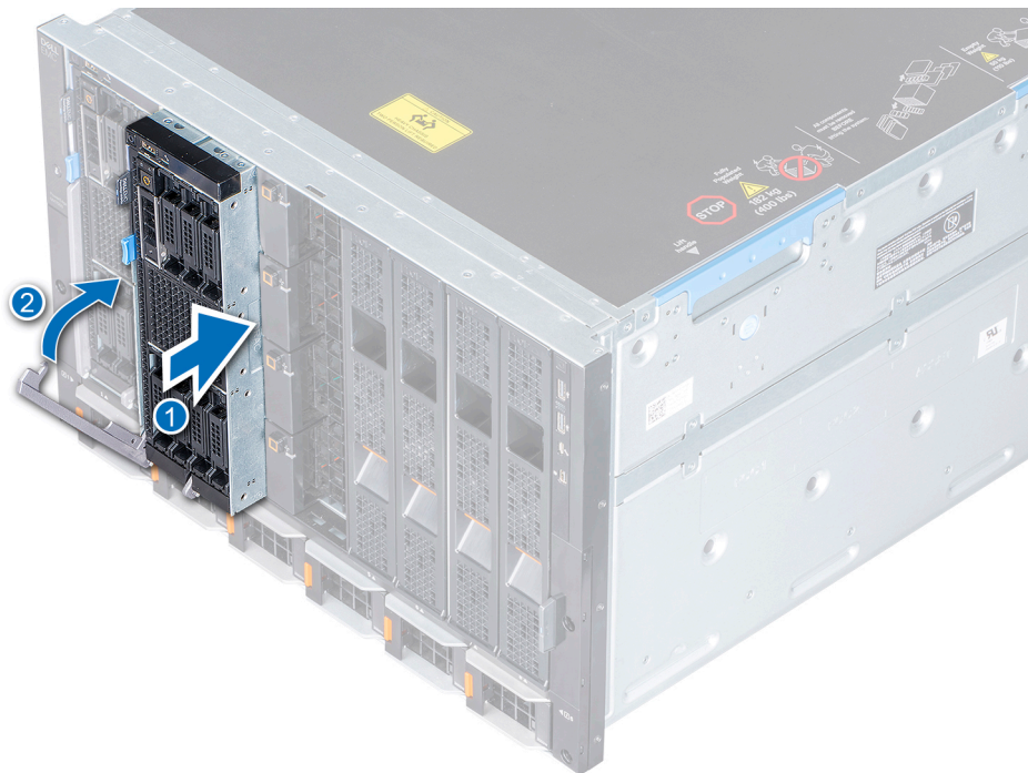
Figure 16. Installing the sled into the enclosure
