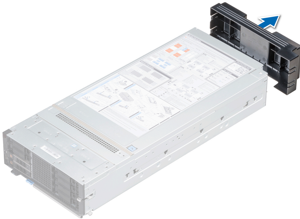
Figure 15. Removing the I/O connector cover from the sled
