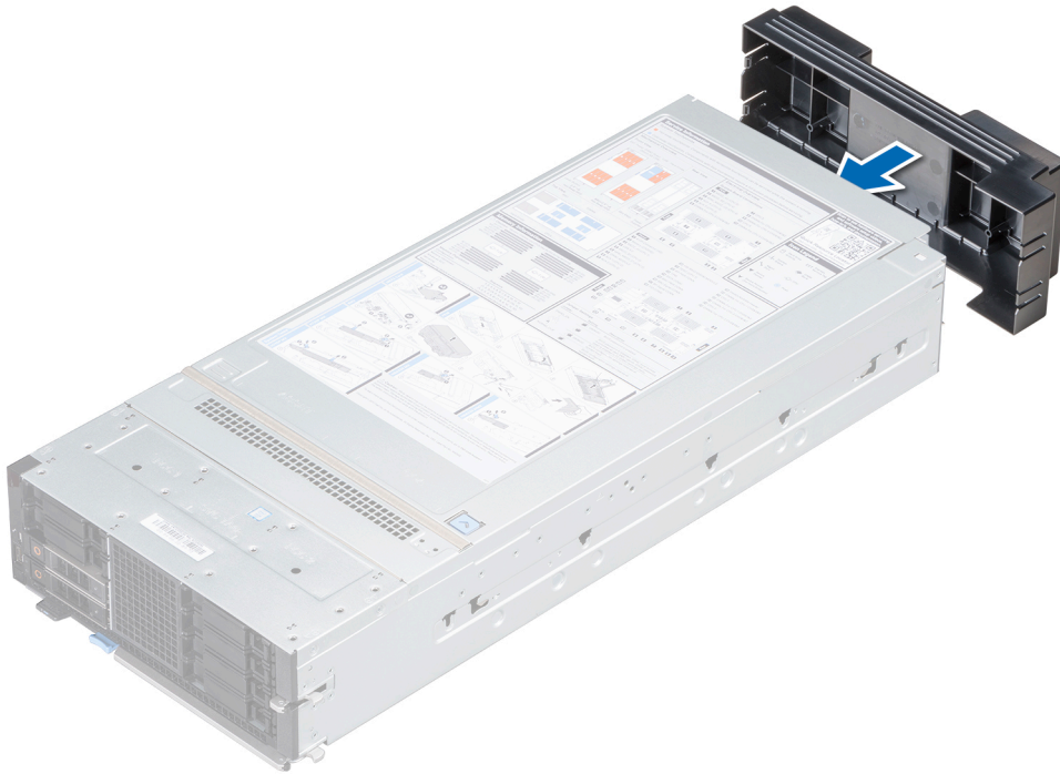
Figure 14. Installing the I/O connector cover on the sled
