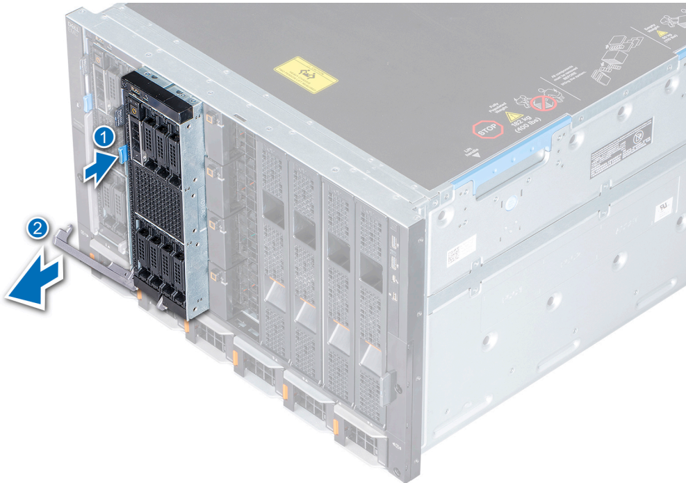
Figure 13. Removing the sled from the enclosure
