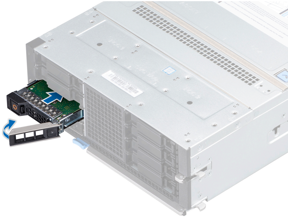
Figure 28. Installing a drive carrier
