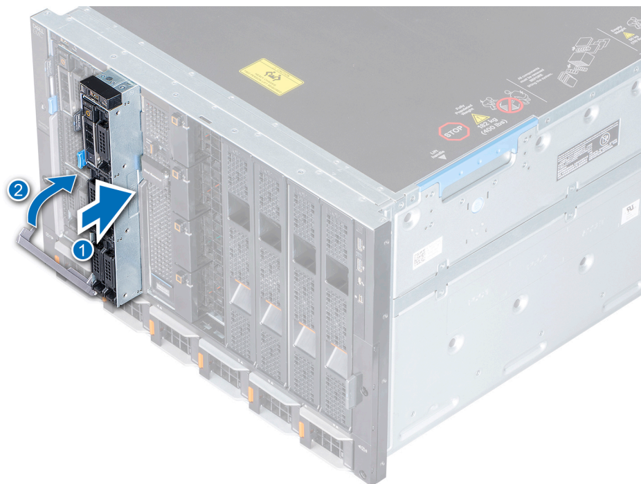
Figure 15. Installing the sled into enclosure
