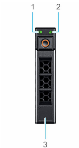
Figure 14. Drive indicators on the drive and the mid drive tray backplane
