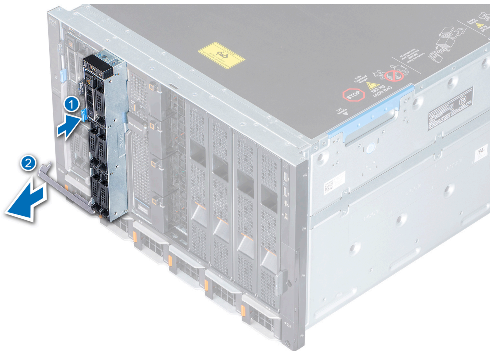
Figure 16. Removing a single-width compute sled from the enclosure
