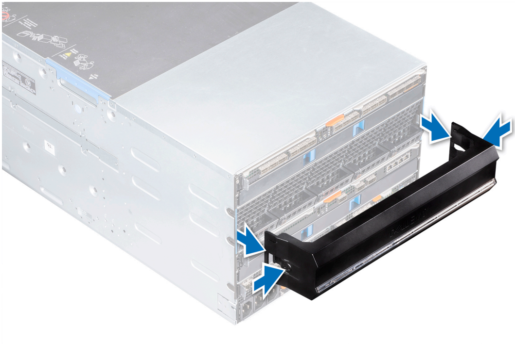
Figure 26. Removing the air baffle
