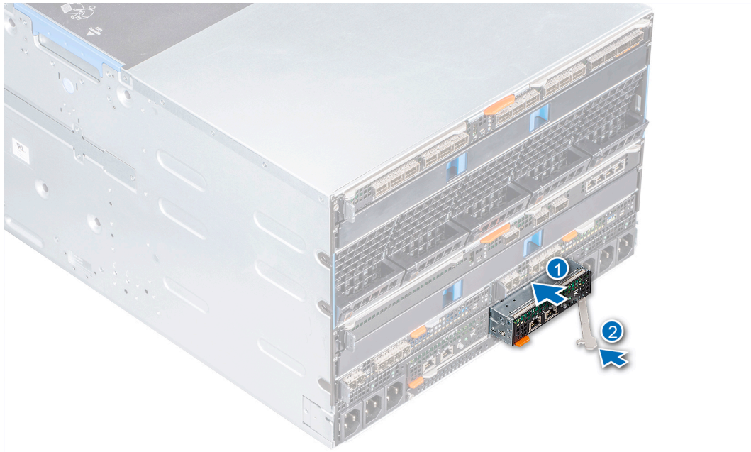
Figure 40. Installing a management module
