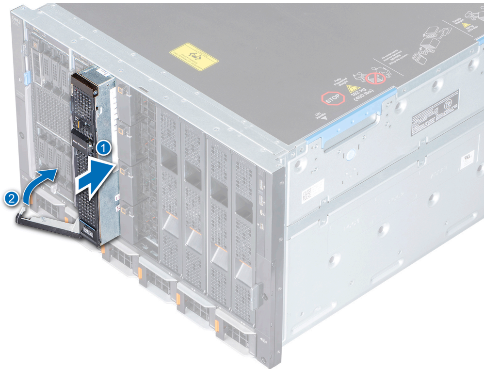
Figure 19. Installing a storage sled into the enclosure
