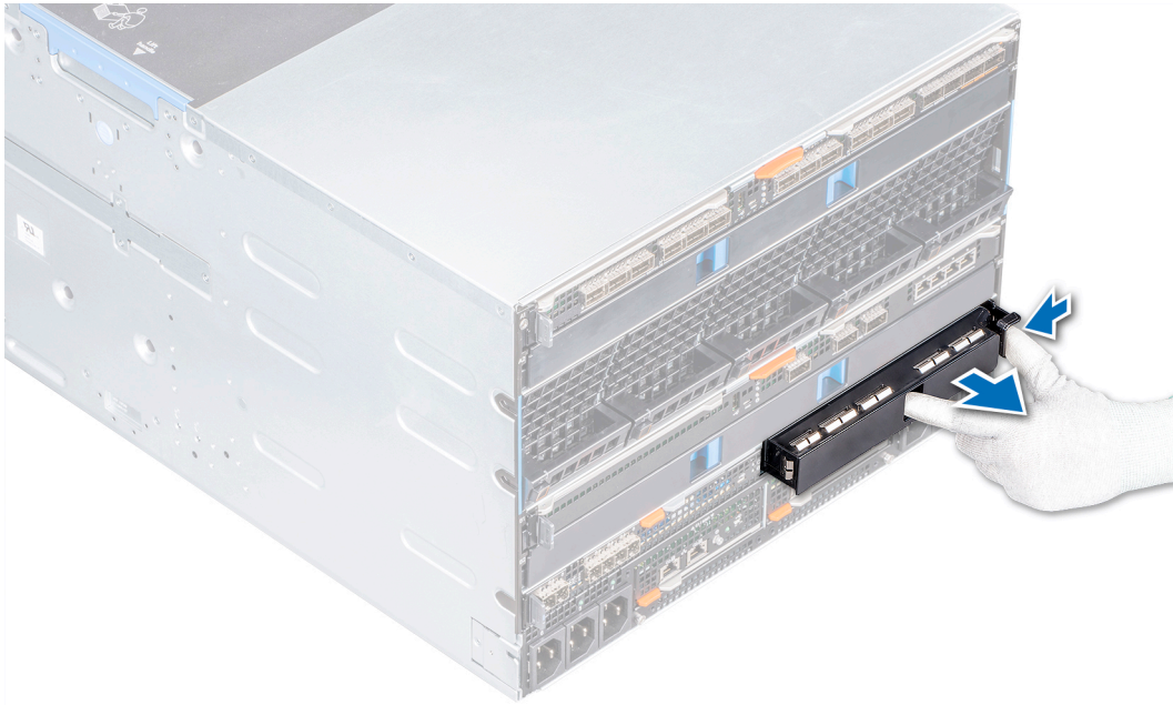
Figure 32. Removing a blank from Fabric C slot
