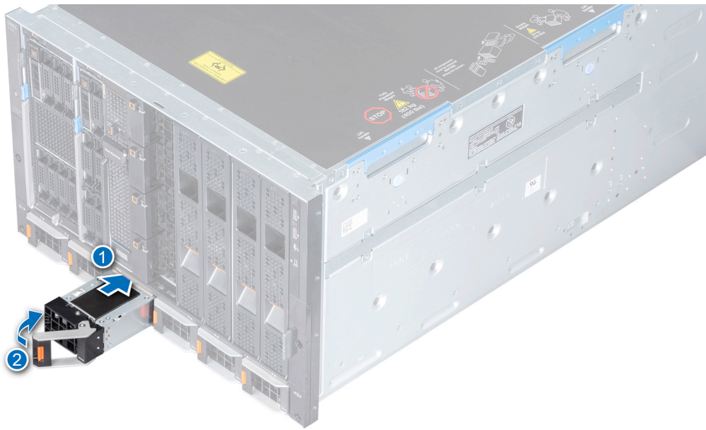
Figure 25. Installing a power supply unit
