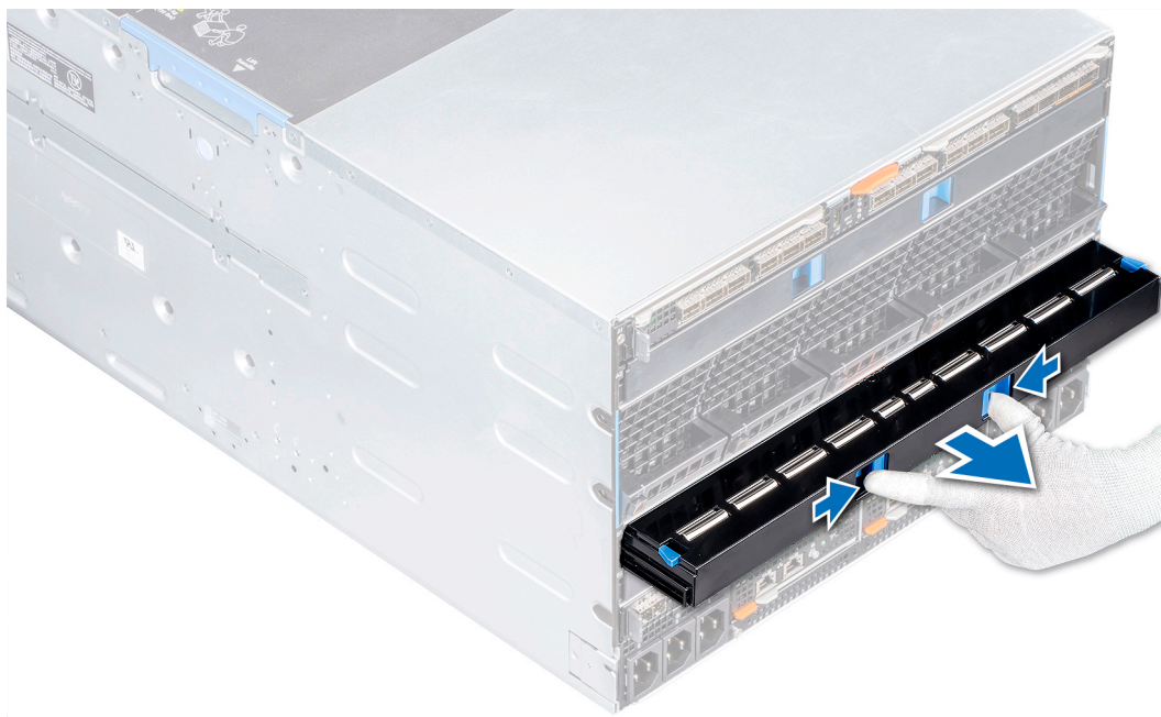
Figure 28. Removing a blank from Fabric A or B slot
