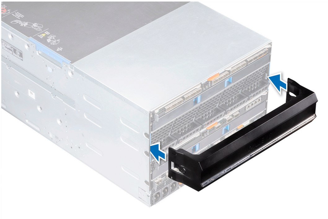
Figure 27. Installing the air baffle
