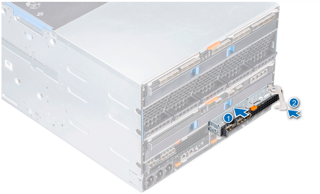
Figure 25. Installing a MX5016s module into Fabric C slot
