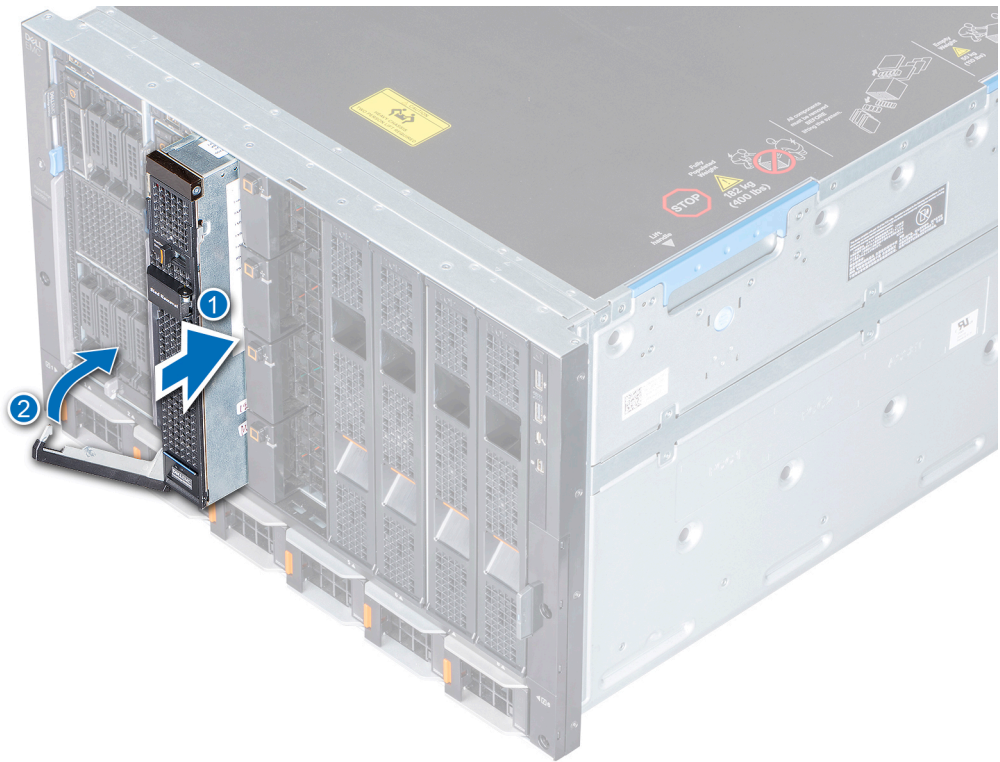
Figure 9. Installing the sled into the enclosure
