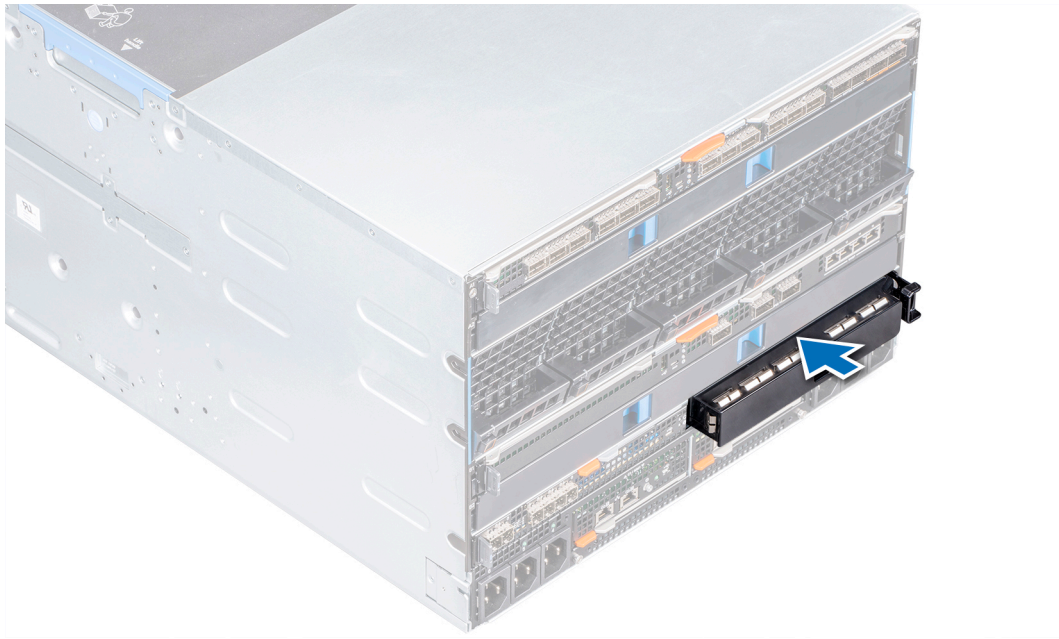
Figure 23. Installing a blank in Fabric C slot
