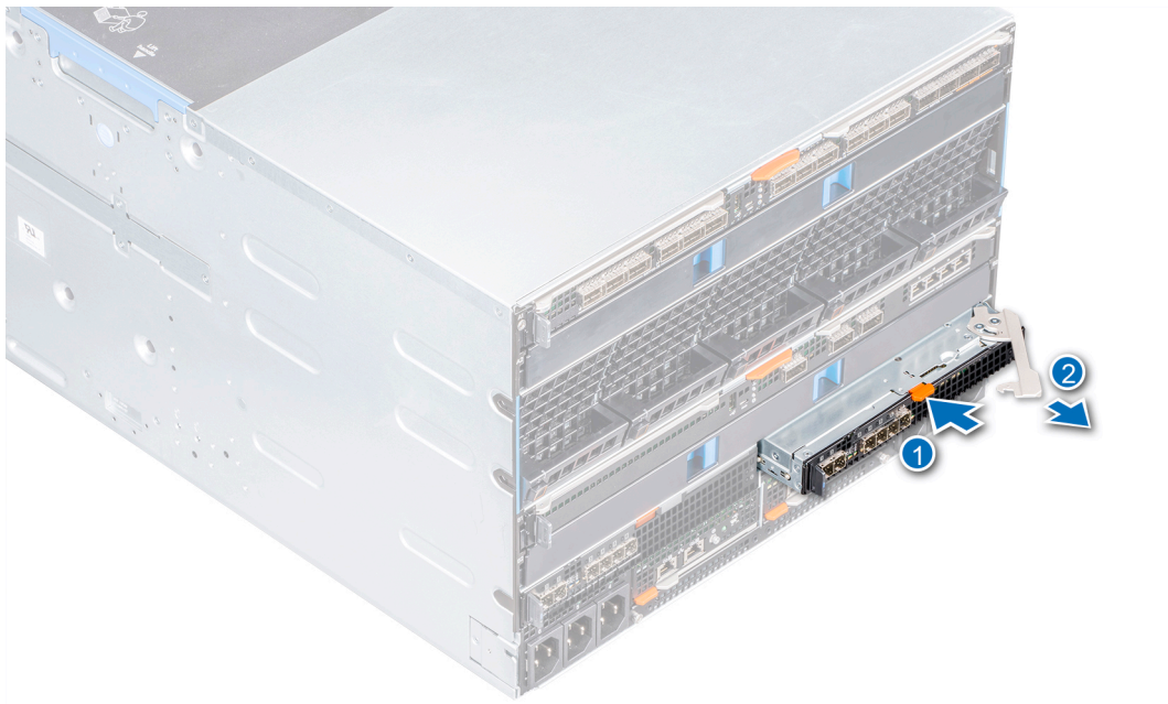
Figure 24. Removing a MX5016s module from Fabric C slot
